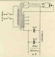
Fig. 12.- A circuit of a simple eliminator with resistance smoothing for the high-tension supply.
