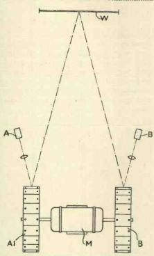
A method of employing two light sources for projection on to one screen in order to increase the lighting intensity. Patent No. 408596.
