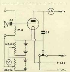
Circuit of the simple slide-back value voltmeter described in the text. Owing to its extreme flexibility it should find many uses in the experimenters' laboratory.
