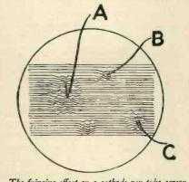
The fringing effect on a cathode-ray tube screen. Patent No. 408297.
