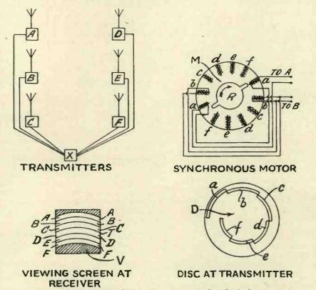
Four diagrams showing the principle of the Marconi apparatus for indicating bearings at sea in visible form. The purpose is to obviate the necessity of any special knowledge on the part of the navigator. Patent No. 408015.
