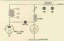
Fig. 4.—The connections for an A.C. mains receiver which are applicable to most commercial receivers.
