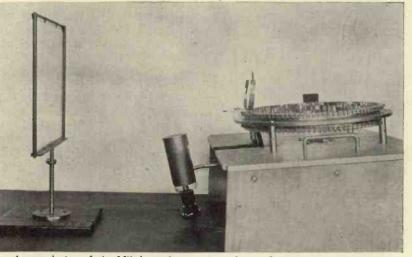
A general view of the Mihaly stationary mirror drum. In the receiver with which the demonstration was given an ordinary projection lamp was used, the light being modulated in a Kerr cell.
