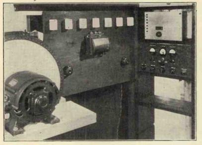
A simple 90-hole disc receiver is used as a check for the output of the transmissions.
