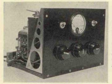
A view of the completed supply unit for the cathode-ray tube.
