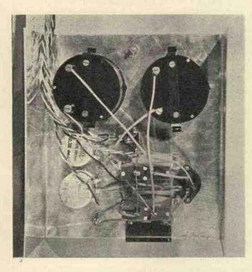
This photograph shows the underside of the chassis; the wiring of the instrument is very simple and will be clear from a study of this picture and the circuit diagram.
