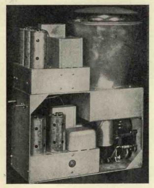
[Photo: Journal of the Franklin Institute An internal view of the Zworykin receiver showing the Iconoscope.
