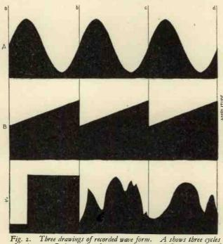
Fig. 2. Three drawings of recorded wave form. A shows three cycles of a sine wave, B three cycles of a saw tooth wave, and C a square topped and two irregular wave forms.
