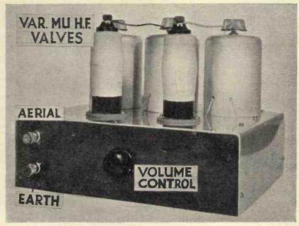
Only the values and coils are on the upper part of the chassis : all the wiring is below.
