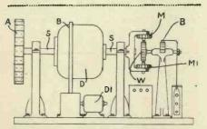
A method of synchronising employing a separate motor to revolve the carcase of the main driving motor. Patent No. 408332.
