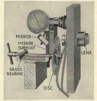
Fig. 4. A photograph of the actual chopper assembly. It will be seen that the mechanical construction is quite simple.
