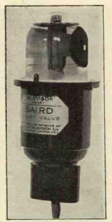
An example of an efficient grid cell-the Baird.
