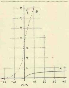
Fig. 3. --- Typical current | voltage curve for a deflector plate, the other three plates being strapped on to the gun. Deflector Plate Current at 50µ.A Gun Current. Curve A: Shielded Structure. Curve B : Similar structure without Shield.
