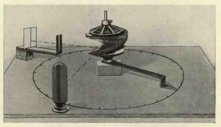
Fig. 2. Accuracy in the setting of the mirrors can best be obtained with a similar arrangement to that shown by the photograph : the long pointer and distance the light beam has to travel ensure that only very small errors can occur.
