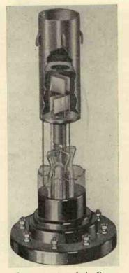
A cut-away view of the Cossor cathode-ray tube showing the arrangement of the electrodes.
