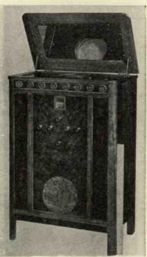
[Photo.: Journal of the Franklin Institute A finished model of a television receiver incorporating the Zworykin Iconoscope.
