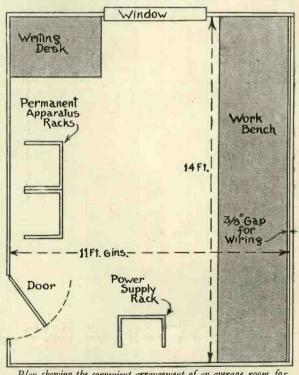
Plan showing the convenient arrangement of an average room for television experiment.
