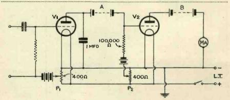
Fig. 4.- The circuit of the highly sensitive value voltmeter described.
