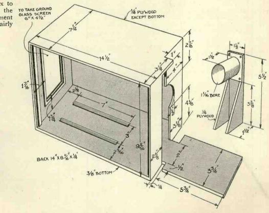
Details of main optical box with baseboard and (inset) projection lamp holder and stand.
