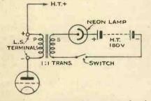
If you have two receivers and can spare one for television, this circuit can be recommended. Simply take off the loudspeaker and connect the neon lamp as indicated. The transformer primary connections should be reversed if the pictures are reversed.
