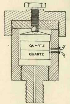
Fig. 5.—Crystal "pressure-gauge" for recording explosion pressures as used by Tokyo Institute.
