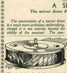
This sketch shows how the drum is assembled ready for filling with plaster.
