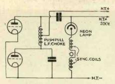
If you have push-pull output a tapped low-frequency choke can be used instead of a transformer. Notice how the synchronising coils are connected in series with the neon lamp and the H.T. side of the hightension baltery.
