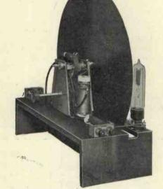
NEW COMPONENT. For controlling your motor speed at 750 r.p.m. on 50 cycles A.C. mains for transmitters and for materially holding the image steady on receiving sets, is an 8-pole, laminated phonic wheel 2 in. diam. interchangeable with 30 pole wheels on standard synchronising gear. PRICE 7/6.
