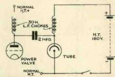
If you use a commercial receiver where the connec-tions are difficult to get at, this is the circuit to use. The output from the power valve is fed to the neon lamp through a large fixed condenser. An extra battery is required to bring the voltage up to over 180 volts.
