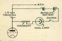
Better definition is obtained if the voltage applied to to the neon is varied by means of a resistance. The additional battery in this case should be large enough to cause the neon lamp to strike with the resistance only half in circuit.
