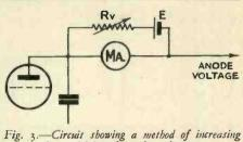
Fig. 3.—Circuit showing a method of increasing the sensitivity of a valve voltmeter.
