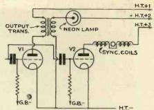
To obtain the maximum efficiency from synchronising coils you should make use of a special synchronising valve. With this circuit pictures can be held steady for quite long periods and will greatly increase the entertainment value of the television gear,
