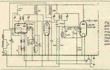
Fig. 1.—This is a good circuit that uses a double diode triode valve for rectification, lowfrequency amplification, and provides automatic volume control.
