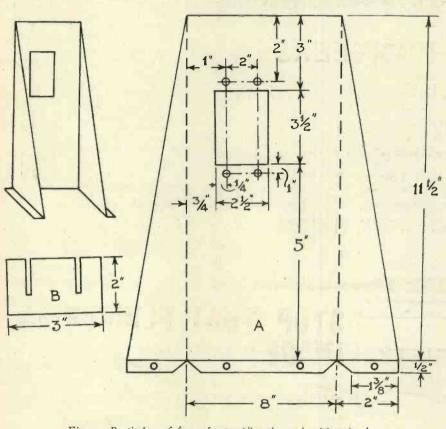
Fig. 2. Particulars of frame for providing the synchronising signal.
