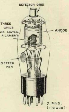
Fig. 2.—You can see from this sketch just how a battery heptode is constructed. It has a seven-pin base, but don't forget that the grid connection to the detector section is at the top of the bulb.
