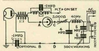
Over 300 volts can be obtained from this power pack so the output is enough to feed both the neon and the output valve. The usual variable resistance is included to improve the definition from the neon lamp.
