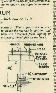
The drum is built up of a metal disc and brass tube. The method of fixing the mirrors is clearly shown.
