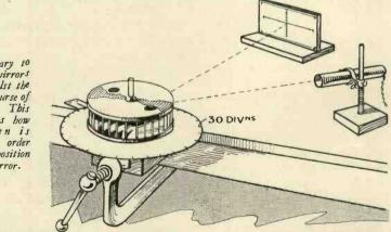
The lid with the boss fitted is then locked on a suitable length of spindle, which is arranged so that it will turn stiffly in a block of wood secured to a table. The sketch will make this mark upwards. When fifteen mirrors have been adjusted the centre line is reverted to and the remaining mirrors set by turning the drum in the opposite direction.
