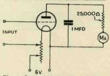
Fig. 2.—Circuit of Moullin type valve voltmeter
