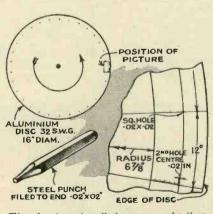
These drawings give all the necessary details to enable an amateur to construct a scanning disc.
