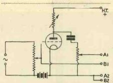
Fig. 4.—Connections for observing value curves under working conditions.
