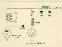
This is a circuit that can be used with the mains receiver. If the applied voltage is too high, the definition will suffer. This can be overcome by the use of the variable resistance.
