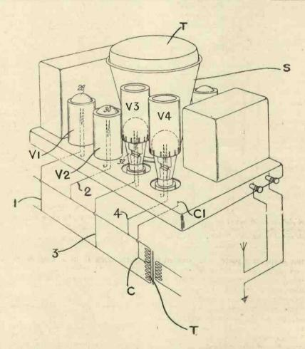
A wireless receiver with means for energising the valve filaments in groups with alternating current energy of opposite phase. Patent No. 412,435.
