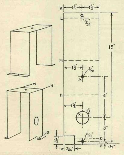
Fig. 1. Details of shield for enclosing the lamp.
