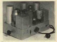
Tekade ultra-short wave chassis using a five valve circuit, octode 3 I.F. triodes and double diode triode detector.
