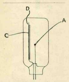
A glow lamp with part of the cathode coated with a substance baving a lower extinction potential than the rest of the cathode. Patent No. 412,024.
