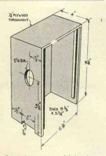
Details of the construction of the lamp box.
