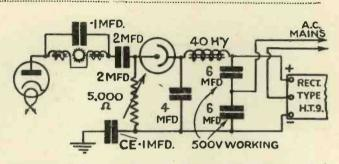
This is a simple arrangement in that there is no transformer and the potentiometer is across the supply instead of in series with the neon lamp. With the synchronising coils in series with the anode of the output value the pictures are kept very steady.
