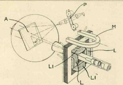
" keystone " Arrangement of cathode-ray tube with means of eliminating distortion. Patent No. 412,092.
