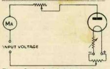
Fig. 1.-Circuit of simple diode valve voltmeter.
