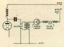
If you have over 200 volts available and can get at the anode circuit of the power value, the neon can be modulated through a 1:1 transformer. The neon lamp is in series with the synchronising coils and the high-tension.
