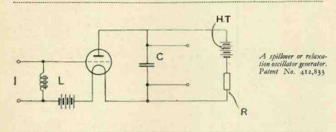
by a frequency applied to the input terminals I may be derived from a terminals I. The latter are shunted by an iron-cored choke L, which is saturated for the greater part of each cycle of the input frequency. A funken Co.)
