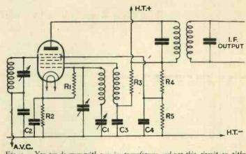
Fig. 4.-You can do away with a mains transformer and use this circuit on either A.C. or D.C. mains, providing you have an Ostar-Ganz high voltage pentagrid.
