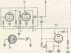
Method of preventing picture signals affecting synchronisation. Patent No. 457,879
