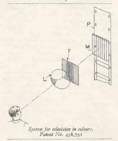
film is placed a lenticular grating M, which consists of a row of cylindrical lenses placed side by side.
