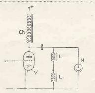
Preserving correct form of saw-tooth waveform in magnetic scanning. Patent No. 457,929
