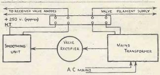
Schematic drawing showing method of supplying low- and high-tension current for the sound and vision receivers.
