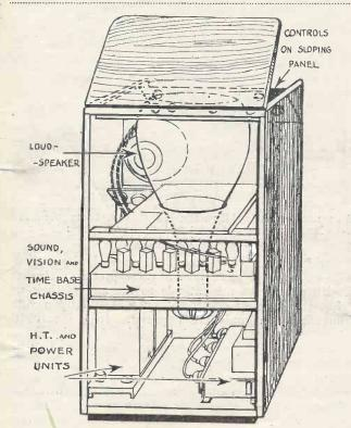
A typical arrangement of the units of a television receiver in which the picture is viewed in a mirror placed at an angle of 45 degrees. The cathode-ray tube, it will be seen, is vertical.
