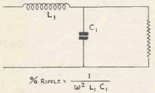
Fig. 1. Calculating ripple value.
