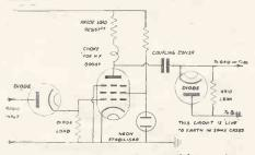
Fig. 3. A complete video amplifying stage showing the D.C. restoring diode and components referred to in this article.
