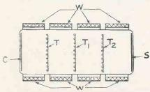
Electron-multiplier with permeable screen. Patent No. 504,927.
