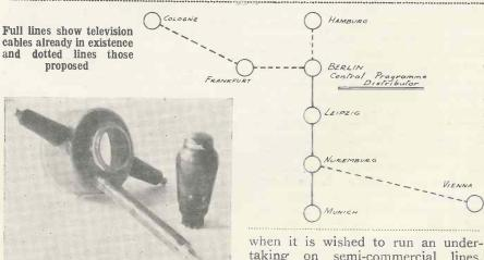
These are two of the small projector tubes used for the Fernseh home projector. An ordinary valve gives an idea of the size.
