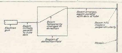
overall sensitivity 10 to 20 times that Fig. 1. In order to maintain perpendicular scanning a combination of electronic and magnetic forces is employed, the field deflecting the beam temporarily.
