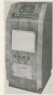
A console type receiver by Marconiphone is the model 713. In addition to providing television sound and vision a 6-valve 3 waveband, pressbutton radio receiver is incorporated.
