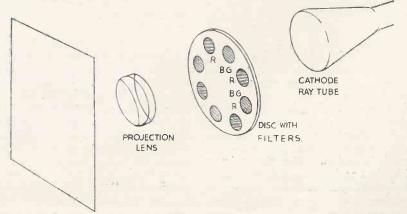
Fig. 2. Schematic outline of Baird colour television receiver.
