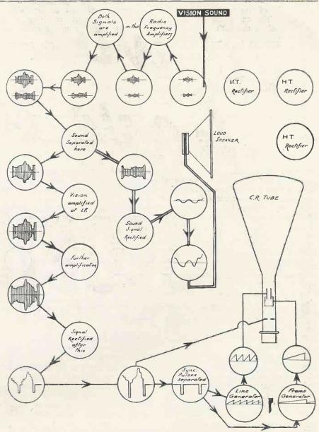
Valve line-up of G.E.C. model BT9121 receiver.
