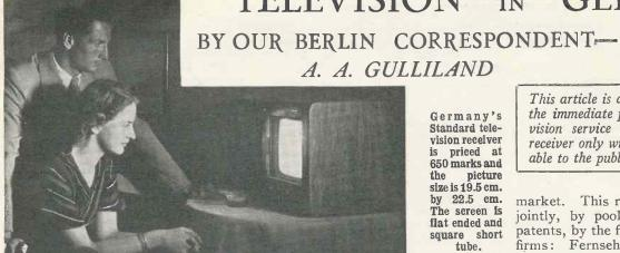
Germany's Standard television receiver is priced at 650 marks and the picture size is 19.5 cm. by 22.5 cm. The screen is flat ended and square short tube.
