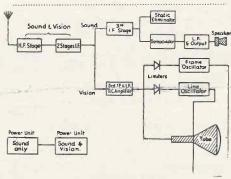
Schematic diagram of H.M.V. receivers.
