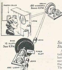
Fig. 1. The Baird colour television transmitter.
