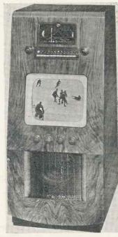
A console type receiver is the H.M.V. 1850. The picture size is  $11\frac{6}{3}$  in. by  $9\frac{2}{3}$  in., and in addition, an all-wave push-button radio is provided.
