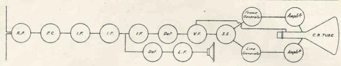
Valve line-up of H.M.V. model 907.
