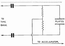
Fig. 5.—Symmetrical circuit for balancing potentials applied to the deflector plates to overcome distortion.
