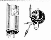
On the left is the first impedance matching transformer connected close to the aerial at the top of the mast. The second transformer is fitted to the receiver chassis.
