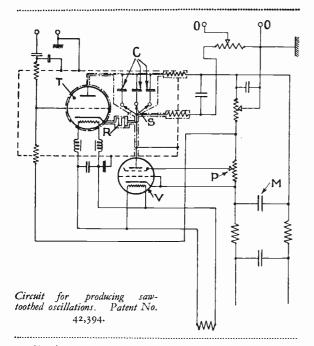
oscillations generated across both values in series are applied to the deflecting electrodes of the cathode-ray tube to produce the two scanning lines shown in Fig. 2. It will be seen that the lower ends of the curve B rise in steps, as compared with the curve A, by an amount represented by the wedge-shaped curve O.—(J. L. Baird and Baird Television, Ltd.)
