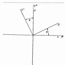
Fig. 3.—OX = fast direction of first quarter-wave plate;  $OX^1 = fast$  direction of birefringent section;  $OX^{11} = fast$  direction of analysing quarter-wave plate.
