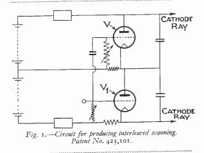
" interleaved " scanning. In this system two separate spots are made to alternate with each other in such a way that when one spot has finished the first line it is returned to a position where it repeats the first line scanned by the second spot, and so
