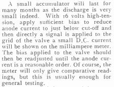
So as to extend the scope of the meter a variable potentiometer has been connected across the bias battery, for the amount of applied bias can be increased to make the unit less sensitive.
