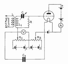
This is the circuit for the suggested meter. It is better to use this than to rely on the fact that 23 per cent. rise should mean 100 per cent. modulation.
