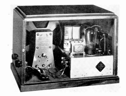
Most of the wiring is point to point. This is most essential on the higher frequencies. Keep the connectin wires short.
