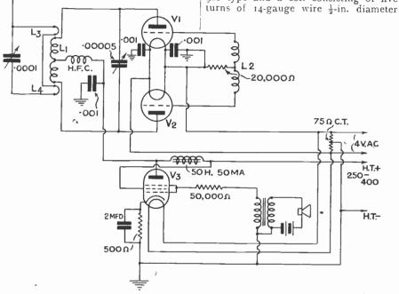
This modulated five-metre transmitter is very stable in operation. The 200 miles record set up last year used a fundamentally similar circuit.
