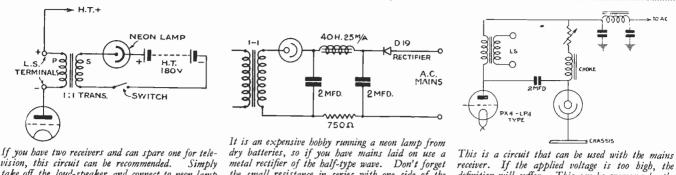
vision, this circuit can be recommended. Simply take off the loud-speaker and connect to neon lamp as indicated.
