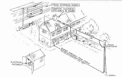
Where the interference is local it is advisable to bury the lead in wires as much as possible. This is particularly advisable when the interference is from car ignition or small motors.
