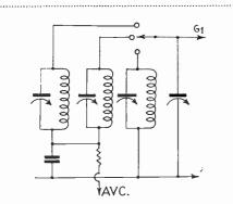
Fig. 2.—It is suggested that on the 25-megacycle band automatic-volume control be omitted. Notice that the third coil is then connected to earth.
