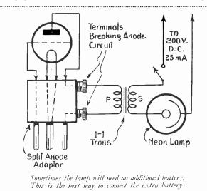
over 200. This is perhaps the most convenient way of connecting the neon lamp, and one that will overcome
