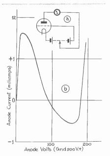
Fig.1.—(a) Circuit to show secondary emission. (b) Anode current curve for triode with coated anode.
