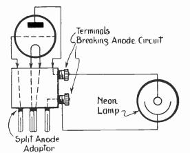
With a commercial receiver a split anode adaptor will come in useful. The lamp can be connected to the two side terminals on the adaptor.
