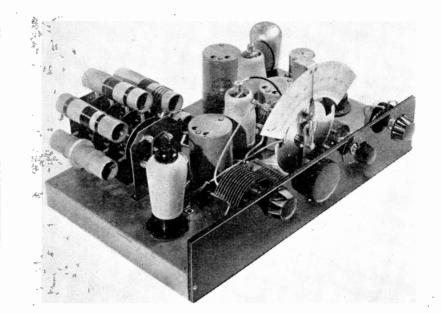
Here is the receiver chassis. The panel is only a temporary one used to secure the tuning components during testing.
