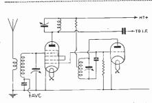
Fig. 3.-For ultra short-wave and or television reception a separate oscillator is recommended in this circuit.
