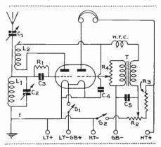
while the values should be .00025-mfd. for C2, .0001-mfd. for C1, .0003-mfd. for C3; R2 is 25,000 ohms, with a class B valve, such as the Cossor B240. The remaining components are of standard values and are not critical.
