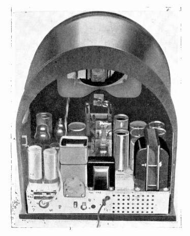
ceiver although it uses eleven valves is no larger than uroad-ust super-bet. Ganged the average broad-Ganged tuning, single dial control and A.V.C. on all wavelengths are only three of the many features of this receiver. Five tuning scales, all calibrated in frequencies, is a fine idea for it overcomes the diffi-culty of designing a clear tuning scale.
