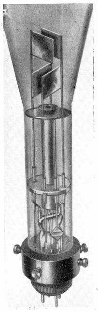
Fig. 1.—Photograph of the elsctrode assembly of the cathode-ray tube.
