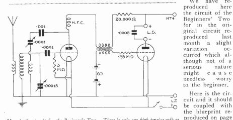
Here is the circuit for the Beginner's Two. There is only one high-tension voltage tapping; it is impossible to slort-circuit high-tension to the reaction condenser owing to the use of a series blocking condenser.
