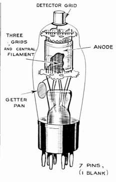
Fig. 5.—All the electrodes in this Osram beptode can be quite clearly seen. A point to remember is that the control grid is taken to the top cap.
