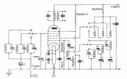
Fig. 1.—This is the heart of an efficient short-wave super-het. It can be added to almost any short-wave super but preferably one with 450 ks. I.F. transformers.
