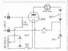
The circuit arrangement is actually an anode bend detector using a low-impedance triode valve.
