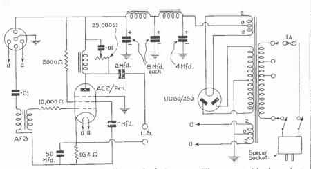
This section of the circuit is entirely self-contained. It gives 3,400 milliwatts output with only a moderate input. The power pack gives' 250 volts H.T. at 60 milliamperes.
