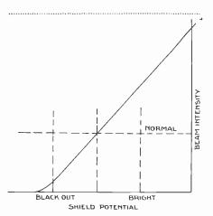
Fig. 1.—Ideal curve of beam Tintensity—shield potential giving full modulation with no distortion.
