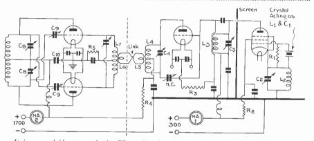
It is a sound idea to couple the CO to the sub-amplifier by means of a transformer. This does overcome the possibility of a faulty high-frequency choke.
