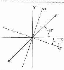
2.—The circular polariser and analyser. 1 is the nicol with quarter-wave plate OX;  $OX_1$ is the analysing quarter-wave plate.
