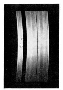
Fig. 1.—Illustrating the effect of an exposure of one-fifteenth sec. Note the vertical bands due to mains modulation on the lamp and indicating asynchronism. The thin vertical black line is a faulty bole in the disc.
