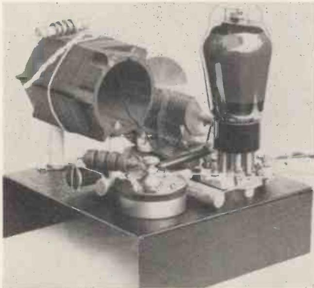
*The split stator condenser shown is used as a single unit condenser, but it can be used as a split stator and then the anode coil must be centre tapped, but the anode by-pass condenser can be omitted.*
