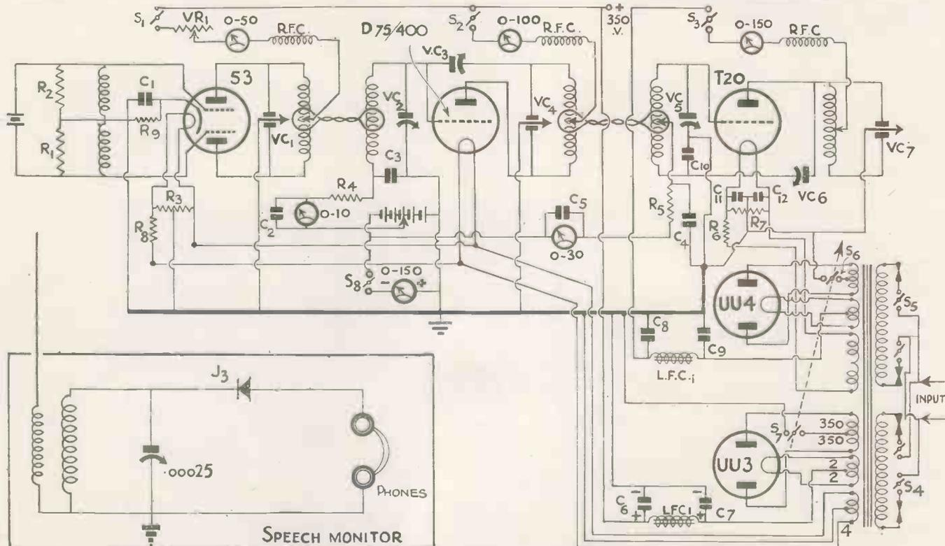
This three-stage transmitter is quite straightforward, although maximum efficiency is obtained. Notice the grid neutralising allowing for maximum impedance in the P.A. stage, and also the built-in speech monitor.
