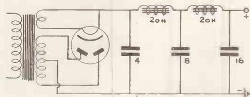
scanning speed and the additional condenser cured this. The total consumption of the scanning circuit is approximately 16 mA, and it would be preferable to tap the H.T. for the video amplifier from the first choke to provide higher voltage and a degree of decoupling.
