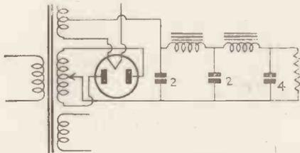
Fig. 1.—This is the most widely used power supply circuit with an untuned filter.
