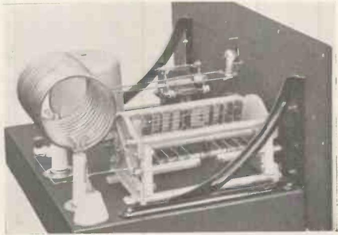
*By mounting the coil near the end of the P.A. condenser, the leads are kept short, while there is only a comparatively simple lead to the anode of the T20 valve.*
