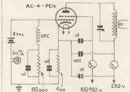
*Fig. 1.—The circuit is quite conventional, but in case of accidents, do not omit to include the fuse-bulb.*
