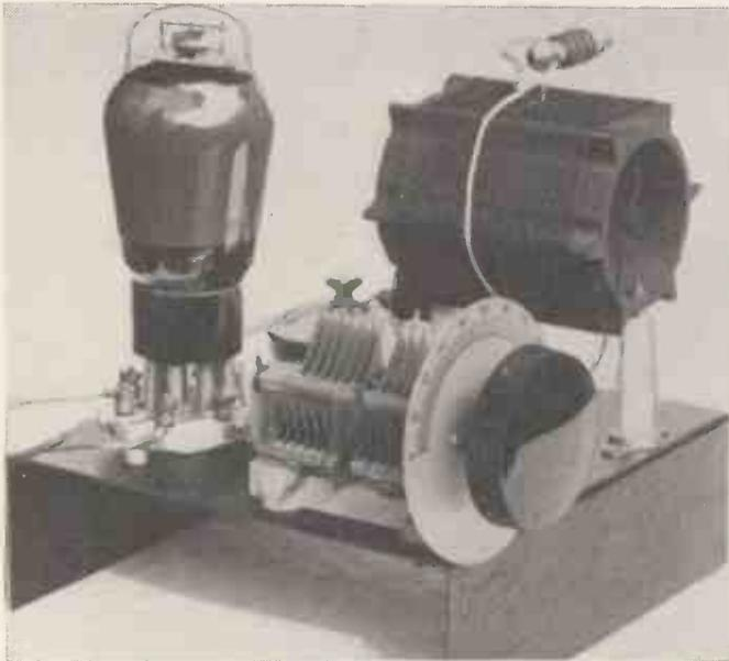
*This is the original experimental chassis on which we tested the AC4/PEN. It is not essential to use such a large diameter coil, but it has one advantage, a tapping point can be made during the experimental stages.*
