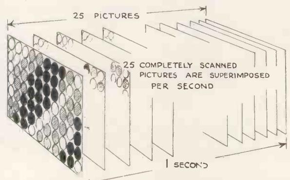
This diagram conveys the idea of how successive pictures can be thrown upon the screen and owing to the persistence of vision effect give an idea of continuity of motion.
