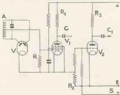
*Separating synchronising and picture signals. Patent No. 466,419.*
