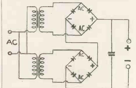
Fig. 8.—Either vacuum valves or metal rectifiers can be used in a bridge circuit. In this instance metal rectifiers connected in series give a high output but require two HT transformers.
