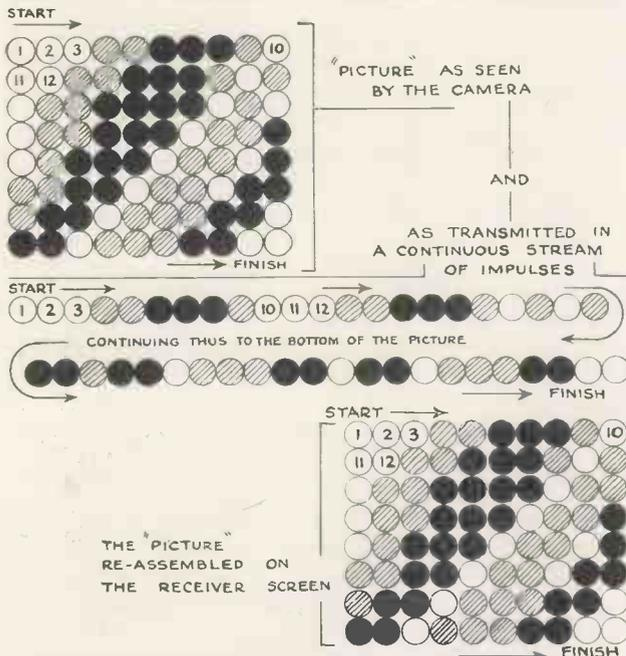
Here is an imaginary analysis of a picture with the units greatly enlarged. The diagram shows how the image can be broken up and transmitted in proper sequence and finally re-assembled to form the original.
