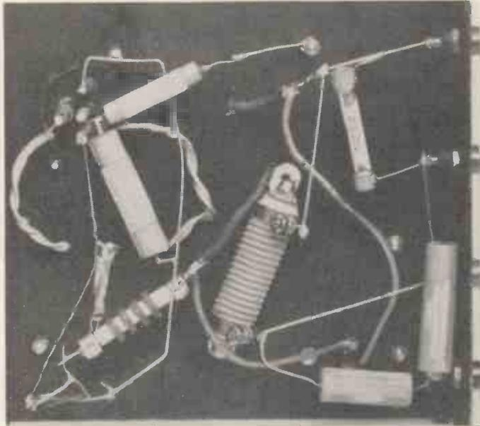
*Here is the unit partially wired. It is quite simple to connect and the condensers and resistances need not be mounted. For those needing a greater number of tappings we suggest the use of a Bulgin group board to take the various resistances.*
