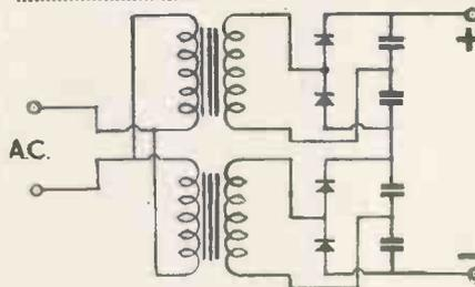
Fig. 6.—Metal rectifiers are a distinct advantage in a voltage-doubling circuit owing to the fact that no delayed switching is required.
