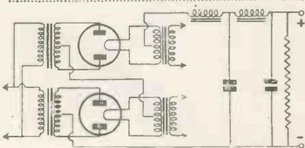
Fig. 5.—By using two transformers for high voltage the bridge circuit can be modified in this way.
