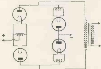
Fig. 4.—A bridge rectifier circuit using four half-wave valves enables twice the voltage output to be obtained.
