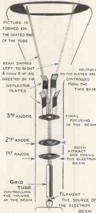
Here is a diagram of a cathode-ray tube showing the arrangement of the electrodes. The photograph shows the electrode assembly of a typical tube employed for television reception.
