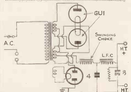
Fig. 3.—Mercury vapour valves must only be used with a choke input circuit and need some means of delayed switching.
