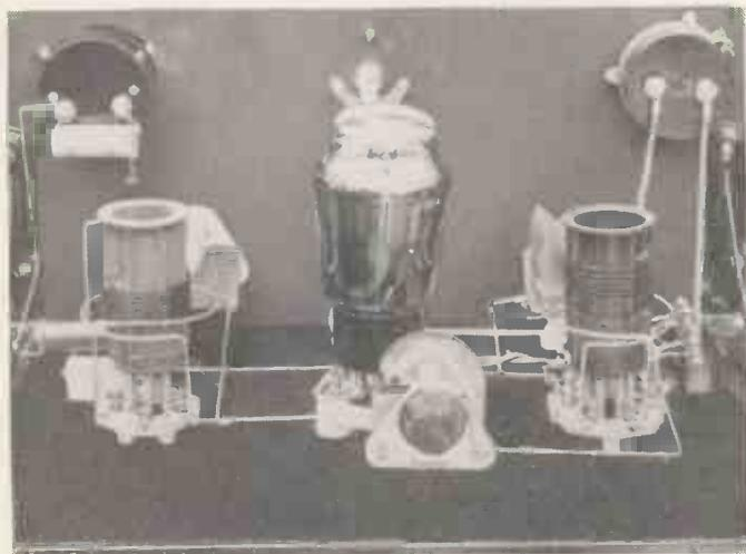
The doubler stage is quite straightforward, but again, link couplings are fixed to the coil holder and not the coil former. To reduce losses, mount the neutralising condenser in the wiring as shown.
