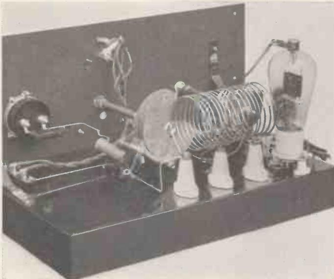
*An air-spaced coil is used in the grid circuit of the T20. This is very efficient and also allows for easy adjustment of the link coupling which is merely plugged in to the centre of the coil.*
