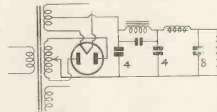
Fig. 2.—By tuning the first condenser and inductance circuit AC ripple can be completely removed.
