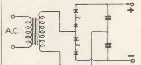
Fig. 7.—A high voltage transformer is required in this arrangement followed by a comparatively simple smoothing circuit.
