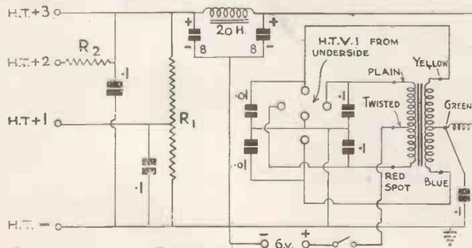
*Fig. 1. — The fundamental circuit cannot be modified but resistances  $R_1$  and  $R_2$  can be varied to give varying outputs.*
