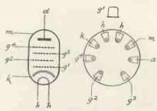
Here are the connections for the EF8 valve
