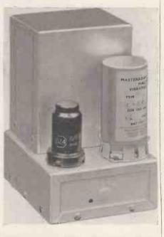
This is one of the Mallory-Masteradio vibrator power units. It includes as a rectifying valve the new filamentless Raytheon tpye AO4G.
