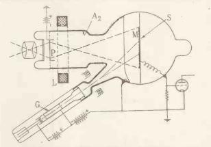
Fig. 6. Schematic diagram of the Super-Emitron.
