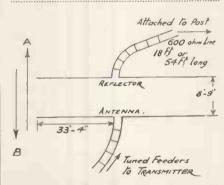
Fig. 2. Two half-waves in phase with parasitic elements.
