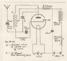
This is the remote control circuit using a new gas triode type RK-62.
