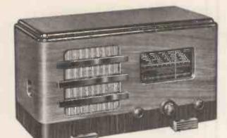
NEW receiver just introduced by A. C. Cossor, Ltd., is a 6valve superhet of modern design. Looking at the circuit, the aerial is inductively coupled to a variable-mu R.F. pentode connected to the A.V.C. line. The reason for this is to make more certain of the A.V.C. action. A stage of R.F. amplification is used on all bands while the coverage is 810-2,085 metres, 195-560 metres, and 18.7-5.7 megacycles.
