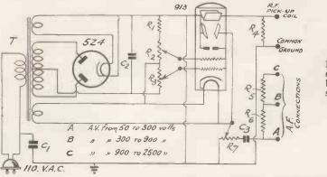
Fig. 4. This C.R. oscilloscope has been designed for simple modulation checking.
