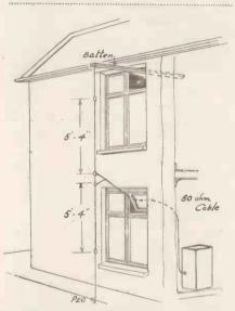
A simple di-pole consisting of two tensioned wires.
