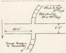
Fig. 3. Parasitic elements with phased halfwave radiators.
