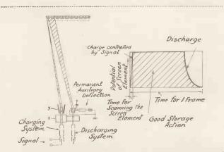
Fig. 6. Storage arrangement with two electron beams and good storage effect.
