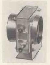
Light relay with crystal, showing angle-brass mount. (Note: In this photo the brass angle is turned the other way from that recommended in the drawings, as this was a first model, and drilled slightly differently.
