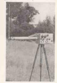
Marconi-Ekco field test equipment for ultrashort waves.
