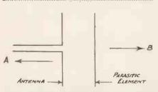
Fig. 1. Parasitic elements with phased radiators co-linear.
