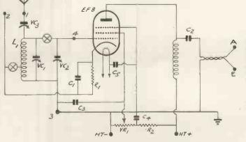
All the coil connections are carried out by the manufacturers so that this portion of the circuit only takes about half-anhour to complete.
