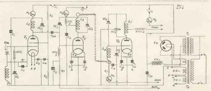
There are three stages in the transmitter which enable coverage to be obtained on four wavebands.
