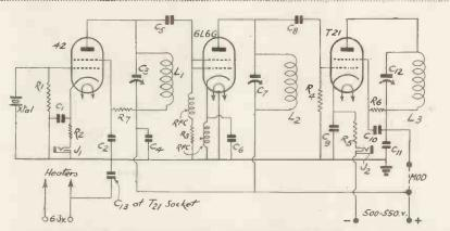
Fig. 3. This is one of the most interesting 5-metre exciters that there has been for some time. It provides high carrier power on 5 metres from a 40-metre crystal.
