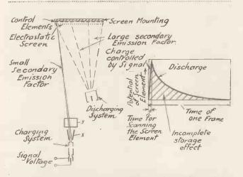
Fig. 5. Simple storage arrangement working with secondary emission.
