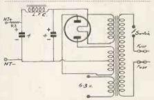
A power pack is optional, but here is the circuit if constructors wish to make the preselector self-contained.
