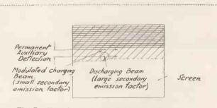
Fig. 7. How the potential distribution is built up.
