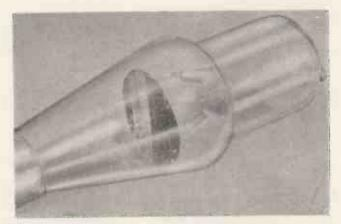
Fig. 2. Cathode-ray tube with different screen metals (Experimental tube for the investigation of charging times).
