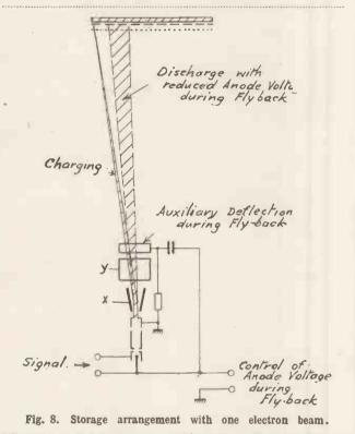
line with high electron velocity and high definition and produces the desired potential distribution; during the following short fly back the anode voltage is reduced and the spot is made to diffuse in order to effect the
