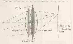
Fig. 3. Schematic diagram of receiver.
