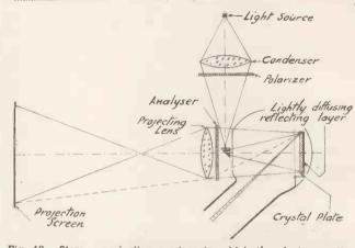
Fig. 13. Storage projection receiver in which the electron optical effect is doubled.
