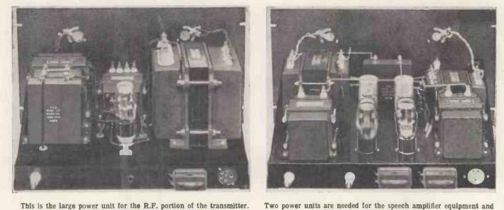
This is the large power unit for the R.F. portion of the transmitter. It provides between 700 and 750 volts at 250 m/A.
