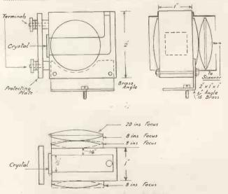
Constructional details of light relay cell.
