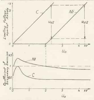
Fig. 1. Production of the control voltage U on an isolated screen element :
