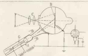
Fig. 1. Schematic diagram showing the constructional and operating principles of the Emitron.
