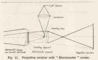
be used just as well as the secondary emission of metals. Thus the advantage is gained that there is no conducting layer at the front of the screen, only the back of the screen must have a conducting transparent layer as counter electrode, consisting, for example, of a thin metal film or of a layer of perfectly transparent zincoxide.
