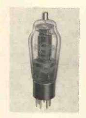
the output is approximately 38 watts. The anode-grid capacity is only 0.1 mmfd. while the total cathode-grid capacity is approximately 16.4 mmfd. This valve is provided with a 6.3 volt heater at which the current is approximately 1.3 amperes. A total emission of 800 mA is claimed.
