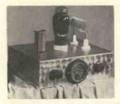
The portable transmitter used by LA1G with an input of 5 watts.
