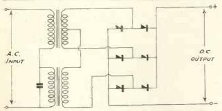
Fig. 1. This is the Noregg circuit which has an efficiency of 70-per cent, and a power factor of 0.94.
