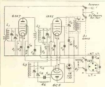
Fig. 4. Two of the latest valves are used in this convertor designed to provide high efficiency on the U.H.F. bands up to about 80 megacycles. Notice also the voltage stabiliser in the oscillator circuit which accounts in a certain degree to lack of frequency drift. A special type of output transformer is also employed.
