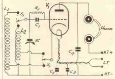
Fig. 1. The single valve C.W. monitor.
