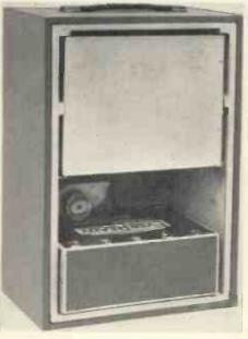
It can be seen that the receiver is completely screened and that there is a gap on either side of at least half an inch to keep the metal away as far as possible from the frame aerial.
