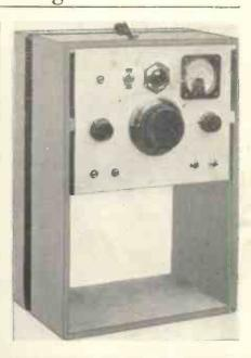
A special plug-in socket, both halves of which are screened, is used to connect the frame aerial into the grid circuits of the H.F. amplifiers. Controls are bottom row, condensers C5 and C6, plus two jacks for headphones wired in parallel. Centre row, switch S1, tuner C7, and reaction. Top row, frame aerial trimmer, C1, on-off switch, dial light and valve meter indicator. All references are from left to right.
