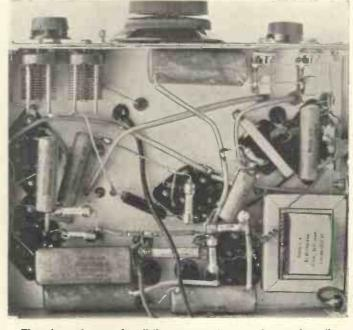
The actual receiver itself is quite small, and in this view can be seen the output pentode, detector and valve voltmeter valve.
