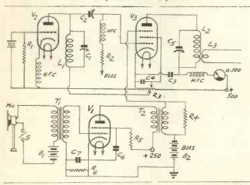
Fig. 4. With this arrangement the transmitter has been designed for telephony use and to run from A.C. mains.
