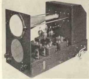
Fig. 1. This photograph shows the kit completely assembled,
