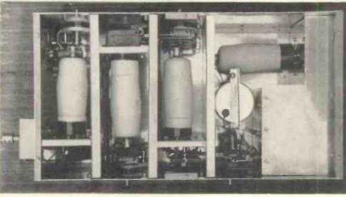
Fig. 2. The interior of the vision unit, Note the staggered mounting of the valves and the screened V.F. compartment.
