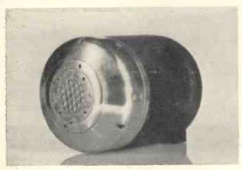
Fig. 4. Movingmicrophone coil used at Alexandra Palace.
