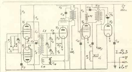
A push-pull R.F. stage is used so as to include a balanced centre tapped frame aerial. Notice also the valve voltmeter circuit.
