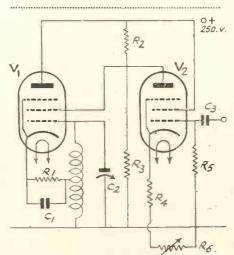
Circuit diagram of modulated oscillator.
