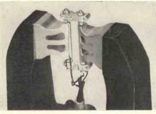
Fig. 4a. Pole piece and ribbon assembly of ribbon-type microphone.
