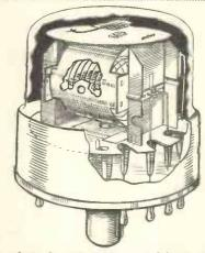
The electrode system is mounted horizontally with a cylindrical grid and anode in this manner.
