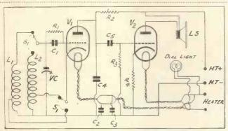
Fig. 2. A suggested two-valve C.W. monitor suitable for feeding a loudspeaker.
