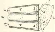
Transmitting tube with mozaic of metal elements. Patent No. 500,430.
