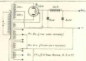
Fig. 2b. The circuit diagram of the vision unit power supply. The mains transformer includes windings for the heaters of the time base valves and for the C.R. tube. Only normal insulation is required for the latter winding as the C.R. tube is operated with an earthed cathode.
