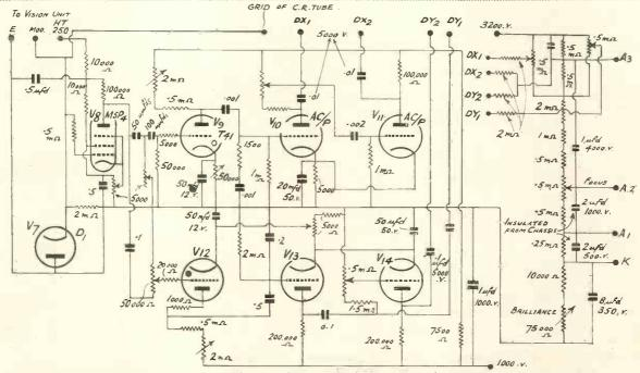
Fig. 6a. The complete circuit diagram of the time base, the sync. filter and the C.R. tube circuits is given above.
