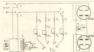
Fig. 1. This meter will read up to 1,000 volts and the resistance values are as follows: R1 5,000 ohms, R2 1,000 ohms, R3 70,000 ohms, R4, 15,000 ohms, R5 200,000 ohms, R6 25,000 ohms, R7 50,000 ohms, R8 800,000 ohms, 100,000 ohms.
