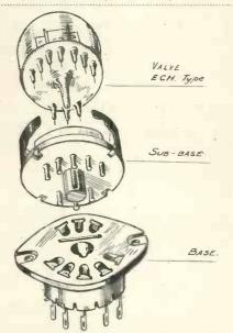
This special drawing shows the glass bulb and lead out wires underneath which is the sub-base and finally the new type of valve holder.
