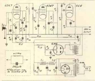
Fig. 3. In the heart of this amplifier is the simple volume compressor built around the 6H6 double diode. It requires a positive voltage of between zero and 30 to give complete variable compression.
