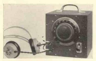
This is the C.W. monitor built in a special Peto-Scott metal cabinet which is only 6 ins. cube.
