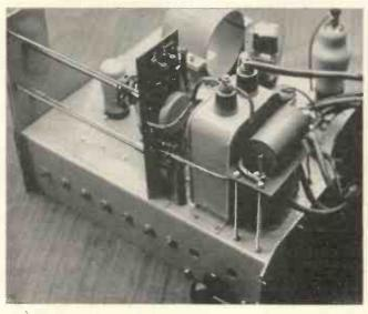
Fig. 9. The above photograph shows the arrangement of the C.R. tube's potential divider. Note the mounting of the smoothing condensers to ensure these are insulated from chassis.
