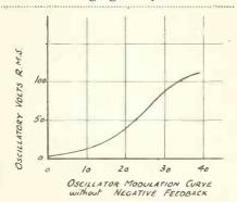
Oscillator modulation curve without negative feed-back.
