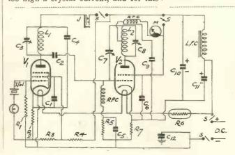
Fig. 5. For those who are limited to operation from D.C. mains this transmitter should prove very serviceable. The output is low but no additional batteries are needed.
