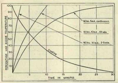
Fig. 10. Heating and cooling curves of target under various load conditions.
