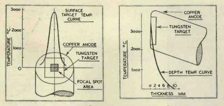
Figs. 6 (left) and 7 (right). Temperature curves of a tungsten-copper target showing variation across the surface and with target thickness.
