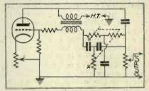
Fig. 4. Audio-frequency Oscillator using parallel-T network.
