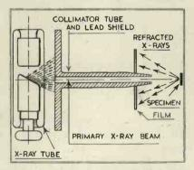
Fig. I. Method of obtaining crystallograms by back reflexion.
