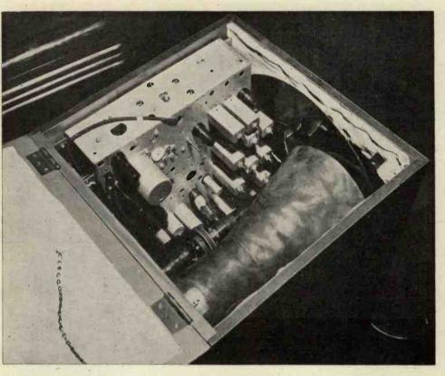
Fig. 11. The interior view of a 9" colour television receiver showing filter disk and cathode ray tube (lower right).
