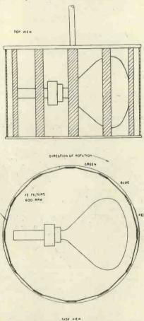
Fig. 14. Diagrammatic view of drum receiver for colour celevision.
