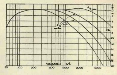
Fig. 35. Effect of tone control  $R_{13}$   $C_{17}$  (Fig. 34) on audio frequency response.
