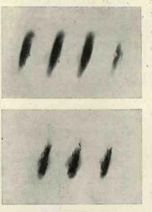
Fig. 4. Photographs of tube filaments. Above : Good filaments. Below : After ion bombardment.
