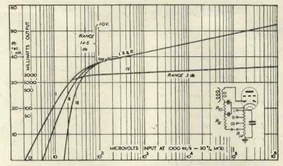
Fig. 33. A.V.C. characteristics. (i) For two controlled stages of conventional receiver with -3 v. delay. (ii) as (i) but with -1 v. at signal diode. (iii) With -1.5v. (iv) Is the same as (i) but with A.V.C. also applied to the Ist A.F. stage.
