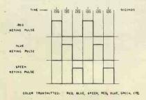
Fig. 8. Colour mixer pulse diagram.
