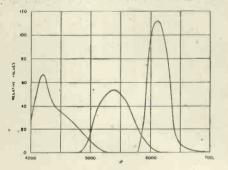
Fig. 4 (above). Colour characteristics at the transmitter: the curves combine the standard dissector, the carbon arc, 2 mm. of Corning glass No. 978 and Wratten filters Nos. 25, 47 and 58.
