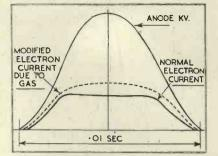
Fig. 3. Effect of gas in increasing emission over a half-cycle of anode voltage.
