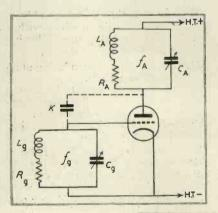
Fig. 2 (above), Circuit of tuned anode-tuned grid oscillator and Fig. 3 (right) the equivalent circuit.
