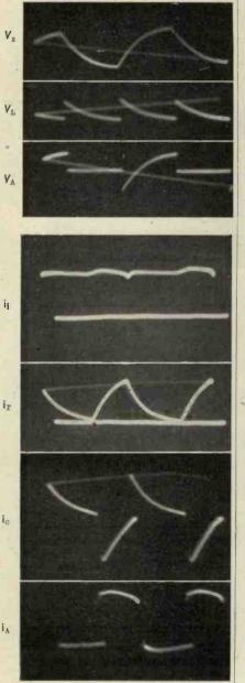
Fig. 4. Oscillograms of the voltages and currents at various points in the circuit. The lettering against each oscillogram corresponds to the lettering on the circuit diagram.
