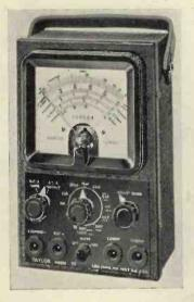
THE improved Model 90 is a universal test meter for general radio and electrical work giving a wide range of voltage and current measurements on A.C. and D.C. A resistance scale is also provided and an output scale calibrated in decibels, making a total of 38 ranges.
