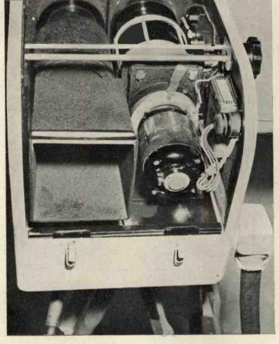
Fig. 6. Orthicon colour camera; inside view showing the filter drum with synchronous driving motor.
