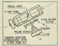
Fig. 8. Method of obtaining photograph of target.
