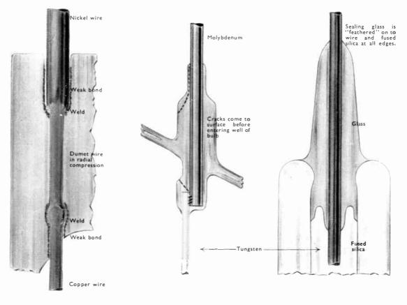
Fig. 6. Rod seal of copper-Dumet-nickel through C.12 glass.
