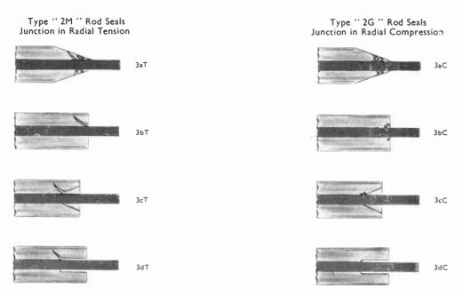
Fig. 3. Crack systems for '' rod '' seals loaded mechanically so that the free end of the rod is bent downwards.
