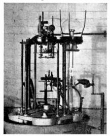
Fig. 7. Four-head drop sealing machine.
