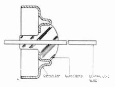
Fig. 1. Sectional drawing of glass-metal seal.
