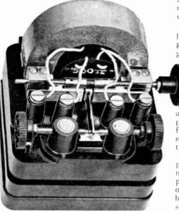
HIGH speed relay developed by the Automatic Telegraph and Radio Transceiver Co., Ltd., combines small overall dimensions with a high sensitivity and a recorded working speed of 1,000 w.p.m.
