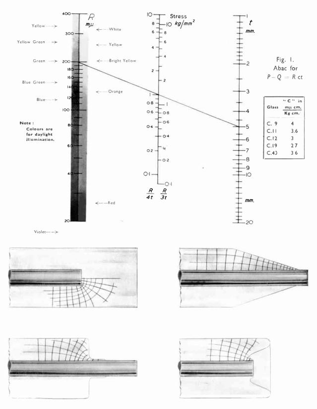
Fig. 2. Lines of principal stress for four "rod " seals.
