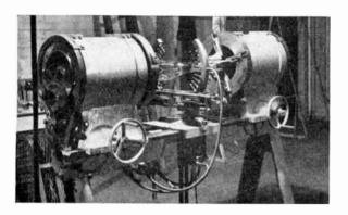
Fig. 9. Large sealing lathe for tubes.
