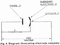
in X-ray tube for high speed radiography.
