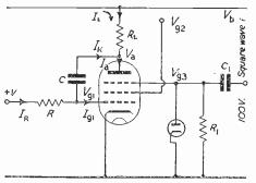
Fig. 3. Control of Miller valve by suppressor switching. The waveform at the various points in the circuit is shown in the diagram below
