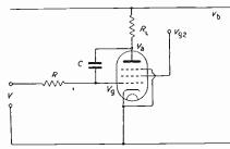
Fig. 2. " Miller Valve " circuit, using single pentode
