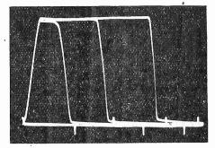
Fig. 3. Composite photograph of curves of a three speed shutter/using logarithmic time base. (1/25th, 1/50th and 1/100th)
