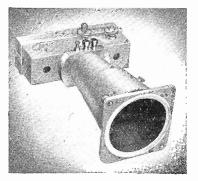
Specially developed for use with Cossor Oscillographs, it provides the simplest means of recording stationary or non-recurrent waveform<sup>S</sup> and slow transients by the moving film method on standard perforated 35 mm. film or paper. Of robust construction it has provision for power drive by the Cossor Three-Speed Motor Attachment, Model 1429.
