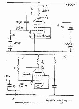
The bottomed state continues until the point D', when anode current is cut off, and the usual exponential recovery takes place. (There is no positive jump in this case, because the grid is already at earth potential, and drawing grid current).
