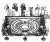
CIRCUIT The new R.F.103 chassis largely removes the difficulty of separating stations after dark as the stages of I.F. two amplification with variable selectivity permit o a maximum selectivity better than 6 Kc/s. On the short wavebands the actual sensitivity is 8 micro volts. It will be appreciated that this chassis has a perform-
