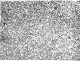
Fig. 2a. Longitudinal view of swaged tungsten rod (etched with alkaline potassium ferricyanide)
