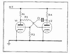
Fig. 3. New circuit for free-running multivibrator
