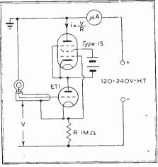
Fig. 4. Farmer valve electrometer
