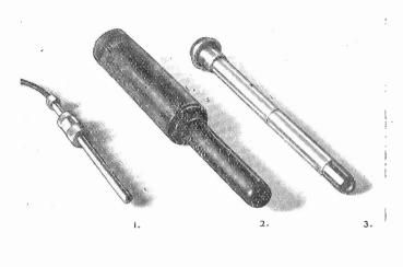
Fig. 8. Ionisation chambers for integrating dosemeters (1) Farmer (2) Hammer (3) Mekapion
