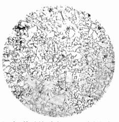
Fig. Ic. Hard Metal, 6 per cent cobalt (etched with alkaline potassium ferricyanide)
