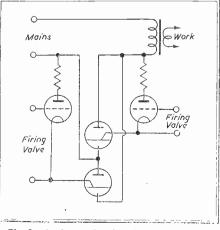
Fig. 2. Ignitron circuit using thyratrons as control valves
