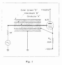
If  $R_K$  is made large then the output impedance of the cathode follower is  $1/g_m$  or  $R_V/\mu$ . Therefore, at a frequency f the phase delay  $\phi$  of the cathode waveform relative to the grid waveform is given by :
