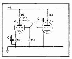
Fig. 5. Multivibrator circuit of Fig. 3, with ddition of self-bias combination C. R.
