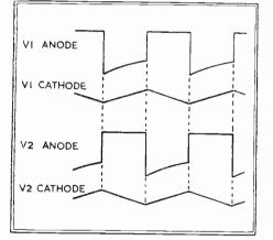
Fig. 2. Anode, cathode wave-forms produced by multivibrator circuit shown in Fig. I above
