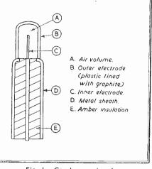
Fig. I. Condenser chamber
