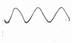
Fig. 4. Oscillogram of sine wave applied to Y plates showing linearity of sweep
