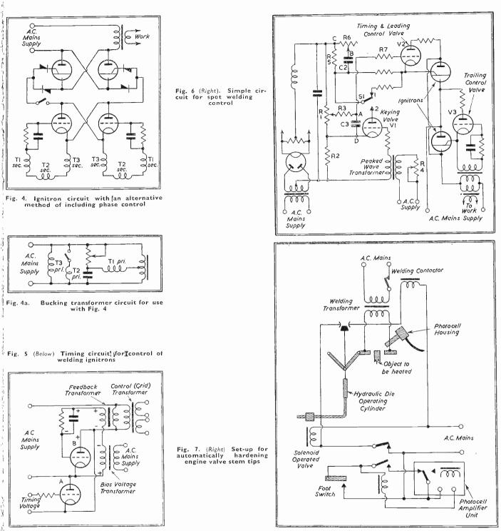
If the grid of valve A is positive when its anode is positive, current will flow for half a cycle. This supplies power to the feedback transformer and, due to the inductance of the primary of the control transformer, the current wave will lag behind the voltage wave. This means that when the current through the valve A falls to zero there will be a positive voltage on
