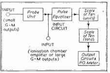
Fig. 13." Schematic diagram of pulse counting unit
