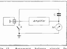
Fig. 12. Automatic balance circuit for measurement of ionisation currents (diagrammatic)
