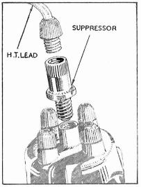
The sketch shows the simple method of fixing the "Belling-Lee" distributor lead suppressor L630 which sell at 2/each
