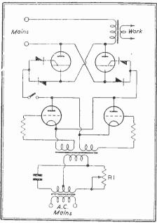
Fig. 3. Ignitron circuit with simple phase control
