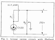
Fig. 3. Linear sweep circuit with Multar CV 20 photo-cell Component Values  $R_{\tau}$  15 M  $\pm 20\%^{-1}/_{10}$  watt.
