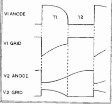
Fig. 4. Anode, grid wave-forms produced by multivibrator circuit shown in Fig. 2
