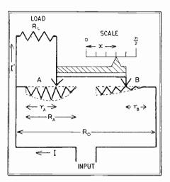
The required properties—that  $I'/I = \phi(x)$ , where x = shaft deflection,  $\phi(\cdot)$  the chosen function; and that  $R_{\circ} =$  const., are obtained if A and B are graded so that
