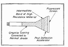
Fig. 2. Practical form of P.D.A. tube
