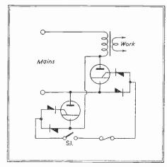
Fig. I. Simple ignitron circuit without phase or timing control
