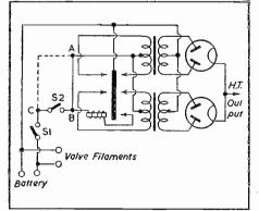
The L.T. current taken by the interrupter may, in 6-volt operation, be of the order of 15 amps., and thus the switch  $S_2$  will have to be capable of carrying this current and consequently a heavy duty switch with substantial contacts will be required.
