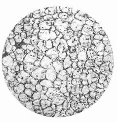
Fig. 1b. Sintered ferro-copper, 25 per cent copper (etched with 5 per cent nitric acid in alcohol)
