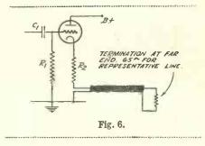
sufficient to terminate the cable at one end only.
