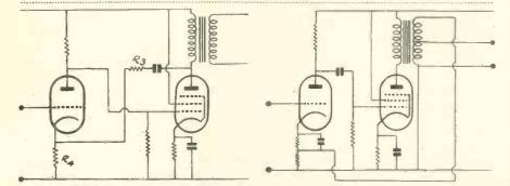
Fig. 3. Two methods of feeding back into a preceding stage. 3b corresponds to b of Fig. 2.
