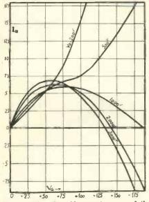
Fig. 6. Grid-volts-grid-current curves of the Tungsram 0-300/3,000 showing the effect of secondary emission from the grid.
