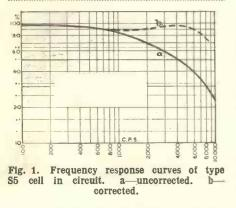
method is by the use of barrier-layer sound head cells, and the Tungsram types S5 and S5X have been produced for this and similar purposes. Two advantages are their small size (total length is only 32 mm. and diameter about 15 mm.), and the large electrical output which obviates the need
