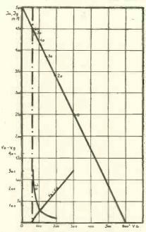
Fig. 10. Anode-voltage-grid and anodecurrent curve limits showing smallest permissible anode-load line of Tungsram type QP-37/600.
