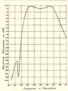
Fig. 6. Overall response curve of a television receiver showing the attenuation of the sound signal by using one of the circuits of Fig. 5.
