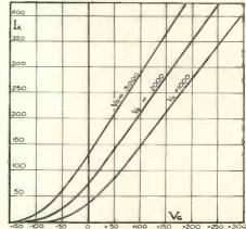
Fig. 4. Grid-volts-anode-current curve of the Tungsram 0-300/3,000 U.S.W. transmitting triode extending above the dissipation limit.
