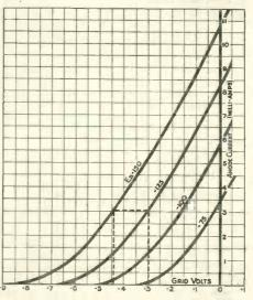
Fig. 1. Characteristic of triode from which the various constants can be measured.
