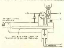
Single-tuned-circuit oscillator, cathode-aboveearth type. The frequency can be varied either by the optional tuning condenser shown or by varying the length of the inner conductor of the concentric line.
