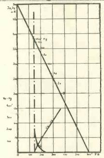
Fig. 11. Anode-voltage-grid and anodecurrent curve limits showing smallest permissible anode-load line of Tungsram type P-25/450.
