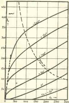
Anode-volts-anode-current curves of Fig. 5, the Tungsram 0-300/3,000.
