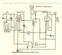
Wiring diagram of the printing timer.
