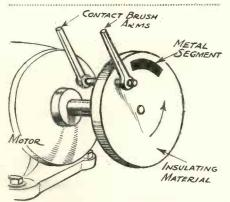
Fig. 2. Motor-driven rotary switch (shown as S in Fig. 1) for rapidly changing the grid bias.
