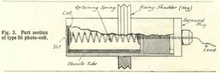
This barrier-layer selenium cell has a sensitive area of only 5 by I mm. arranged as a slit on the metal housing; it has a frequency response equivalent to the average wireless set, in other words, tolerable quality sufficiently good for the average listener.
