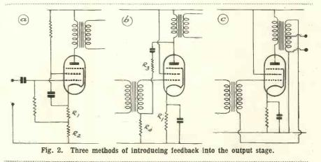
the feed-back network has a constant phase frequency characteristic up to the frequency of the highest harmonic it is desired to reduce, and that no valve in the amplifier is run either into grid current or off its characteristic.
