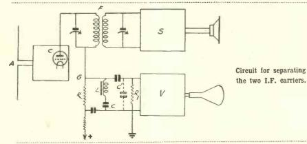
offering a high impedance to them, but which present only a low impedance to the vision signals and so allow them to pass. On the other hand, the vision filter G by reason of the series resonance circuit formed by the inductance L and capacity C tuned to the sound intermediate-frequency carrier takes negligible account of the sound signals, but offers relatively high impedance to a
