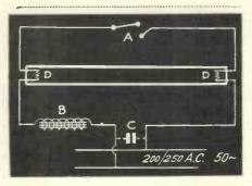
Diagram showing method of connecting discharge to the mains
