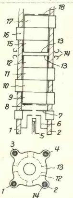
Fig. 1. Electrode supporting system of high-voltage cathode-ray tube shown in elevation and plan.
