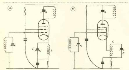
Fig. 5. The application of negative feedback to r.f. amplifiers, with cathode tuned circuit.
