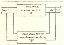
Fig. 1. Illustrating the principle of negative feedback.
