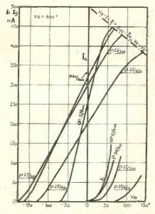
Fig. 12. Grid-volts-anode and grid current curves of several Tungsram types of the 25-37 watts category, taken with the smallest permissible anode load.  $R_L = 1,200$  ohms.
