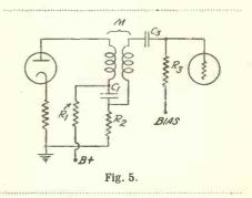
it is found convenient to use the degenerative or cathode-loaded amplifier. In this case, the principal reasons for using it are to provide a low-output impedance, and also to maintain the cable near ground potential insofar as direct current is concerned.
