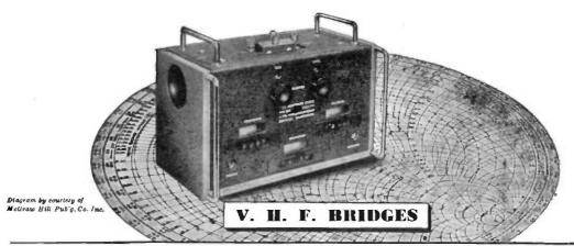
for balanced and unbalanced measurement at frequencies between 1 Mc/s and 100 Mc/s.
