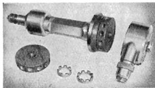
The complete air turbine hand-grinder showing the rotor separately in the left foreground. The ball-race cages are also of Tufnol.
