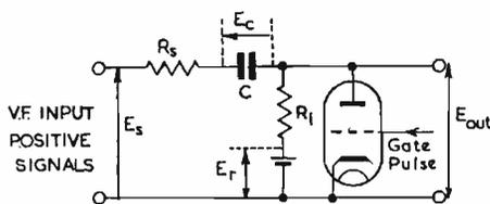
Fig. 16. Black level restoration circuit
