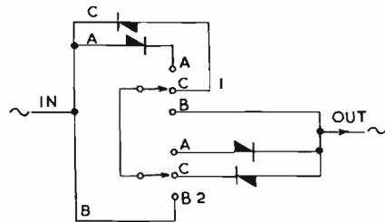
Fig. 5. Single pole interlock for two switches having three positions. Rectifiers are not essential for ensuring correct indication in position B
