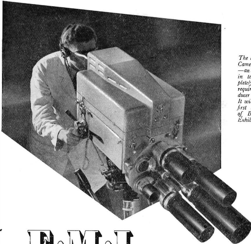
*The latest C.P.S. Emitron Camera with 6 lens turret — an entirely new conception in television which completely satisfies the exacting requirements of both producer and operator. It will be in action for the first time at the Festival of Britain, South Bank Exhibition.*
