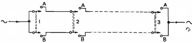
Fig. 1. Conventional two-position interlock (two switch poles used). Circuit is made only with "all A's" or "all B's"
