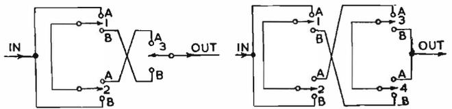
Fig. 3. Interlocking of three switches
