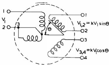
Fig. 5. Resolver No. 1. Resolution of polars to cartesians
