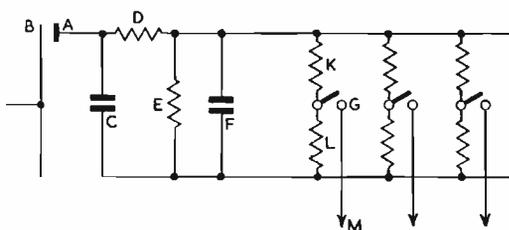
Fig. 4. Circuit of electrical network for different polarizing voltages
