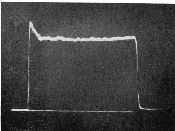
load conditions is shown in Fig. 2. The arc voltage is represented by the height of the oscillograph deflexion above the base line. This height may, of course, be measured by applying a variable known sinusoidal voltage to the input of the amplifier and drawing a calibration curve of the whole apparatus.
