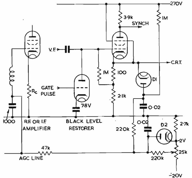
Fig. 24 (Right). Suggested circuit for applying A.G.C. to a television receiver. Diode D2 protects the receiver valves during the absence of signals.  $R_c$  stabilizes the input capacitance of the controlled stage
