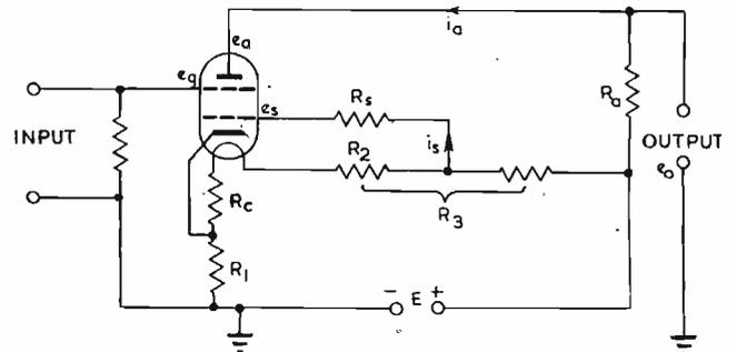
Fig. 3. Caldwell circuit with input resistor for current measurement by direct deflexion method
