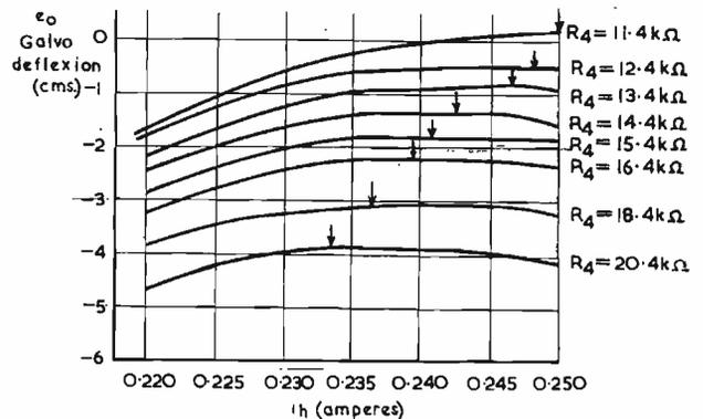
Fig. 6. Barth circuit—variation of balance point with R<sub>4</sub>
