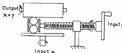
Fig. 2. Mechanical multiplication
