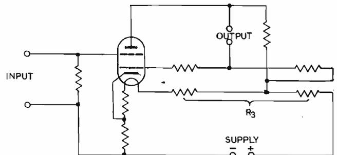
Fig. 1. Dubridge and Brown circuit, with input resistor for current measurement by direct deflexion method
