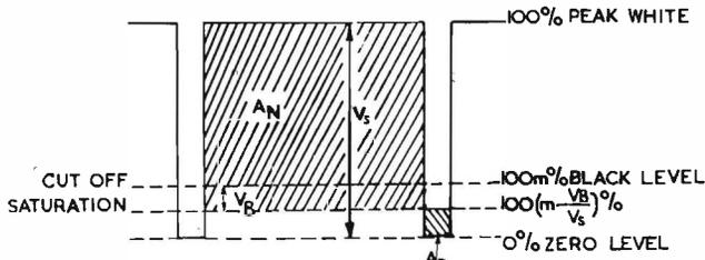
Fig. 15. Assumed operating conditions of a double limiter when designed for maximum rejection of noise modulation
