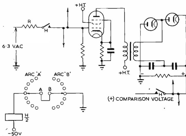
Fig. 7. Measurement of the heater voltage
