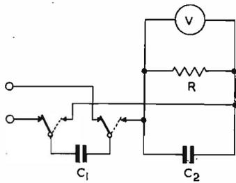
Fig. 8. Electrical rate measurement
