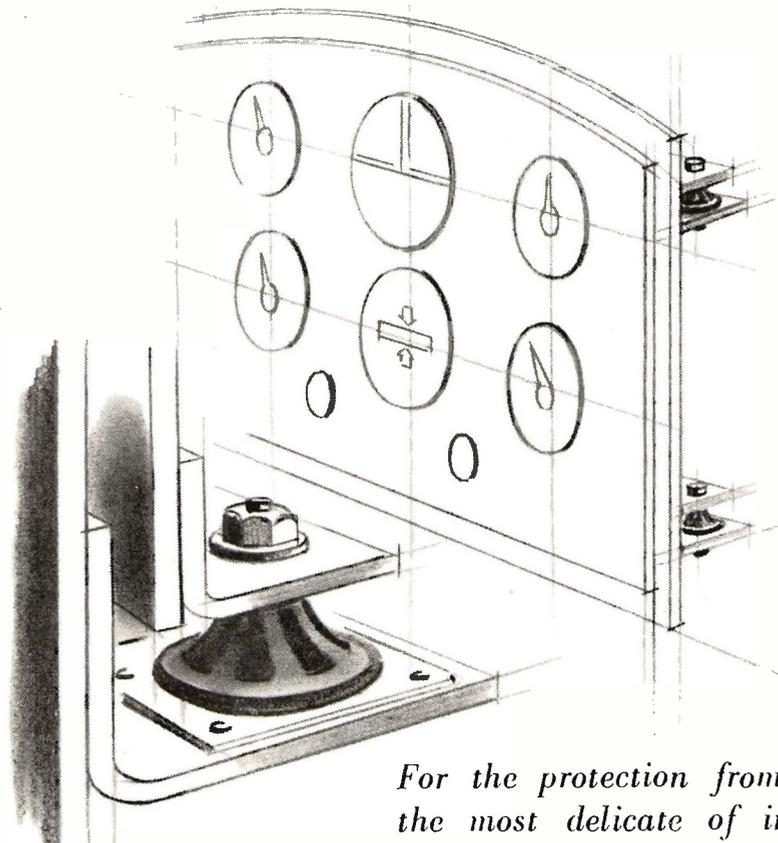
*For the protection from shock of the most delicate of instruments and of panels which are subject to vibration, this range of "Flexilant" light mountings is at your service. Have you any problems where we could help?*
