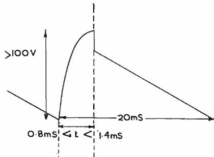
Fig. 21. A typical waveform present at the anode of a frame time base output valve
