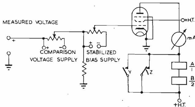
Fig. 1. Principle of the measuring circuit
