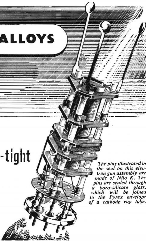
The pins illustrated in the seal on this electron gun assembly are made of Nilo K. The pins are sealed through a boro-silicate glass, which will be joined to the Pyrex envelope of a cathode ray tube.
