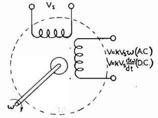
Fig. 7. Induction generator. Voltage proportional to speed with A.C. supply. Voltage proportional to acceleration with D.C. supply
