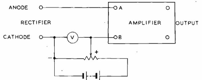
Fig. 3. Connexions for arc voltage measurement
