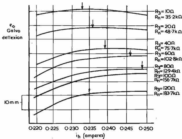
Fig. 4. Barth circuit—determination of minimum value of R<sub>3</sub> necessary for balance (the vertical separation of the curves is arbitrary)
