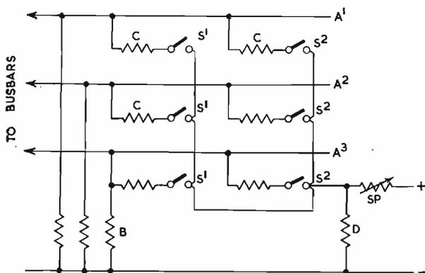
Fig. 5. Stop circuit
