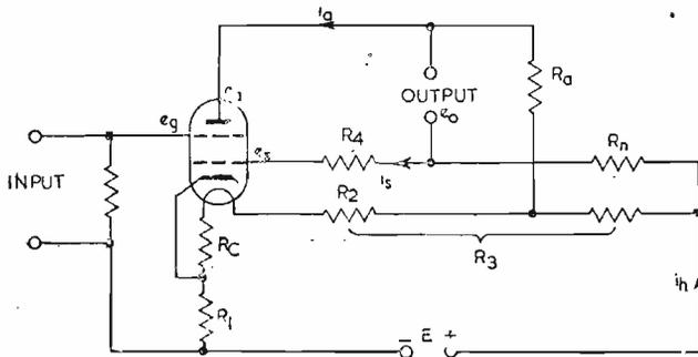
Fig. 2. Barth circuit with input resistor for current measurement by direct deflexion method
