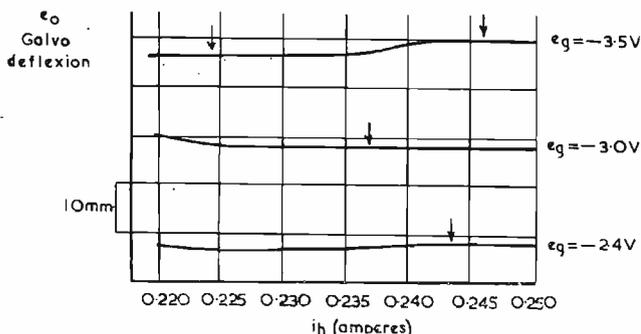
Fig. 8. Caldwell circuit—variation of balance point with control grid potential (the vertical separation of the curves is arbitrary)
