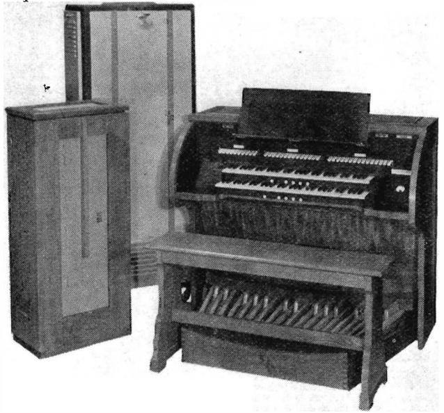
*The console, generator rack and loudspeaker cabinet of the Compton Electrone*
