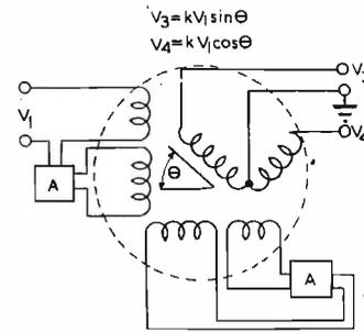
Fig. 6. Resolver No. 2. Resolution of polars to cartesians
