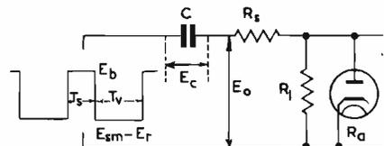
Fig. 17. Equivalent circuit of Fig. 16 referred to in the text
