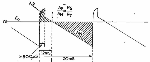
Fig. 23. Equivalent waveform  $E_0$  obtained when the anode waveform of a short flyback frame time base is passed onto the clamp valve grid via a resistance ratio  $R6 : R7$  of Fig. 20
