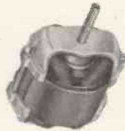
h.p. Measuring 2in x 3in with a ½in long shaft the motor weighs 8oz. It is precision built with a ground shaft mounted in sintered bearings and requires no maintenance.
