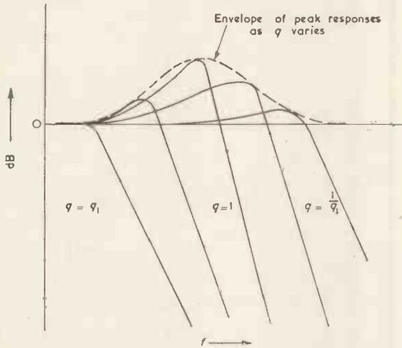
Fig. 7. Variation of response of single variable element low-pass 12dB/octave filter with variation of  $q$  from  $q_1$  to  $1/q_1$  (see Table 1)
