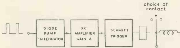
Fig. 11. Block diagram of frequency-sensitive relay
