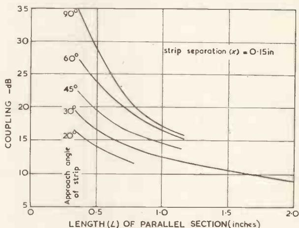
Fig. 7. Coupling against parallel section of strip line
