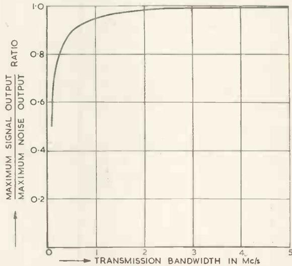
Fig. 9. Variation of output peak signal-to-noise ratio with transmission bandwidth
