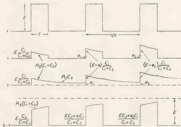
Fig. 7. Waveforms of complete integrator circuit
