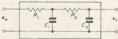
Fig. 5. Two section RC network—low-pass
