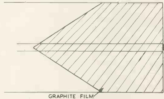
Fig. 4. Strip line termination
