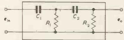
Fig. 6. Two section RC network—high-pass
