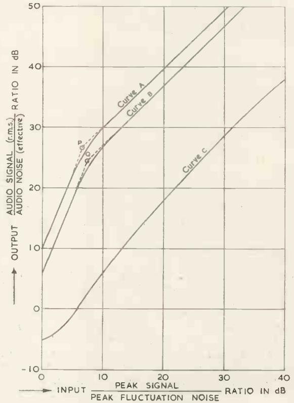
Fig. 7. Experimental values of signal-to-noise ratios
