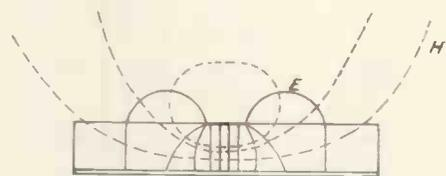
Fig. 3. Field configuration of an open strip line
