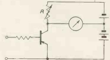
Fig. 1. Transistor voltmeter showing bridge arrangement
