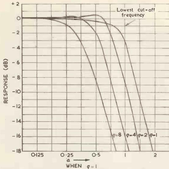
Fig. 9. Response of single-variable-element 18dB/octave filter  $q_1 = 8:1 + \beta M = 5.5$
