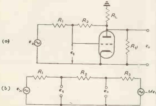
Fig. 13(a). Negative feedback over single stage
