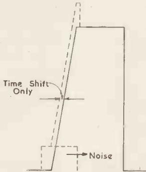
Fig. 2. Effect of rectangular noise pulses on p.s.m.
