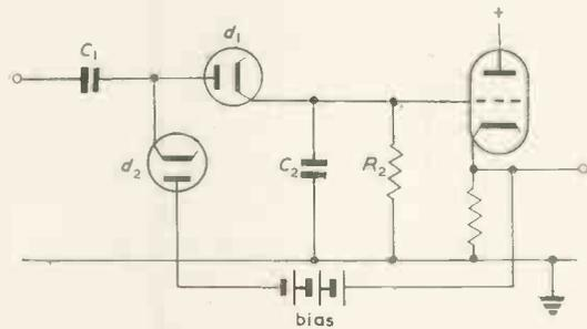
Fig. 9. Circuit for linear relationship between  $v$  and  $n$ .
