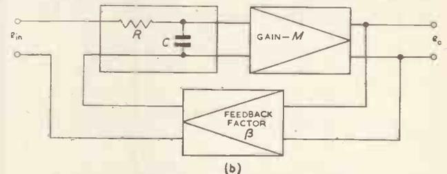
(b) Feedback amplifier with single section low-pass RC network in the forward path
