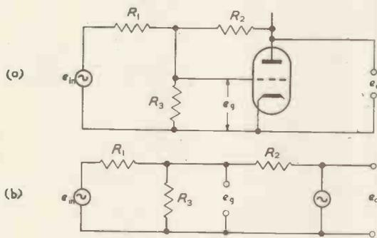
Fig. 14(a). Negative feedback assuming zero output impedance and finite input impedance
