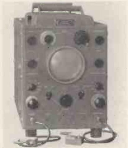
Nine calibrated sweeps are available with durations of 0.5 $\mu$ sec to 1msec. The Y shift control is calibrated directly in microseconds. Direct, amplified and delayed triggering facilities are provided.
