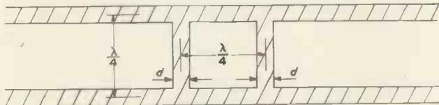
Fig. 8. A possible 3dB strip line coupler
