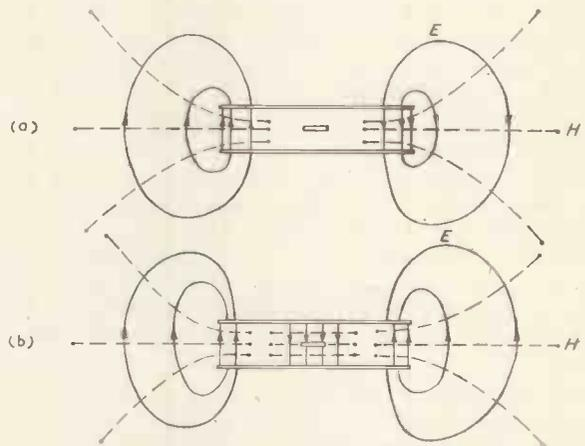
Fig. 2. Possible field configurations of sandwich strip line
