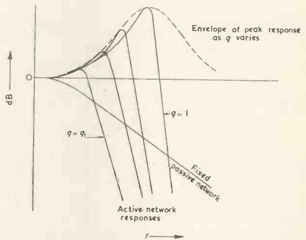
Fig. 8. Responses of component parts of single-variable element low-pass 18dB/octave filter
