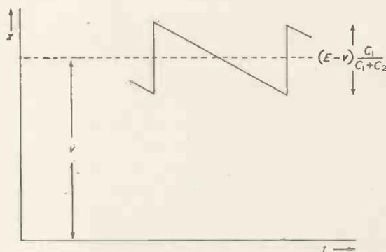
Fig. 8. Integrator output waveform
