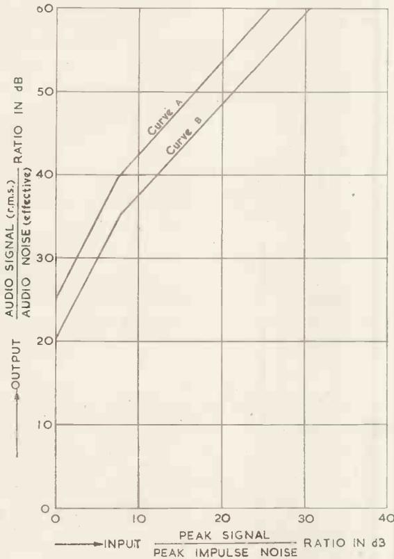
Fig. 8. Experimental values of impulse noise tests
