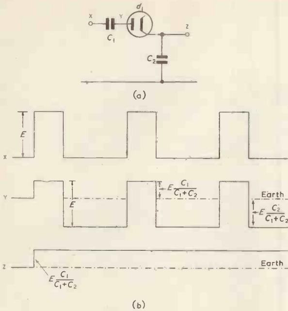
Fig. 3. Introduction of diode into integrator circuit
