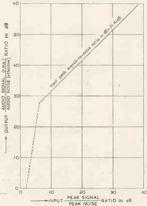
Fig. 6. Theoretical signal-to-noise ratio
