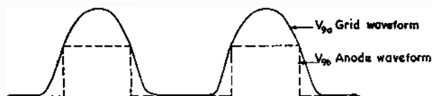
Fig. 3. Grid and anode waveforms of V_1 .
