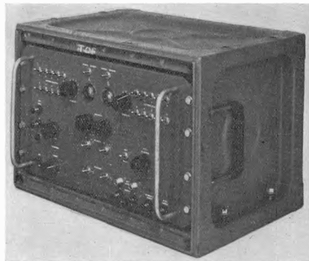
The complete pattern generator
