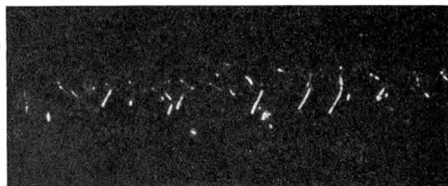
Fig. 3. Filament of an AV33 diode which has developed a crystalline structure after operating on d.c. Magnification 450. Total operating time 95 days
