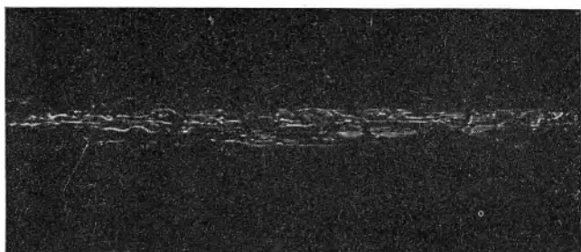
Fig. 4. Filament of a 29C1 valve after running for an appreciable time on a.c. Magnification 450
