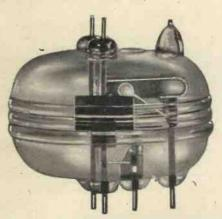
Fig. 6. Ultra-short-wave oscillator showing double lead-out from electrodes. Due to this construction, oscillations can be produced up to 1,800 Mc/sec. (Western Electric Co. D.156548.)
