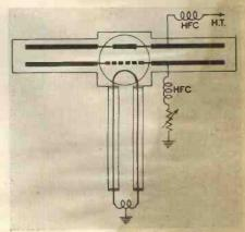
Fig. 4. Circuit recommended for use with valves of the 3B250 type. (See Fig. 6).
