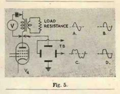
under these conditions the square of the voltage measured by the A.C. voltmeter, divided by the anode load of the valve will indicate the watts output. If the power is calculated for a condition as shown in C, it will contain a very high percentage of 3rd harmonic which is most undesirable. The other condition as illustrated in D is due to grid current as a result of excessive input.
