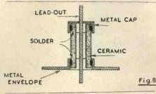
filled with a solder such as silver, in a powder or wire form. The whole is then heated in a reducing atmosphere or vacuum, the solder taking to the metal and the ceramic, thus forming a vacuum-tight joint.
