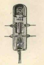
Fig. 7. R.C.A. ultra-short-wave valve type 1628, capable of delivering 34 W. at 500 Mc/sec.
