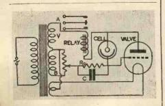
Fig. 4. Circuit for operation of cell from A.C. mains.
