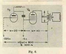
Sensitivity of the 1st L.F. stage is now measured by injecting a 400 c.p.s. signal into the grid of V3 and adjusting the input until a level of 50 mW is reached in the output load. For the receiver circuit shown in Fig. 1 this was in the region of .025 volt and this now enables to calculate the overall L.F. voltage gain (Fig. 6) to be calculated.
