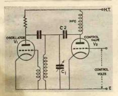
Fig. 2. Valve used as damping resistance.
