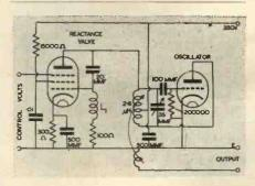
Fig. 4b. Circuit of 20-Mc/s. oscillator.
