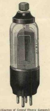
Fig. 1. Typical photo-cell.
