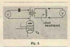
lower it will be necessary to check anode and bias potentials and if these are in order the output transformer may be suspected for either serious mismatching or shorted turns.
