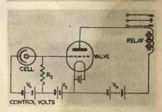
Fig. 3. Photo-cell circuit which operates when light is cut off.
