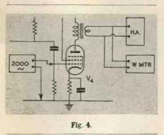
indicates directly the percentage of 2nd and 3rd harmonics contained in the output. The distortion does not vary very much with frequency, but if this test is carried out at about 1,000 to 2,000 cycles, a good idea of the average distortion will be obtained.
