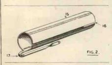
The shield 15, shown separately in Fig. 2 has a gap 16 extending along its entire length so that it does not present closed current paths linked with the magnetic flux surrounding coil 10.
