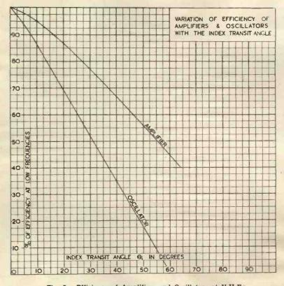
Fig. 5. Efficiency of Amplifiers and Oscillators at U.H.F.  $\theta_t = \omega T_t = (T_t/T_p) \times 360^\circ$ .  $T_t = Transit Time F-G, calculated on peak grid volts.$  $T_p = Period of R.F.$  wave.
