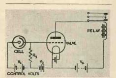
Fig. 2. Photo-cell circuit which operates relay when cell is illuminated.
