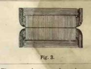
Figure 2 shows a plan view of a single saddle coil, H, with one of the halves of the sheath, S, and one vertical scanning coil, V, wound on it placed in position over the saddle coil. Figure 3 shows a side elevation of the whole assembly.
