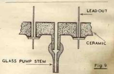
of one of the specially designed glasses, to a bush on the envelope of the valve (see Fig. 9). This again, however, reintroduces certain undesirable factors into the manufacture of the valve.
