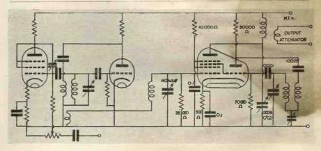
Fig. 6. Circuit diagram of complete frequency modulator.
