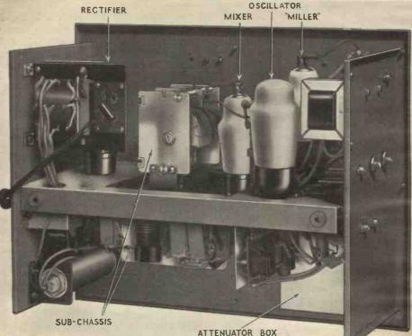
operating on the curved part of its characteristic, so that the change in frequency of the oscillator is linear with respect to the control voltage. This control voltage is applied to the grid of the Miller valve, but is prevented from grid-modulating the oscillator by the low capacity of  $C_2$ .  $C_1$  has an optimum value which determines to some extent both the linearity and the amount of frequency sweep for a given control voltage.
