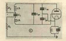
Fig. 2 (C). Equivalent circuit of the Colpitts oscillator of Fig. 2 (A).
