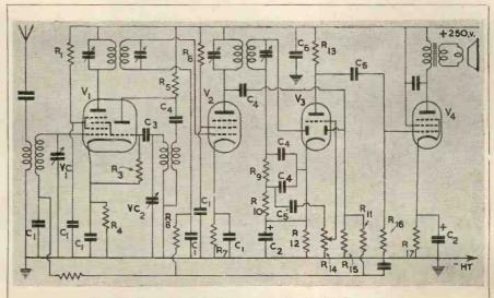
Fig. 1. Typical circuit diagram of a standard radio receiver.
