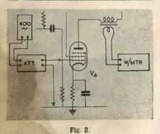
For a valve of the PENA4 class, about 0.3 volt input should produce 50 mW output, but in practice the sensitivity may be of the order of .4 or .5 of a volt. This can be due to variations in valves and/or in some cases transformer efficiency, which can vary so much in practice with different makes that it is difficult to give a definite figure.
