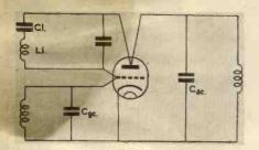
Fig. 1. "Coil-neutralized" circuit in which the grid-anode capacity is converted into a high resistance by resonating with the inductance L1.
