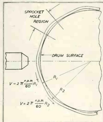
Fig. 6. Polygoning of a Film when flexed around a Drum.
