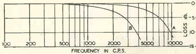
Fig. 3. Sound-track Losses due to Light Scatter: (a) 35 mm. Positive Emulsion, (b) same emulsion run at 16 mm. speed. (From Jour. S.M.P.E.)
