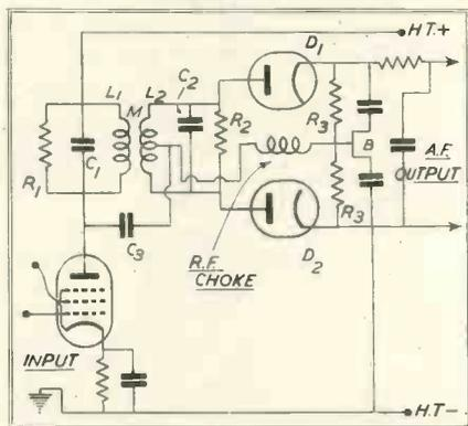
Fig. 5. The phase discriminator as a frequency-amplitude converter.
