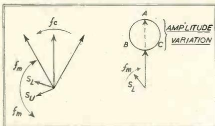
Fig. 2. Frequency Amplitude conversion by suppression of one sideband.
