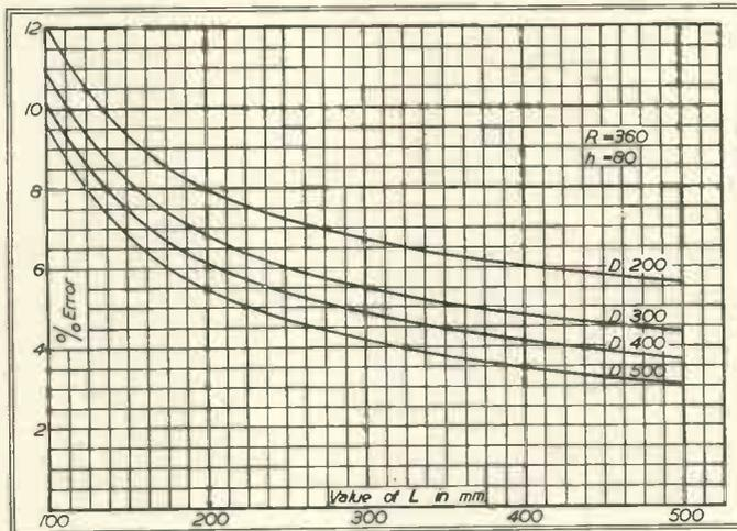
Fig. 5. Curves of per cent. error plotted for various values of L, the plate-screen distance, and D.
