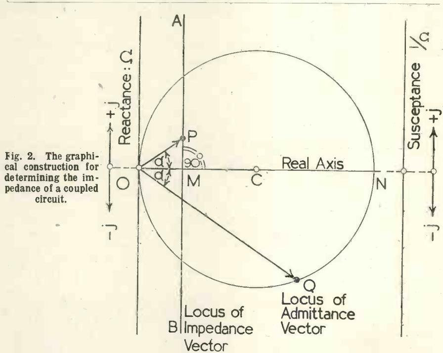
Fig. 2. The graphical construction for determining the impedance of a coupled circuit.
