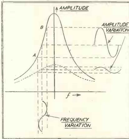
Fig. 1. Frequency Amplitude conversion of a detuned circuit.
