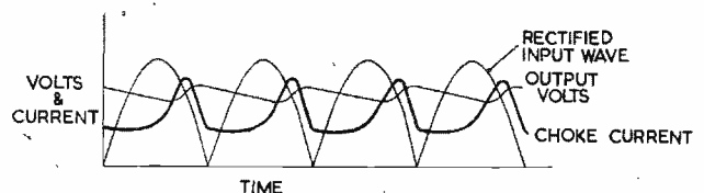
Fig. 3. Conditions of working with the input choke partially saturated
