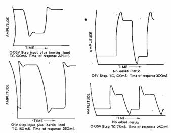
Fig. 10. Response curves of prototype (Mk II)
