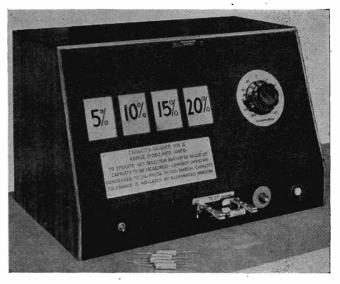
means of suitable amplifiers and switch gear the 5 per cent, 10 per cent, 15 per cent and 20 per cent tolerances are quickly measured in succession and when balance is obtained the appropriate indicator is illuminated.
