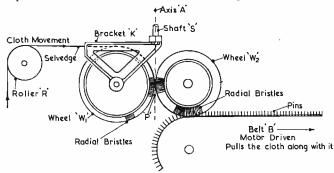
Fig. 2. Cloth guider system (side elevation)
