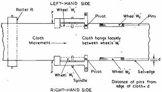
Fig. 1. Cloth guider system (p!an)
