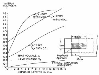
Fig. 3. Photocell sensitivity curves
