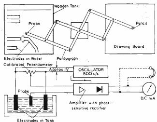
Fig. 11(a). Schematic diagram of electrolytic tank
