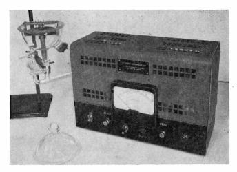
The diaphragm type micromanometer.
