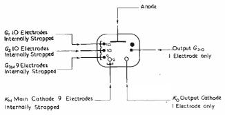
Fig. 7. Tentative signal for single pulse dekatron
