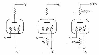
Figs. 2(a), (b) and (c). Circuits for demonstrating 2-transfers
