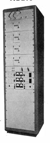
The Redifon R93 fixed frequency, high stability receiver is particularly suitable for monitoring, diversity reception or frequency shift operation. A typical application is this twinchannel, dual diversity, frequency shift radio teleprinter terminal. Multi-channel diversity or non-diversity racks can also be provided which incorporate a multi-receiver coupling unit (Redifon Type MCU.I) allowing up to eight receivers to be fed from a single aerial.
