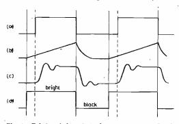
Fig. 1. Relative timing of the input square wave C.R.O. time-base, simulator response and C.R.O. blackout wave-forms
