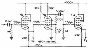
Fig. 22. " Clamp " waveform generator
