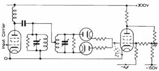
Fig. 6. Arrangement for negligible time lag
