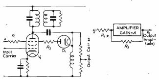
Fig. 2. Circuit for amplitude modulation Fig.
