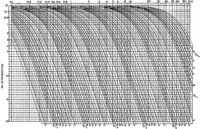
12 db/OCTAVE HIGH FREQUENCY CUT-OFF AMPLITUDE RESPONSE
