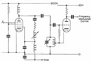
Fig. 5. The frequency modulator
