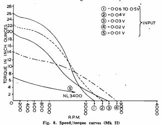
ing to maintain a sensibly constant current through the armature of the motor unit in spite of back E.M.F. To this end some hundreds of volts D.C. were fed to the armature through limiting resistors, only about one-fifth to one-quarter of the total voltage appearing across the armature when it was stationary, some 40 watts being dissipated in the dropping resistors.
