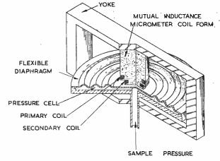
Cross-sectional view of the pressure cell.
