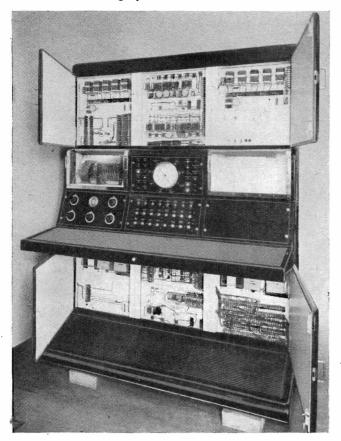
Fig. 10. Control console for a photographic zenith telescope for time determination
