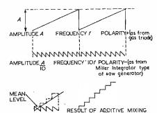
It operates as follows for ten steps: a sawtooth oscillator of amplitude A, fresawtooth oscillator of ampittude A, frequency f, and positive polarity, is used to synchronize another sawtooth oscillator of amplitude frequency 10f and negative polarity. These waveforms are A/10 applied, one to each grid of a double triode having a resistance load common to both anodes. It can be seen from the above diagram that this arithmetic mixing produces a step waveform of the required shape.
