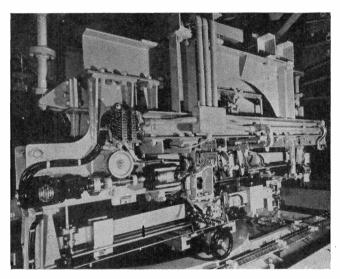
Fig. 9. Six-component wind tunnel balance
