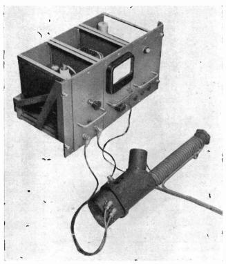
Fig. 16. A low temperature radiation pyrometer
