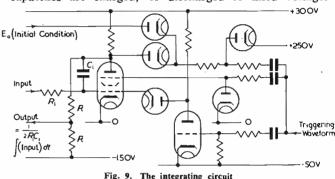
(In a subsequent circuit a resistor is connected across the suppressor grid diode)
