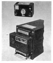
Electrical Remote Control for Transmitter/Receiver
