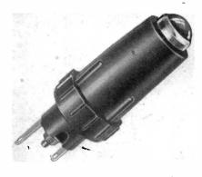
This switch, catalogue No. S.930, is rated 1 amp 250 volt, and is designed for single ½in. hole fixing. It is biased normally "on", a very small depression of the push breaking the circuit and the rest of the movement of the push being "overrun."
