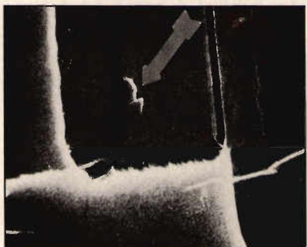
Fig. 3: SEM photomicrograph of a ruptured gate oxide.
