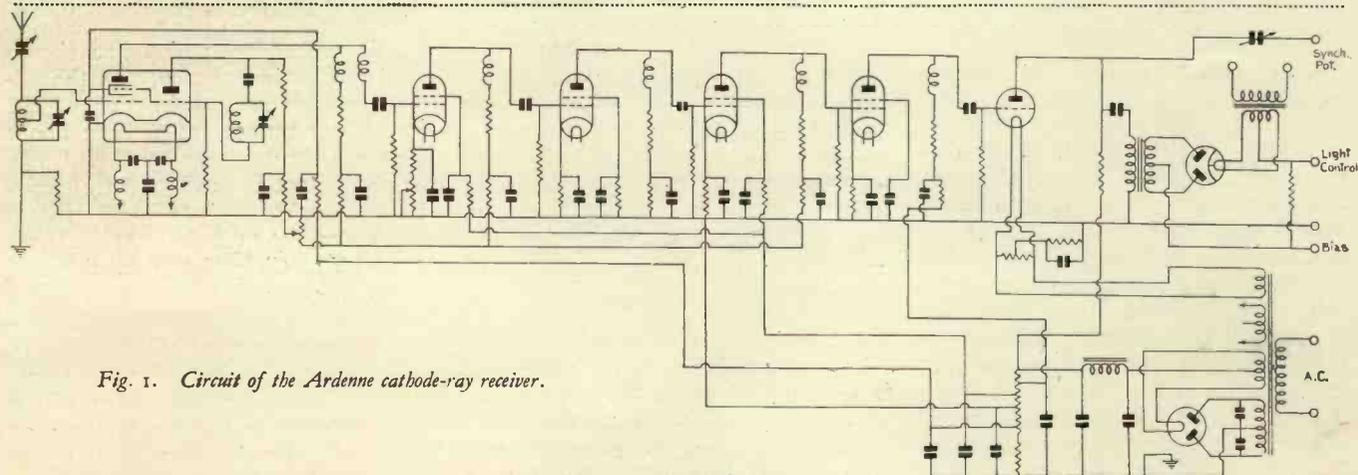
Fig. 1. Circuit of the Ardenne cathode-ray receiver.
