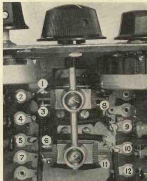
Above: Details of the wiring to the change-over switch. Note the insulated bush where the spindle passes through the chassis.
