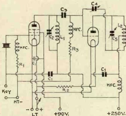
Fig. 2.—Frequency stability is assured by crystal control.
