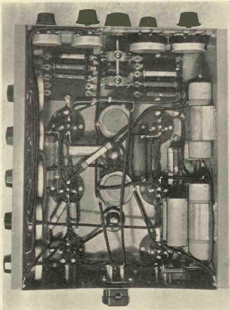
Holes 20, 21 and 22 in the lower flap of the chassis fit a two-pin mains socket (20) Bulgin Type P.20 or its equivalent; a five-pin Belling-Lee socket (21), and a four-pin valve socket (22).
