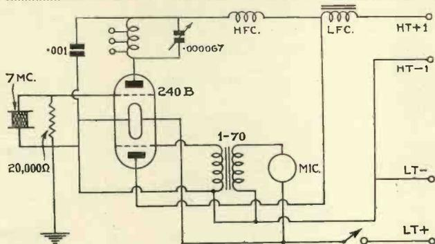
Wavelength is governed by the coil and crystal. The output is ample on 160 and 80 metres, but unless a 20-metre crystal is already on hand this band is best left alone.
