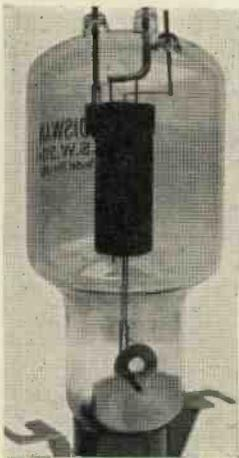
*This is the British answer to the American high-power transmitting valves. It is an Edison ESW 204 carbon-anode triode suitable for its full output of 250 watts down to 5 metres. Anode, grid and filament mid-tap contacts are brought out through the top of the bulb.*
