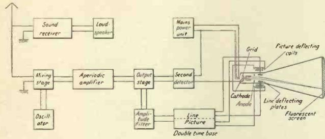
Fig. 2. Schematic diagram of receiver.
