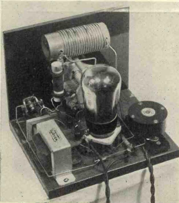
*There is plenty of room on this little baseboard so that construction is very easy. The 240B is mounted on a chassis-type valve holder, which is raised off the baseboard.*
