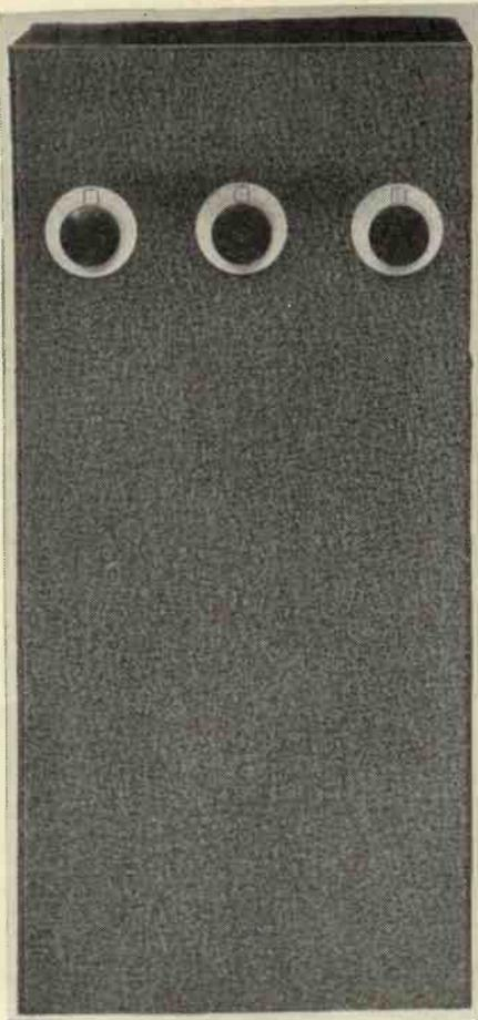
*This is just the beginning. The three controls are for the C.O. and P.A. grid and anode stages. When the transmitter is finished there will be meters in the centre with the switching circuit at the bottom.*
