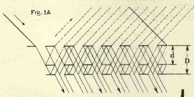
Using a piezo crystal as a light valve. Patent No. 450,686.
