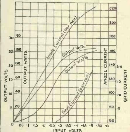
This curve gives a true idea as to the total output that can be obtained with varying input levels.
