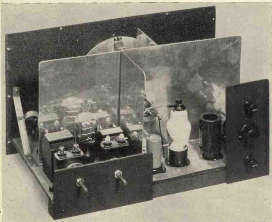
The detector voltage control should be mounted on the middle dividing screen. The resistance must be of the dead-spindle type.
