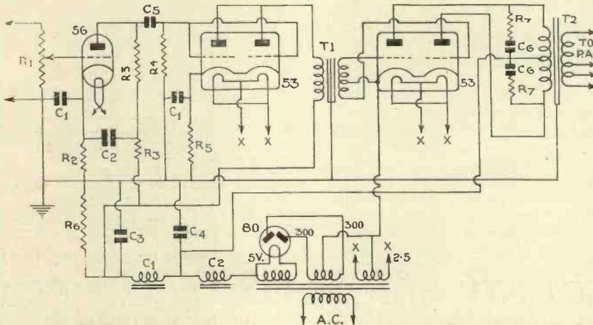
The second two valves in this amplifier are 53's twin triodes normally designed for class B operation. The first 53 has both halves wired in parallel with the second 53 used normally.
