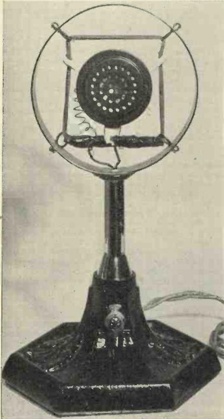
*The microphone unit is made by B.T.S., but it was fitted to this home-made stand.*
