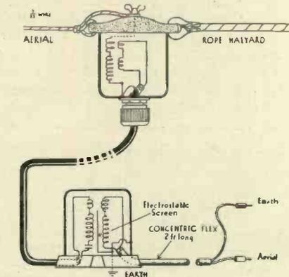
*The aerial transformer case is actually used as the insulator. It is connected to the transformer at the set end by a special low-loss cable.*
