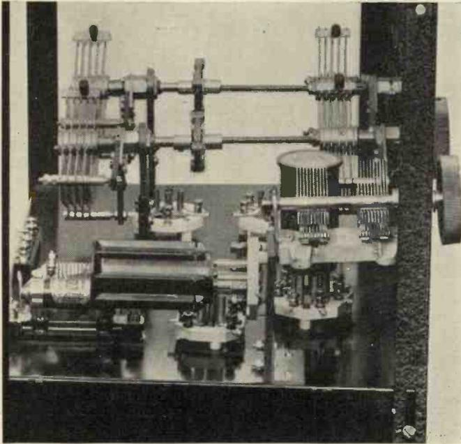
Mount the components for the crystal oscillator stage in this manner. How the P.A. stage is constructed is to be described in the December issue.
