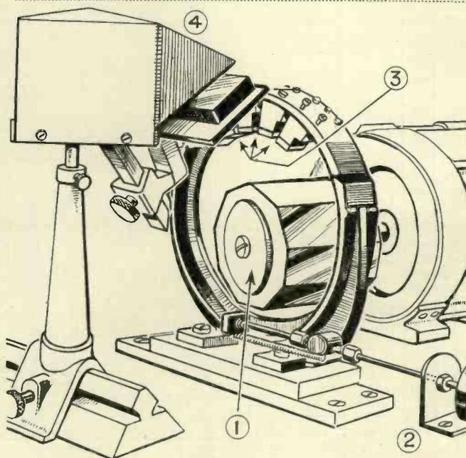
*Detailed drawing of the Mihaly-Traub scanner : the motor is on the right.*
