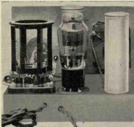
*This pentode valve has its heater connected directly across the power supply. No mains transformer is needed with this circuit.*
