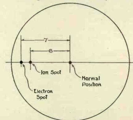
Fig. 2.—Position of the electron spot and ion spot observed with deflection by a condenser field.
