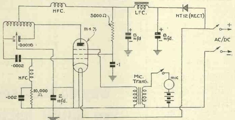
A key can be inserted in either the cathode or screen-grid circuit.
