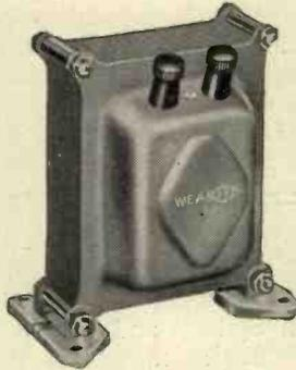
The H.T.35, like all the chokes in this series are specially layer wound — the inductance being adjusted by the air gap. Tested to 1,000 volts. Characteristics: —30 henries 50 ma., 1,600 ohms.
