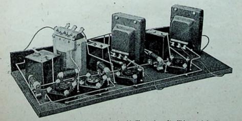
The layout of the amplifier is clearly shown by this illustration. It will be noted that large by-pass condensers are arranged across the high-tension tappings.
