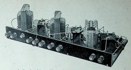
Another view of the amplifier showing more clearly the angle at which the L.F. transformers are set.
