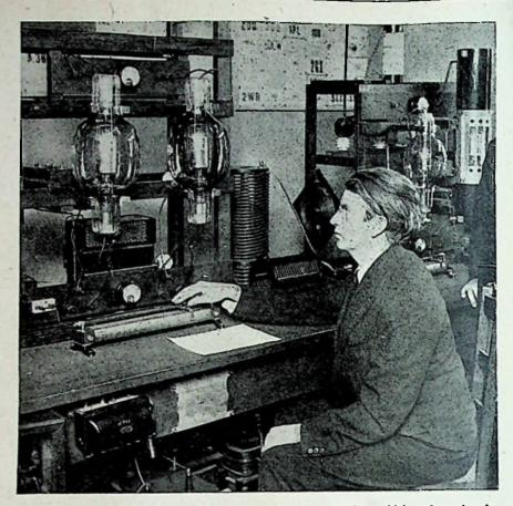
Mr. J. L. Baird seated before the 2 kw. amateur wireless transmitter which performed such yeoman service in the recent transatiantic experiments. The station is at Coulsdon, Surrey; its call sign is 2 KZ, and its wave-length is 45 metres. Television transmissions may sometimes be heard from this station after midaight.
