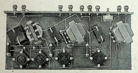
A plan aspect showing the baseboard layout. It is important to follow this closely as any modification may result in instability. Across the centre L.F. transformer is connected the 100,000 ohm resistance.
