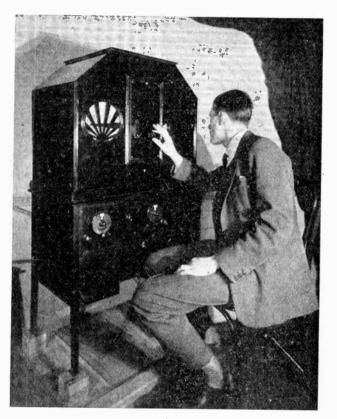
Receiving a Television transmission on a Baird Dual Exhibition Receiver. The apparatus shown contains two wireless receiving sets, one for speech and one for vision. The "televisor" is fitted with a Baird automatic synchronising apparatus.
