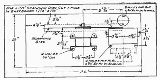
Fig. 1.—Detailed dimensions for the baseboard layout.
