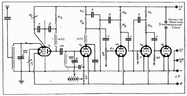
Fig. 1.—A wireless circuit for receiving Television.
