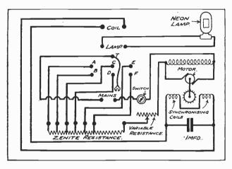
Fig. 2.—The complete circuit for wiring up the Baird kit of components.
