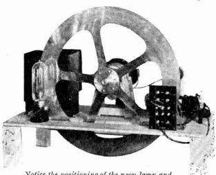
Notice the positioning of the neon lamp and terminal board.
