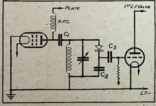
Fig. 4.—Showing how the crystal was connected up when receiving television images.
