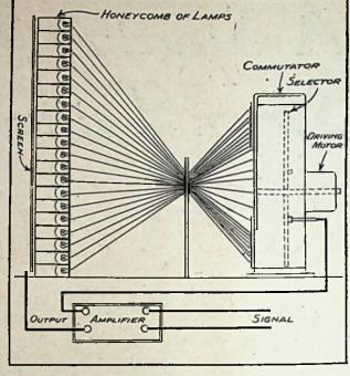
A rough schematic diagram of the wiring between commutator and screen.
