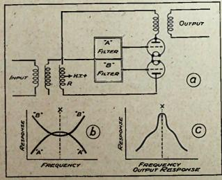
Fig. 2.—A suggested filter circuit together with the frequency responses of the filters.
