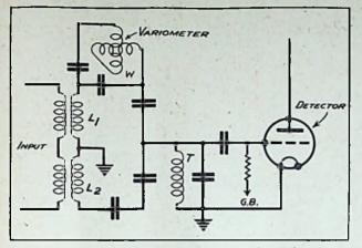
Fig. 3.—Circuits can be designed for neutralising and accepting the unwanted and wanted frequencies respectively.
