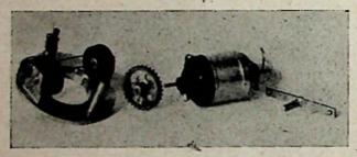
Parts of the Baird synchronising mechanism shown dismantled from the motor.
