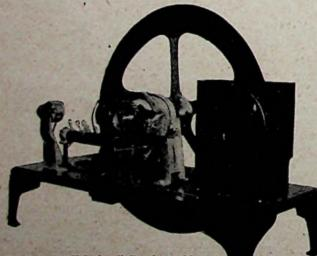
The Baird "Televisor" Receiver with cover removed showing all the internal mechanism. Try and win it. occurs. During these pauses an object, action or person representing the missing word will be televised.
