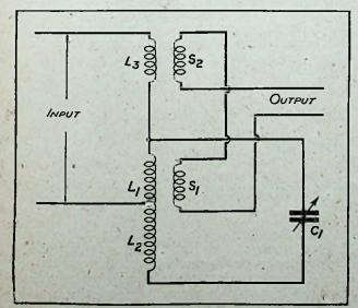
Fig. 4.—Here the oscillatory circuit acts both as a tuning circuit and as a wavetrap.
