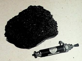
A sample of a modern crystal detector with a large carborundum crystal in the background.
