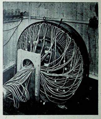
The intricate nature of the selector and commutator mechanism and wiring are revealed in this photograph.
