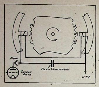
Fig. 2.—Showing how the cogged wheel synchronising mechanism may be connected in series with the neon and output valve.
