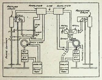
The schematic diagram of the Siemens-Karolus-Telefunken picture transmission system.
