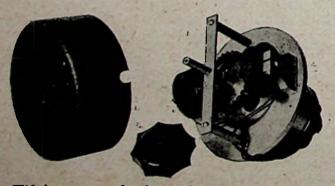
With the cover removed we here see the magnetic toothed wheel . synchroniser.
