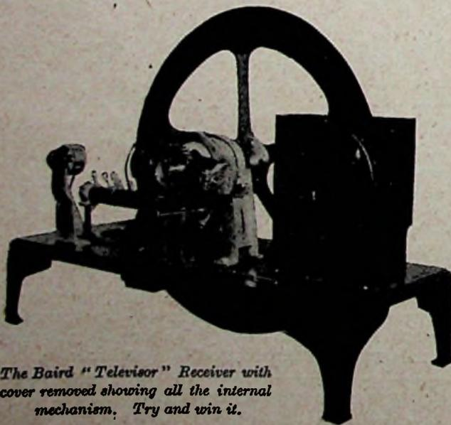
*The Baird "Televisor" Receiver with cover removed showing all the internal mechanism. Try and win it.*
