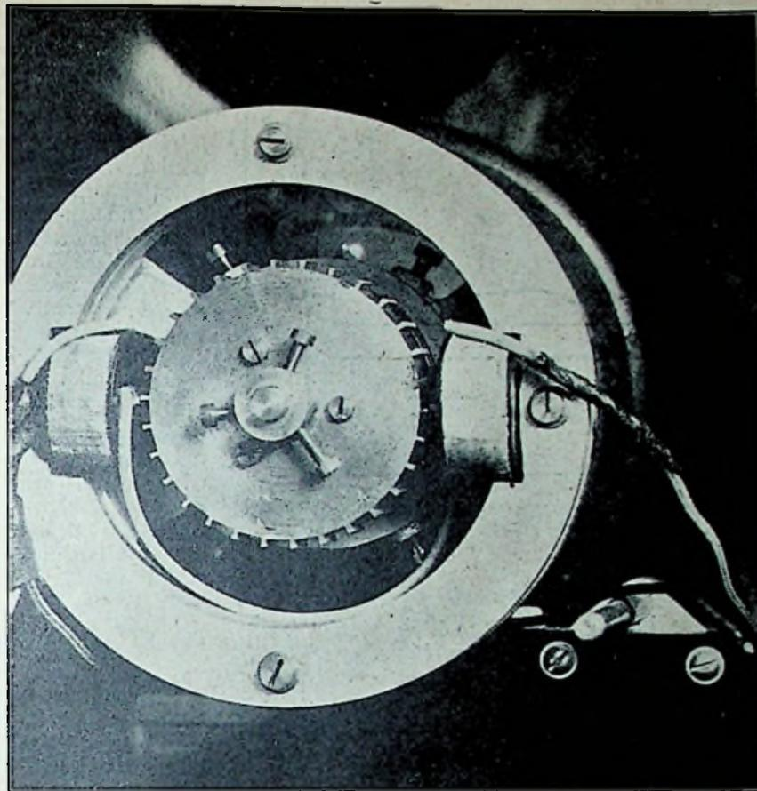
*One of the first models of the cog-wheel mechanism. Note how this has been improved upon in the commercial "Televisor."*
