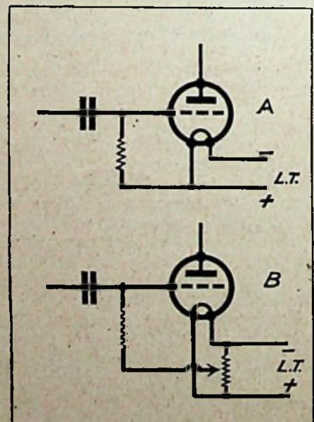
this method lies in the fact that by properly adjusting both grid bias and high tension voltages, very strong input signals can be handled without any trace of distortion. Note that the high frequency impulses are amplified in the valve itself before undergoing rectification in the anode or plate circuit, so that the scheme is entirely different from that of the previous method.
