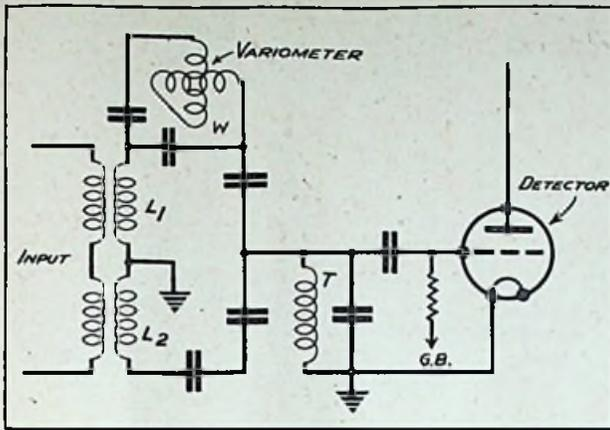
Fig. 3.—Circuits can be designed for neutralising and accepting the unwanted and wanted frequencies respectively.
