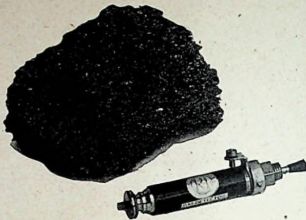
A sample of a modern crystal detector with a large carborundum crystal in the background.
