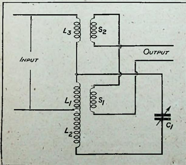
Fig. 4.—Here the oscillatory circuit acts both as a tuning circuit and as a wavetrap.
