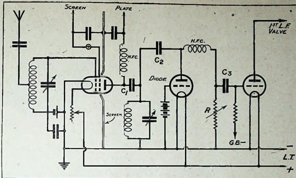
Fig. 3.—Details of the diode detector circuit which have given such good results.
