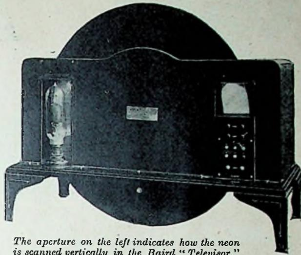
The aperture on the left indicates how the neon is scanned vertically in the Baird "Televisionor."
