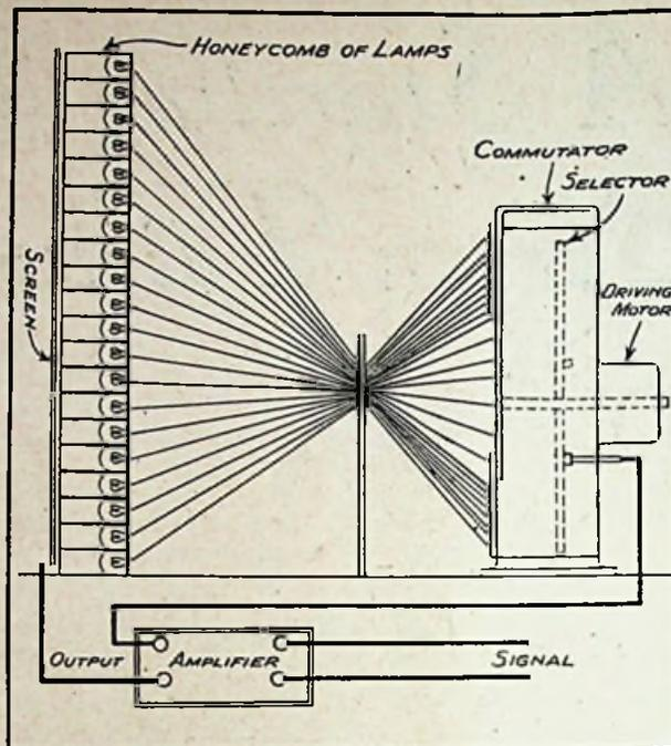
*A rough schematic diagram of the wiring between commutator and screen.*
