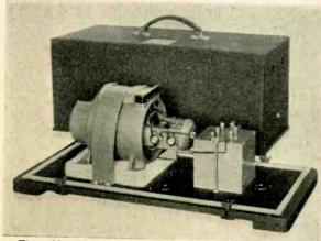
The " M.-L." rotary transformer with anti-interference unit.
