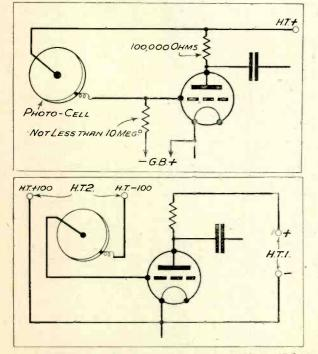
(Above) Method of coupling cell to first stage amplifier. (Below) An alternative method, which is more sensitive but requires two H.T. batteries; no grid leak is used.
