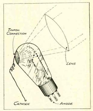
Diagram showing the light being directed from the lens to the valve.
