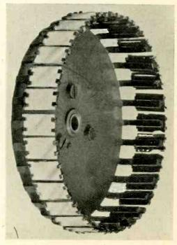
The completed drum with mirrors in position.
