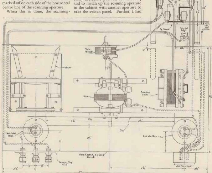
A plan view of the disc receiver showing the wiring. TA large-scale blueprint is available, price 1/-
