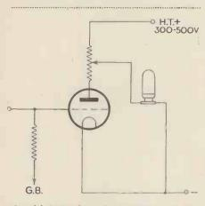
A useful circuit where voltage is limited; the value of the resistor should be equal to the optimum load of the value, the amount of modulation being con-trolled by moving the slider.
