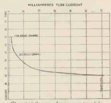
Characteristic curve of mercury-vapour tube.
