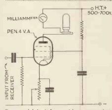
Recommended circuit for use with a mercury-vapour lamp, the current is controlled by means of the bias resistor.
