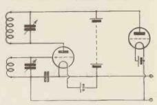
Fig. 6. "Ticking-grid" time-base circuit, developed by Appleton, Watson-Watt and Herd, using a valve oscillator
