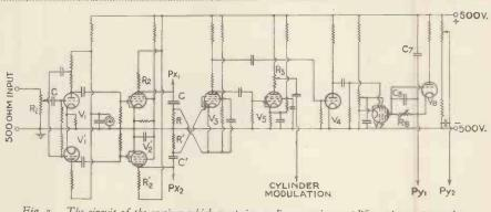
Fig. 2. The circuit of the receiver which comprises a line-scanning amplifier, picture-traversing time-base and an intensifying system.
