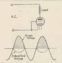
Fig. 5 Diagram showing the formation of uni-directional pulses when A.C. is applied to a resistance loaded gas-filled relay.
