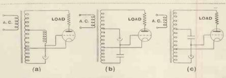
Fig. 9. Three arrangements showing how the gas-filled relay is adapted to be worked from a photo-cell
