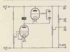
Fig. 4. Simple time base adapted for use with mains values. The letters refer to the plates of the oscillograph
