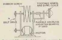
A suggested layout for driving a mirror screw by step-down belt gearing.
