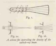
whilst a positively-charged ring is the equivalent of a concave lens. This enables a reduced or enlarged image of the spot to be produced on the fluorescent screen as desired. A combination of ring and disc may be used to produce a sharper focal effect.—(Siemens-Shuckertwerke Akt.)
