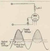
Fig. 6 Showing the effect of biasing the grid of the gas-filled relay.
