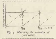
commences to charge up. It takes a certain fraction of time to do this because of the relatively high resistance introduced into the circuit by the valve, but ultimately it builds up to a voltage somewhere approaching the full value.
