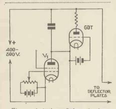
Fig. 1. A simple gas-discharge time base.
