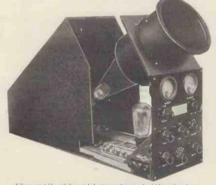
Ediswan portable cathode-ray tube 'equipment shown partly withdrawn from its case. Underneath the tube can be seen the thyratron for the time-base. On the jront panel are the controls for the time-base and for the focusing tube
