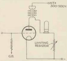
Transformer-coupled arrangement of mercury lamp where H.T. voltage is limited. The resistor is essential for current limitation.
