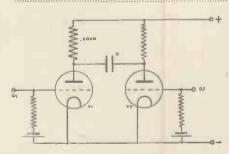
How the function of the switch can be Fig. 11. performed by a second relay.
