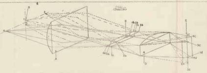
Fig. 4. Diagram showing the action of two cylindrical lenses
