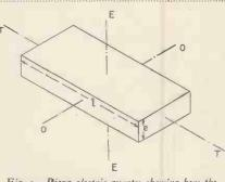
Fig. 5. Piezo-electric quartz showing how the application of an electric field brings about a strain.
