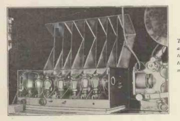
time-base sweep to be uniform, and the arrangement adopted is that of allowing the scanning lines to be moved on in a step-wise manner between consecutive lines, the magnitude of the step being fixed and independent of the time taken by the lines.
