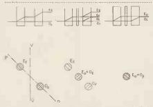
Fig. 1. A diagram explaining the action of the double-image polariscope.
