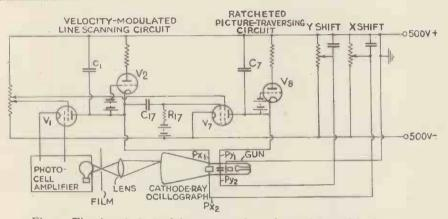
Fig. 1. The schematic circuit of the transmitter for producing velocity-modulated scanning.
