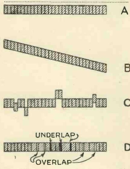
Fig. 5. — These diagrams show the defects due to bad angular, lateral and radial spacing of the scanning arrangements.
