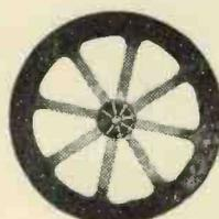
**E**ACH disc is of light gauge aluminium, dull black one side, and centres cut out to reduce weight. The centre boss is an 8-ribbed black bakelite moulding. Each rib being faced white to give true stroboscopic effect, and thereby visual speed indication. A heavy brass bush insert with grub screw provide simple and accurate fixing for  $\frac{1}{2}$ " motor spindles. Scanning holes perfectly punched to secure uniform scanning without preventable lines. **7/6**
