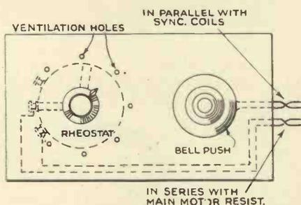
Fig. 2.—Details of a motor control panel.
