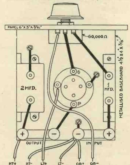
Fig. 4. Details of a simple single stage amplifier for supplying current to the synchronising coils.
