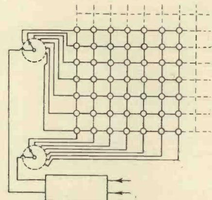
Fig. 2.—A double commutator system designed with the object of reducing the number of commutator segments.
