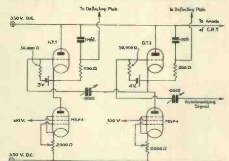
Fig. 17.—Scanning circuit employing gas-filled relays for 180 lines and 25 pictures per second.
