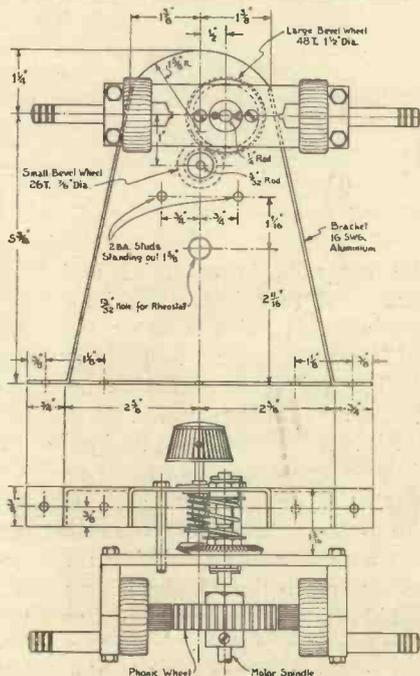
Fig. 2. Detailed drawings showing the gear fitted with reduction wheels.
