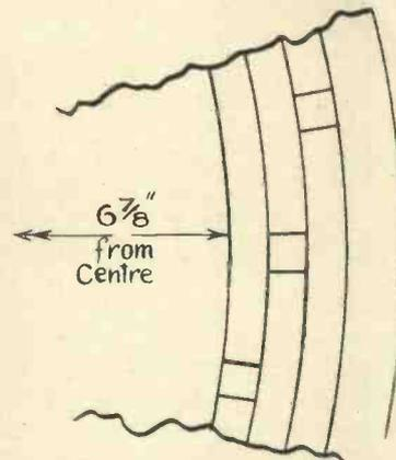
*Diagram showing the radial positions of the holes.*
