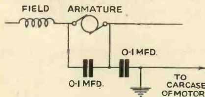
Fig. 4.—Tbis arrangement can be recommended for a motor of the universal type operated from A.C. mains.
