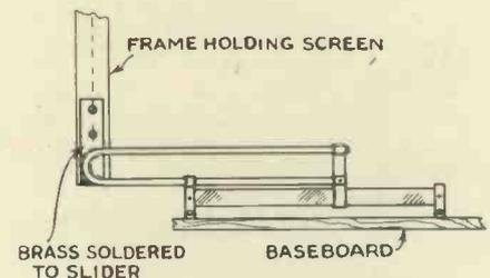
Fig. 3.—A cheap improvised focusing arrangement.
