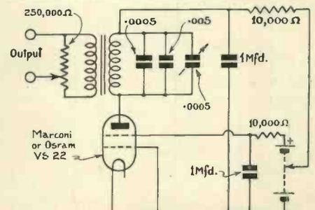
Fig. 2.—The circuit diagram of the dynatron low-frequency oscillator described in the text.
