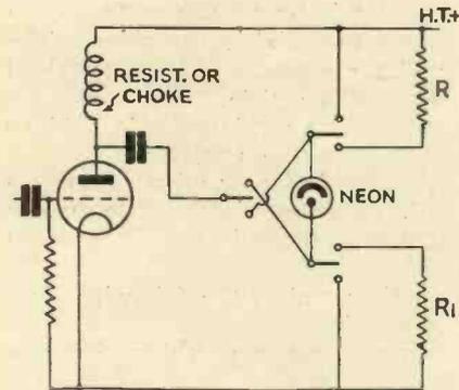
Fig. 3.—A circuit suitable for use with a neon lamp. This also allows for reversal of the image from negative to positive or vice versa.
