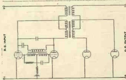
Fig. 16.—A circuit of a high-efficiency D.C. transformer.
