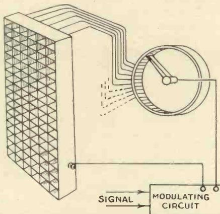
Fig. 1.—Schematic diagram showing the system of using a number of light units to build up the picture.
