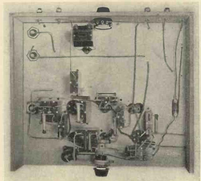
*Except for a part of the tuning circuits, most of the wiring is connected underneath the chassis*
