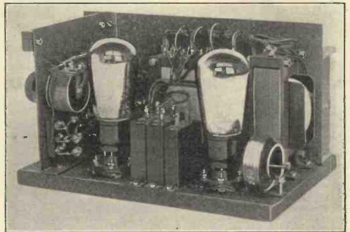
Fig. 14.—An inverter of the self-excited type employing a pair of gas-filled relays.
