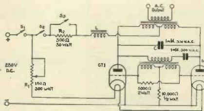
Fig. 15.—The theoretical circuit of the inverter shown by the photograph.
