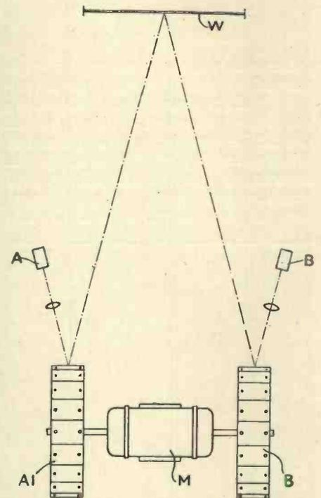
A method of employing two light sources for projection on to one screen in order to increase the lighting intensity. Patent No. 408596.
