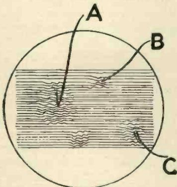
The fringing effect on a cathode-ray tube screen. Patent No. 408297.
