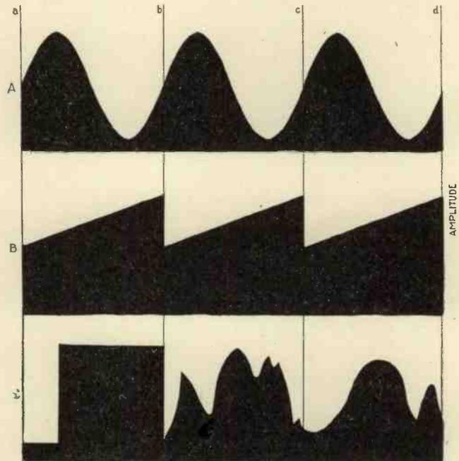
Fig. 2. Three drawings of recorded wave form. A shows three cycles of a sine wave, B three cycles of a saw tooth wave, and C a square topped and two irregular wave forms.
