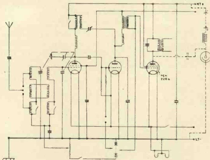
*Fig. 1. — The Halcyon three-valve battery set with pentode output. With a large pentode the output is sufficient to modulate the neon.*
