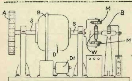
A method of synchronising employing a separate motor to revolve the carcass of the main driving motor. Patent No. 408332.
