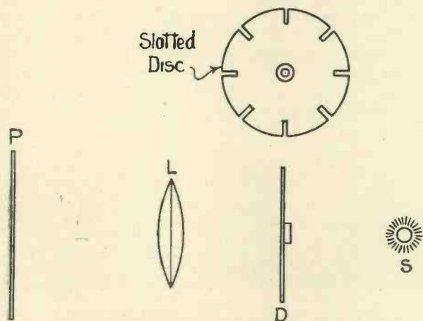
Fig. 3. A schematic diagram showing the layout of the light chopper.
