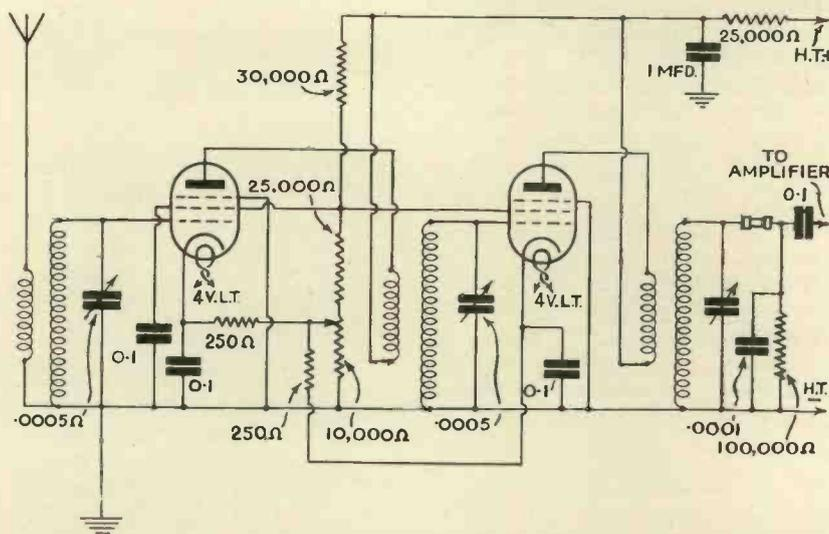
Circuit diagram of the receiver. Two variable-mu H.F. pentode stages are used followed by diode detection.
