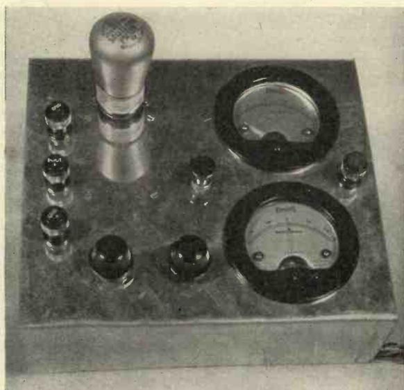
*The valve voltmeter ready for use.*
