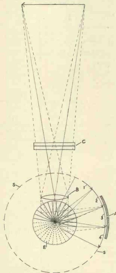
Fig. 33. Reflecting angularly displaced rotating echelon for television.
