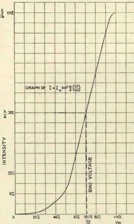
A voltage-intensity graph of a Kerr cell.
