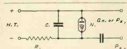
Fig. 4.—A simple time base circuit using a neon lamp.
