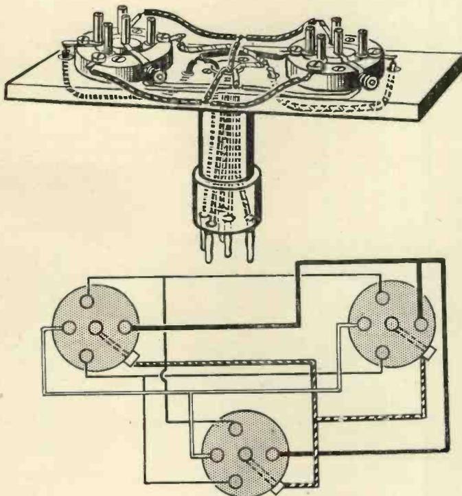
Fig. 3 (left) A useful gadget for use with battery sets; the output can be doubled without altering the receiver.
