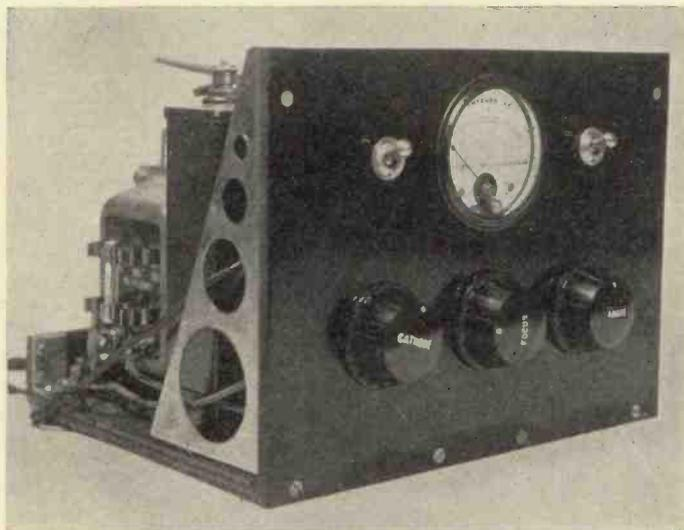
A view of the completed supply unit for the cathode-ray tube.
