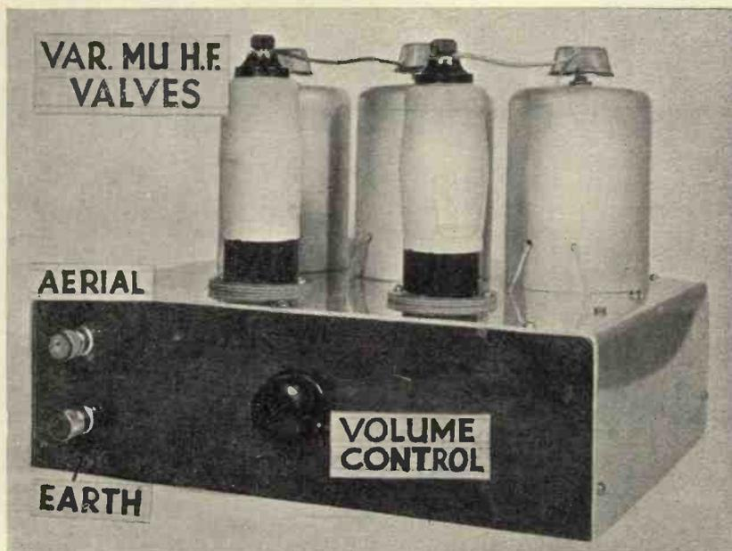
Only the valves and coils are on the upper part of the chassis : all the wiring is below.
