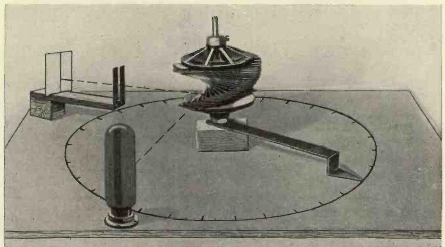
Fig. 2. Accuracy in the setting of the mirrors can best be obtained with a similar arrangement to that shown by the photograph: the long pointer and distance the light beam has to travel ensure that only very small errors can occur.
