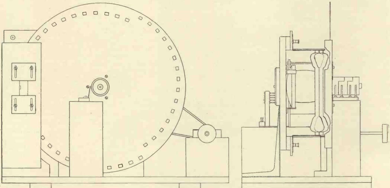
These drawings are side and end elevations of the Baird colour television receiver.
