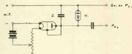
Fig. 5.—A time base incorporating a saturated diode to provide a more linear effect.
