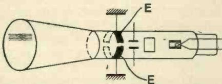
A special construction of cathode-ray tubes to prevent distortion effects in the picture due to movements of the ions formed between the screen and the deflecting electrodes. Patent No. 408297.
