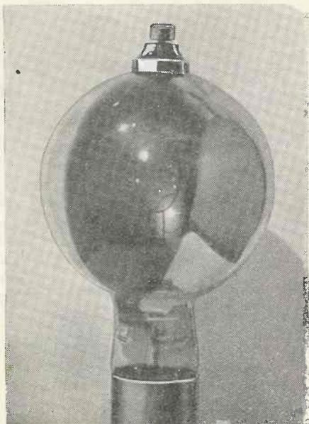
An Oxford photo-cell specially designed for television.
