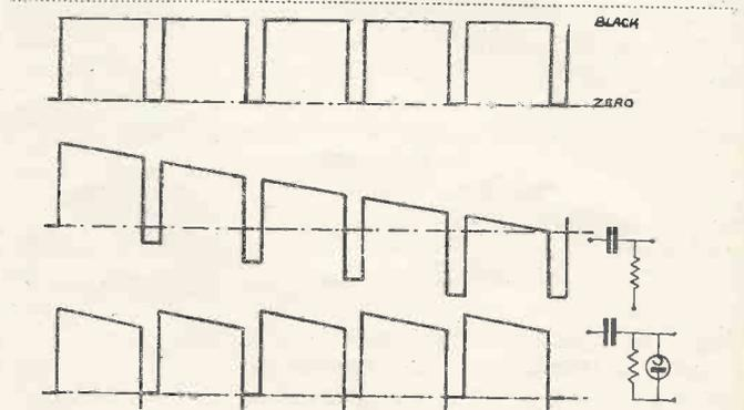
Fig. 2. A series of "black" impulses showing how the condenser potential varies without the D.C. restoration.
