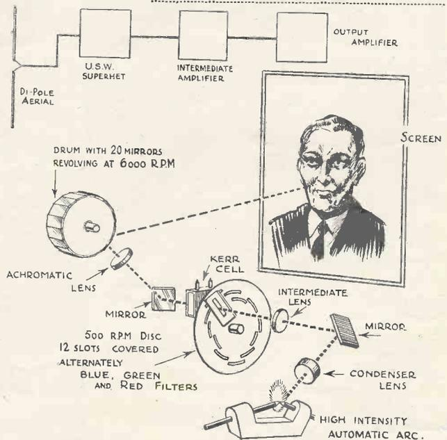
Schematic drawing of the receiver.
