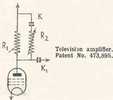
dance of the anode circuit, and therefore the effective "gain" of the valve, can now be changed by varying the parallel resistance  $R_2$ , though this does not affect the D.C. voltage applied through the resistance  $R$  from the H.F. supply to the plate. The output is taken off either directly or through a condenser  $K_1$ .—*Baird Television, Ltd., and L. C. Bentley.*
