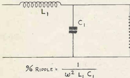
Fig. 1. Calculating ripple value.
