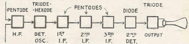
Schematic diagram showing the stages in a vision receiver.
