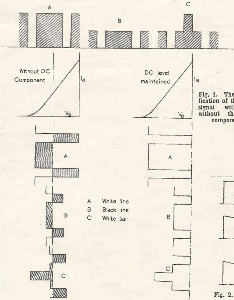
Fig. 1. The amplification of the video signal with and without the D.C. component.
