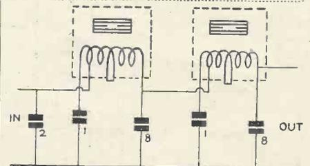
Fig. 3. The hum-bucking circuit.
