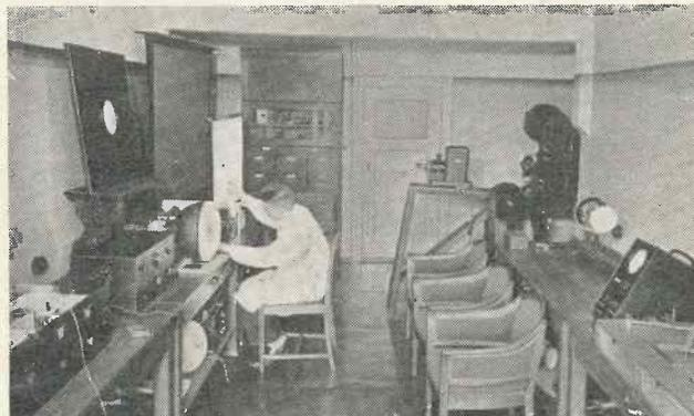
**Television laboratory.** The receiving set for 441 lines can be seen on the left, while in the foreground is an electrolytic trough for plotting field lines. At the back is a film scanner and apparatus for investigating stereoscopic projection.
