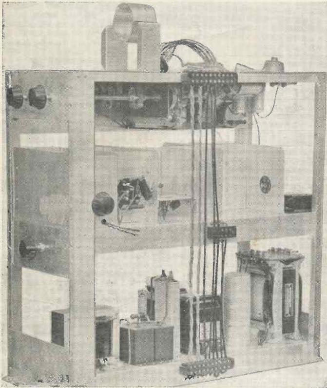
A general view of the complete vision receiver. Chassis construction is of sheet aluminium or steel and is of the simplest type.
