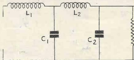
$$\% \text{ RIPPLE} = \frac{1}{\omega^4 L_1 L_2 C_1 C_2}$$
