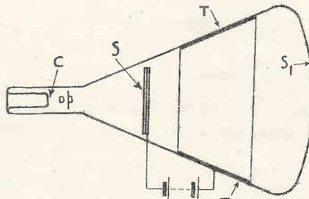
Cathode-ray tube construction for increasing picture size. Patent No. 474,391.
