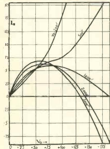
Fig. 6. Grid-volts-grid-current curves of the Tungram 0-300/3,000 showing the effect of secondary emission from the grid.
