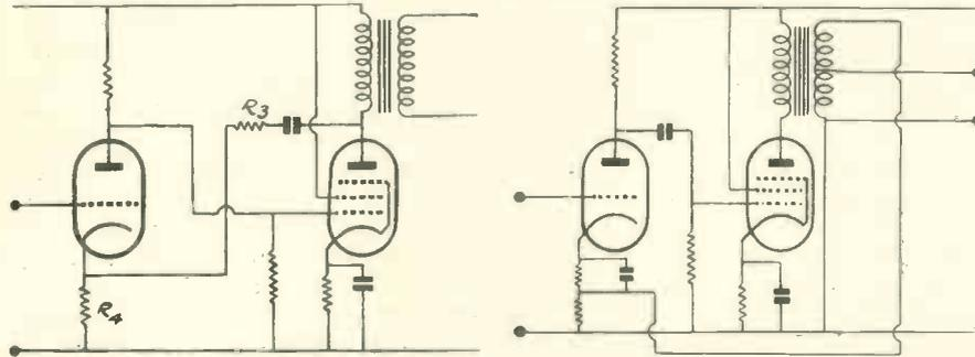
Fig. 3. Two methods of feeding back into a preceding stage. (3b corresponds to b of Fig. 2. and 3c to c of Fig. 2.)
