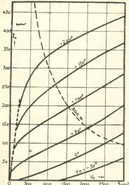
Fig. 5. Anode-volts-anode-current curves of the Tungram 0-300/3,000.
