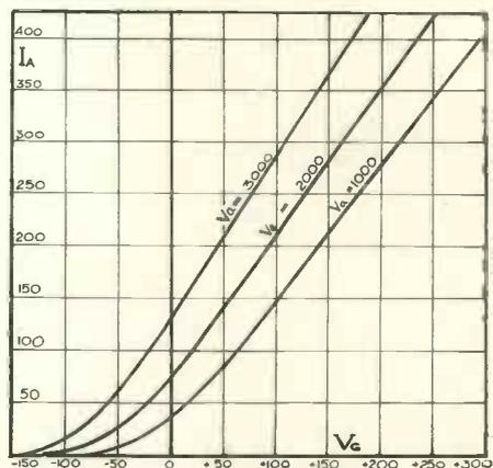
Fig. 4. Grid-volts-anode-current curve of the Tungram 0-300/3,000 U.S.W. transmitting triode extending above the dissipation limit.
