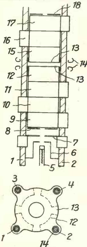
Fig. 1. Electrode supporting system of high-voltage cathode-ray tube shown in elevation and plan.
