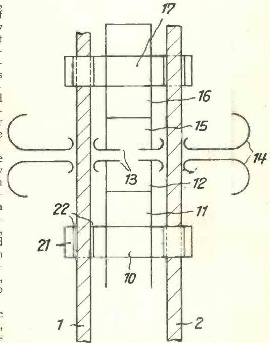
Fig. 2. Diagram showing how the cylinder is assembled in two parts.
