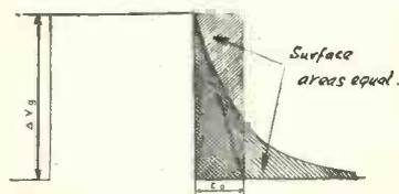
Fig. 15. Grid voltage waveform due to the action of the grid shunt condenser included in circuit Fig. 1 in order to eliminate transient oscillations.
