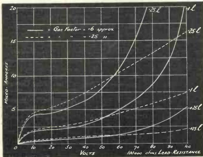
The effect of gas pressure upon the current-voltage curve at various light fluxes.
