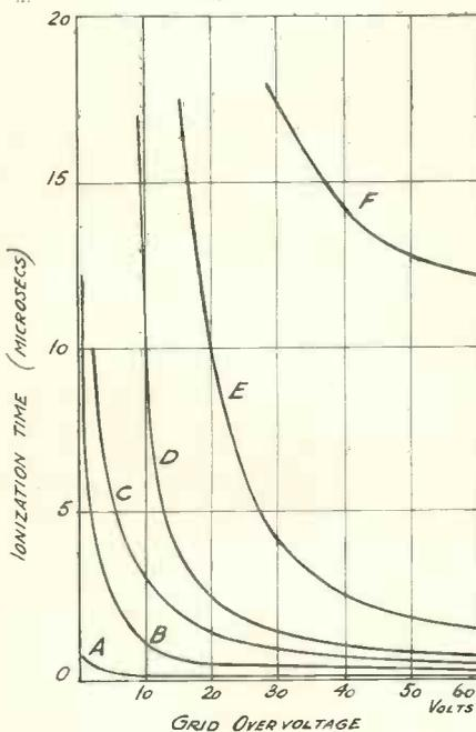
Fig. 2. Curves showing relationship between time of ionisation and grid overvoltage.
