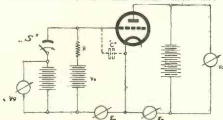
Fig. 1. Schematic diagram of measuring circuit. S is the rotary switch shown in Fig. 2. C is included to stop transient oscillations.
