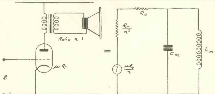
Fig. 4. Equivalent circuit of output valve and loudspeaker at low frequencies.
