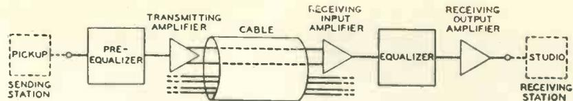
Fig. 2. Block diagram showing arrangement of equalisers.
