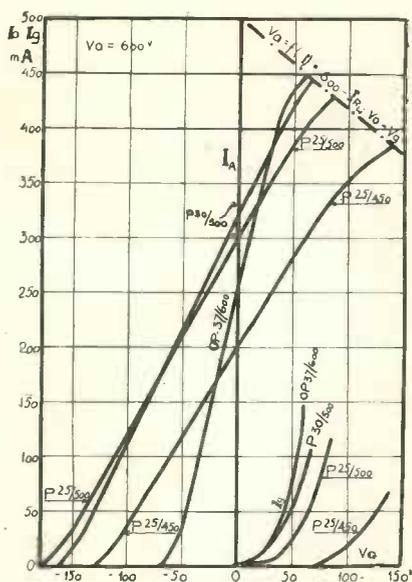
Fig. 12. Grid-volts-anode and grid current curves of several Tungram types of the 25-37 watts category, taken with the smallest permissible anode load.  $R_L = 1,200$  ohms.
