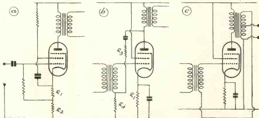
Fig. 2. Three methods of introducing feedback into the output stage.
