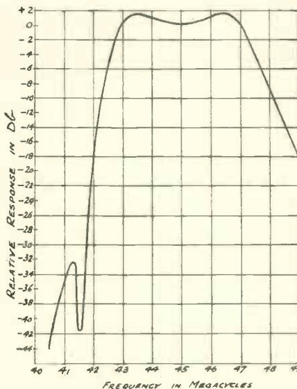
Fig. 6. Overall response curve of a television receiver showing the attenuation of the sound signal by using one of the circuits of Fig. 5.
