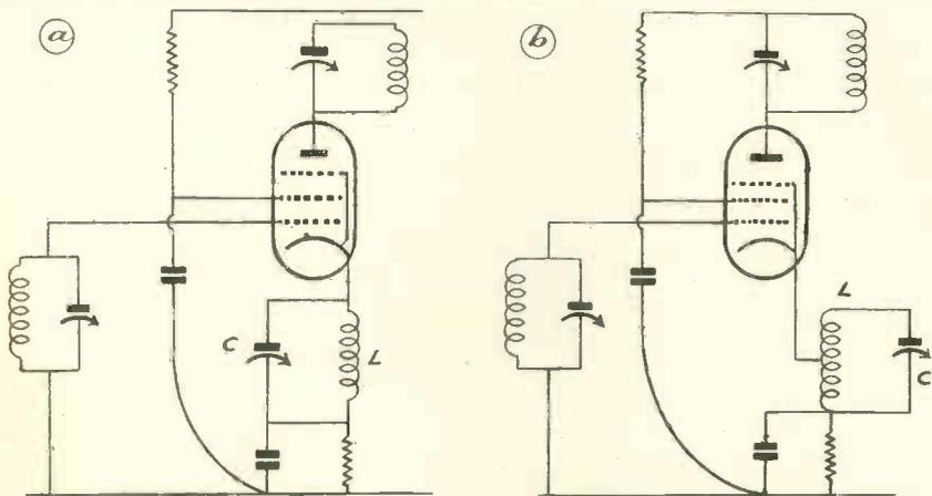
Fig. 5. The application of negative feedback to r.f. amplifiers, with cathode tuned circuit.
