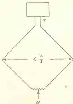
Fig. 2. Rectangular arrangement of loop antenna.
