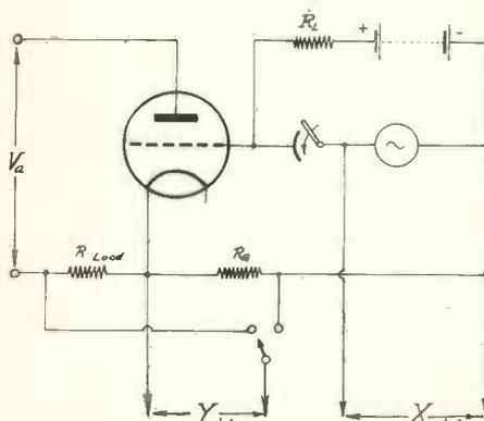
Fig. 13. Circuit for oscillographic observation of characteristics.
