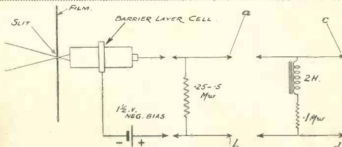
Fig. 2. Diagram showing how the cell is used with sub-standard film. a b and c d are points for amplifier connection.
