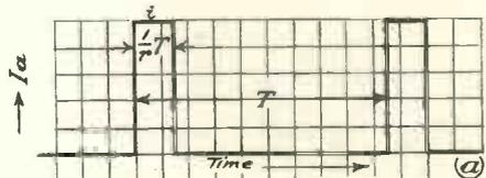
Fig. 3a. Ideal anode current waveform.
