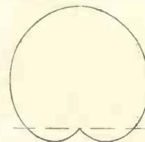
Fig. 4. Directional diagram of cardioid form.
