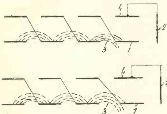
Figs. 2 and 3. Detuned and tuned conditions respectively in secondary-emission valve.
