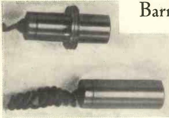
This photograph shows the S5 and S5X barrier-layer photo-cells a little larger than actual size.
