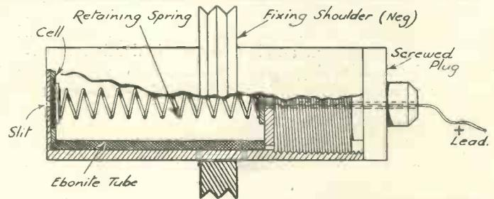
This barrier-layer selenium cell has a sensitive area of only 5 by 1 mm. arranged as a slit on the metal housing; it has a frequency response equivalent to the average wireless set, in other words, tolerable quality sufficiently good for the average listener.
