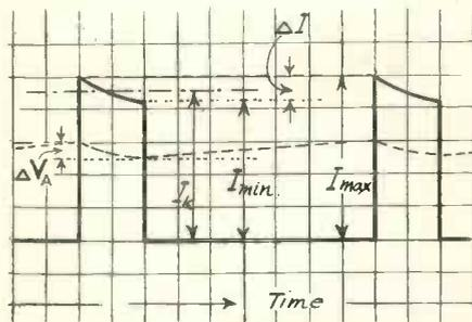
Fig. 14. Anode current waveform as a function of time.
