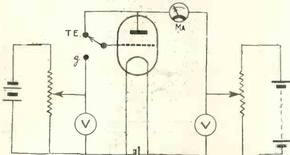
Fig. 2. Typical circuit for measuring static characteristics. The switch in the grid circuit enables measurements of total emission from the cathode to be obtained.
