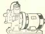
A 500-watt, single cyl. 2-stroke, water cooled, self-oiling Stuart Turner engine; mag. ign., coupled to 50/70 volts, 10 amps., shunt dynamo, 1,000 r.p.m. £16.
