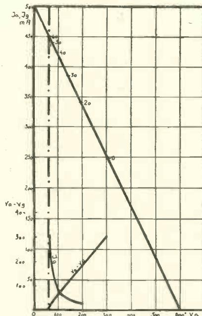
Fig. 10. Anode-voltage-grid and anode-current curve limits showing smallest permissible anode-load line of Tungram type OP-37/600.
