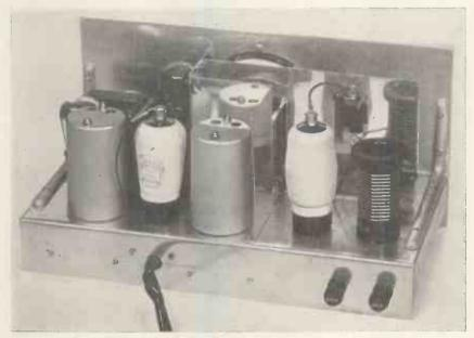
The triode-pentode value can be seen on the right-hand side next to the aerial coil.
