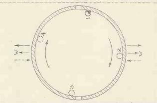
Fig 3.—An anology of the method of operation of the split-anode magnetron.
