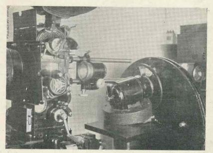
TeKaDe transmitter for interlaced scanning.
