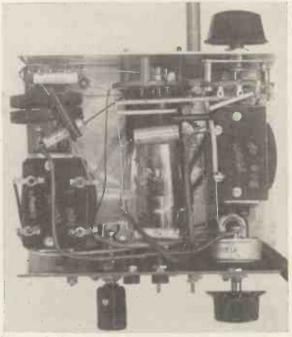
Fig. 4.-Some idea as to the layout can be seen from this view. The pentode modulator is in the centre of the chassis.
