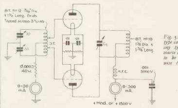
Fig. 3. A circuit of this type can be adapted to use any type of value. Of course the anode voltage has to be re-adjusted, otherwise the circuit remains unchanged.
