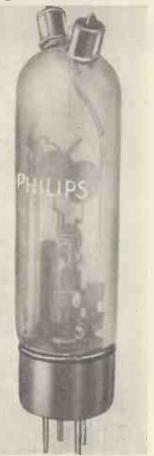
very highest frequencies Fig. 4.-The Philips Magnetron valve.
