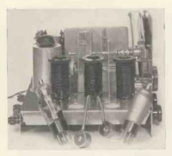
an X41 triode-hexode used as a detector-oscillator. This valve permits of level oscillation down to well under ten metres with a very high conversion conductance. The triode sec-
