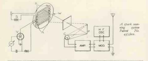
picture P, and the reflected light is received by a photo-electric cell C and is used to modulate the outgoing carrier-wave in the usual way. At the receiving end, the brilliancy of the spark-discharge on a similar viewingscreen is constantly varied by the incoming signal voltage, and so reproduces the light-and-shade effects of the original picture.—(Communication Patents Inc.)
