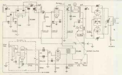
Fig. 4. The ten-metre band has proved its use this year. Here is a straightforward circuit that can be adapted for English values.
