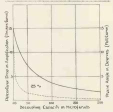
Fig. 5.-Showing effect with second method of decoupling for same value as in Fig. 3.  $R\nu = 10,000, R_1 = 20,000, R_3 = 100,000,$  $\mu = 30, R_2 = 1,000.$
