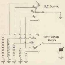
Fig. 6.-Coils of higher inductance than the one in use are short-circuited by an additional switch.
