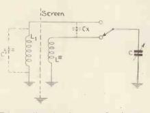
Fig. 3.—Absorption due to coupling by stray capacity.
