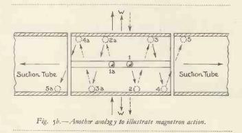
will be obvious. In a mechanical working model to illustrate the magnetron action, the trough-cylinder could be slightly tilted in the plane of vibration (Fig. 5a) in order to throw the used marbles clear, whilst the new marbles were fed in at the centre of the slots (analogy with tilted magnetic field) or a blast of air or suction device be directed along the axis of the cylinder (analogy with "end-plates") (Fig. 5b).
