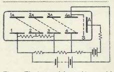
Fig. 3.—The circuit used for supplying potential to the electron multiplier. The initial stage resistances can be inserted in the bulb.
