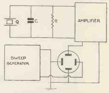
A simple circuit for using the tube as an engine indicator.
