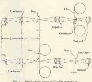
Fig. 1.—Simple optical layout of disc film transmitter.
