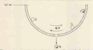
Fig 2.—A mechanical anology of the Barkhausen-Kurz mode of operation.
