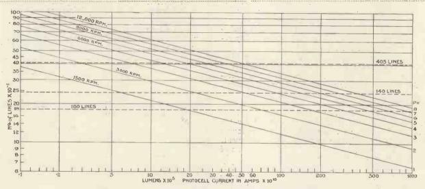
Fig. 2.-Graph showing the efficiency of the apertured disc film transmitter.
