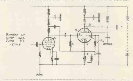
A.C. components are concerned, through a condenser C. The cathode F. is connected to the mid-point of two equal resistances R,  $R_1$  in order
