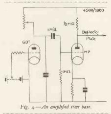
tubes to some point of fixed potential. Care must be taken to avoid high voltage between heater and cathode.
