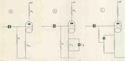
Fig. 1.—Automatic grid bias is derived from the voltage drop across R<sub>2</sub>, but amplification is resistance, both of which, with proper choice of condensers, avoid any loss of amplification.
