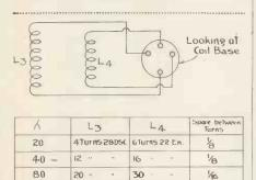
Only the 160-metre oscillator coil is close wound. The remainder of the coils are spaced as indicated.
