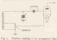
Fig. 2. Electron coupling is an arrangement that should be more widely used. This is a particularly good circuit.
