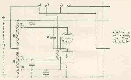
one pair 1, 2 of the deflectingelectrodes in a cathode-ray receiver. A similar circuit is, of course, necessary for supplying the second pair of electrodes marked 3, 4.
