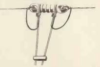
Fig. 7.- This is the way the feeders should be connected to the insulator in the centre.
