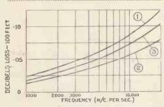
Fig. for 12-gauge copper wire at 600 ohms. for 1-in. copper tube at 300 ohms. and (3) 1-in. ohms. aluminium tube at 300 ohms.
