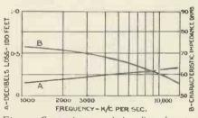
Fig. 5 .--Concentric transmission line characteristics. Velocity is equal to 86.1 per cent. of free space between 2 and 10 M.C.
