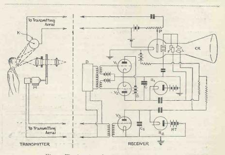
Fig: 2.-Time-base circuit for new method of interlaced scanning.
