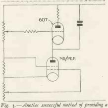
Fig. 3.—Another successful method of providing c continuous variation of sweep.
