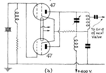
Fig. 3a.—The original crystal stage.
