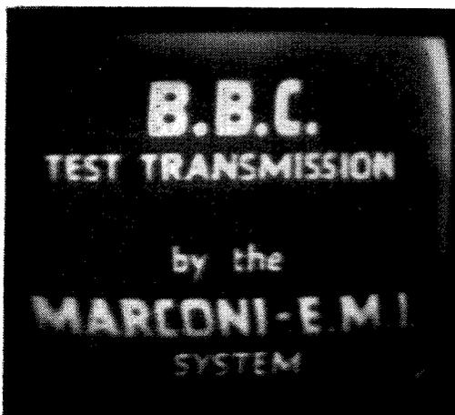
*Left: The tube biased to about correct brightness for ordinary viewing. Again note slight cut off in brilliancy of the I in E.M.I. Another effect is also noticeable, namely, the white edge on right of picture; this white edge appears to be present in varying degree in all M.-E.M.I. pictures.*
