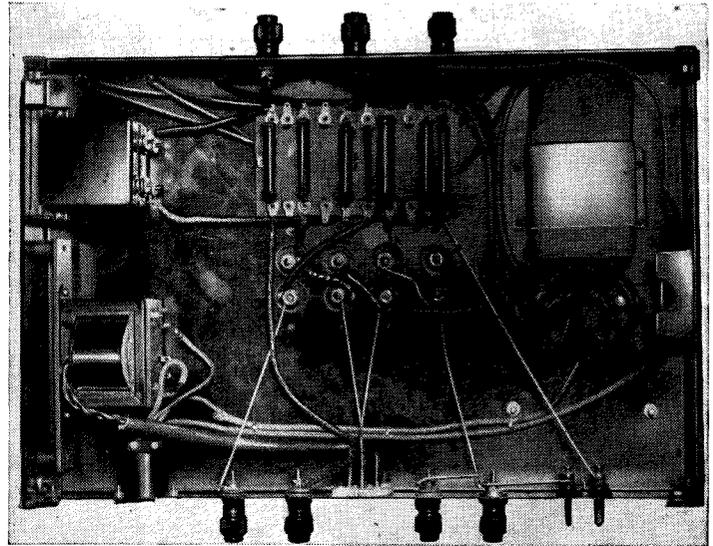
Photograph of underside of base showing wiring and positions of components
