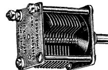
The Tank condenser unit has a capacity range of 10 x 14 m.mfd., achieved by a patented step by step device. Complete with scale and knob.
