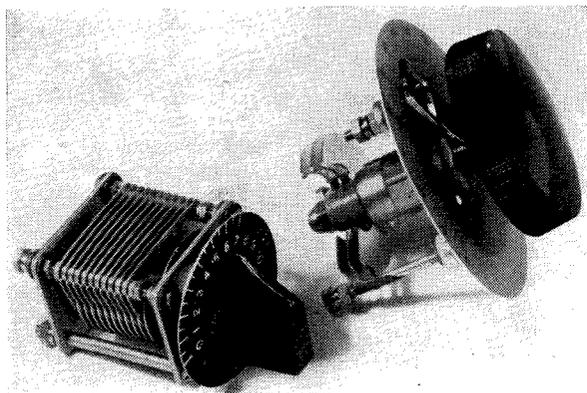
*The new Eddystone condensers for ultra-high frequency work are a good example of stable design. Both rotor and stator plates in addition to all spacers are all constructed of the same material, so having the same coefficient of expansion.*
