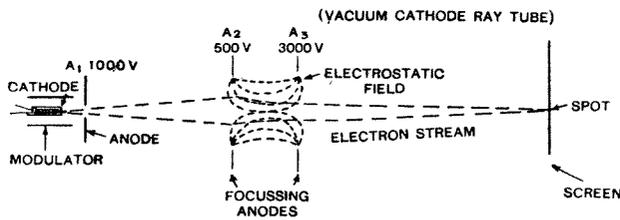
Fig. 3.—Electrostatic focusing of the cathode-ray beam.
