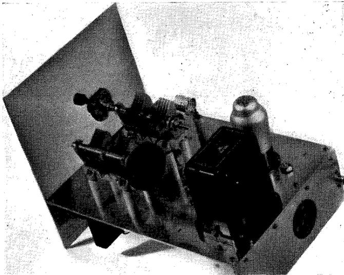
The large double-gang condenser in this illustration is for band setting.
