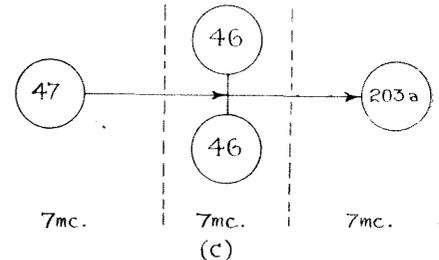
Fig. 4c.—This is the final valve line-up when used on the lower frequencies.
