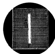
*Frame scan disconnected. Faulty valves or disconnection in scan unit.*
