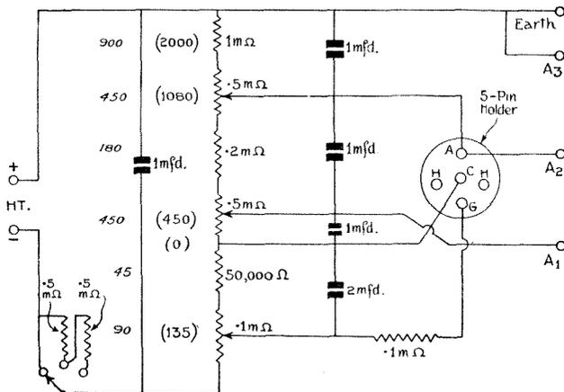
Fig. 1.—Circuit diagram of resistance chain.
