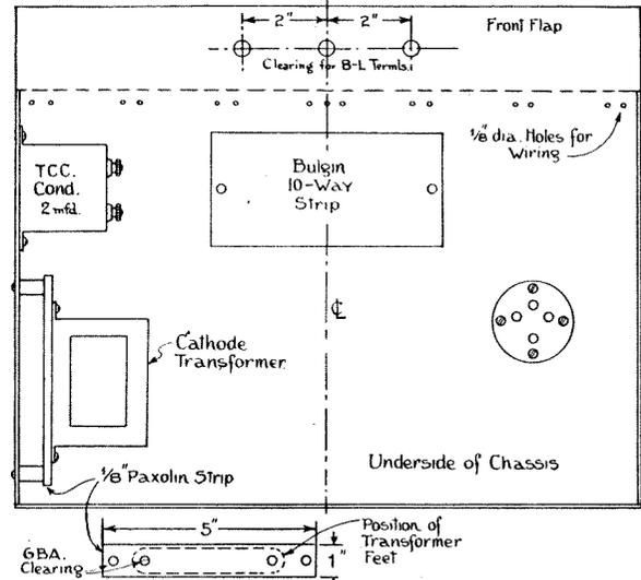
Fig. 3.—Diagrams of upper and under sides of base showing positions of components.
