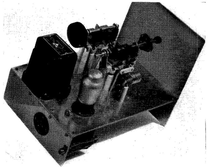
Notice how the detector valve, grid condenser and tuning coil are all closely linked together.
