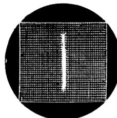
*Line scan disconnected. Faulty valves or disconnection in scan unit.*
