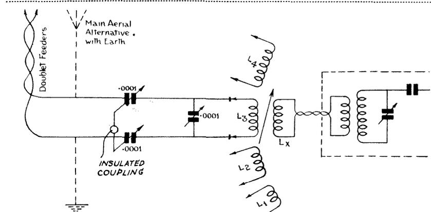
*Fig. 2.—This theoretical circuit illustrates how the coupler can be used with almost any receiver.*
