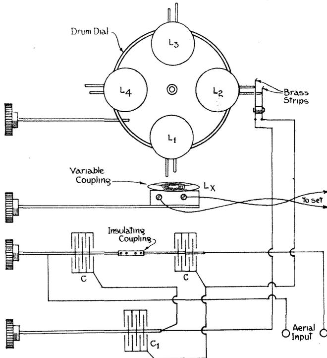
*Fig. 1.—There is nothing in this unit that cannot be made by the average constructor. A small improvement can be made by enclosing the components in a metal container so as to prevent any stray pick-up. All coils are of the flat pancake type which have proved to be most satisfactory despite their old design.*
