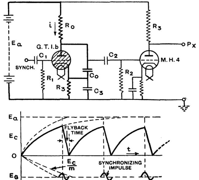
Fig. 5.—Time base circuit using gas-filled relay and (below) the saw-toothed wave form produced.
