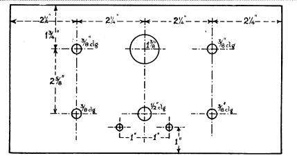
Fig. 4.-The box is drilled with several holes, the exact dimensions being as above.
