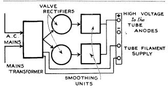
Fig. 5.—Units supplying high and low tension to the cathode-ray tube.
