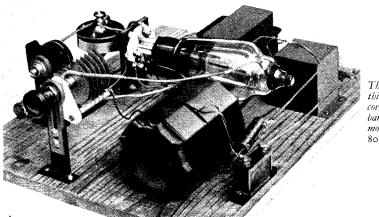
The coil shown in illustration this covers the 160 metre band, but it can be modified for use on 80. 40 or 20 metres.
