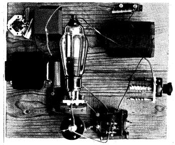
condenser. Even beginners know that since the introduction of the pentode and screen-grid valves, there has not been the need for neutralising in radio receivers. This generally applies to transmitting apparatus, but in this particular case, unless there is slight feed-back from anode to grid, the circuit will refuse to oscillate, owing to the complete screening offered by the third grid.
