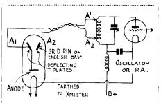
This miniature cathode-ray tube can be connected very simply to a C.W. transmitter, and, as explained in the text, has numerous uses.
