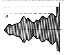
Fig. 3.—The method of distinguishing between signal and synchronising pulse used in the French system.
