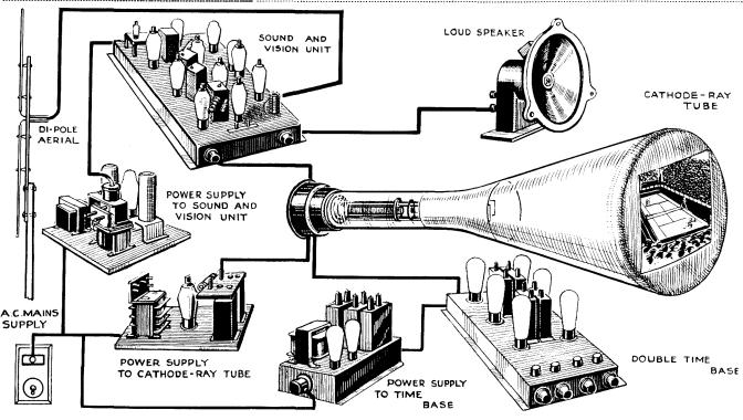
Fig. 7.—The complete arrangement of a cathode-ray receiver shown schematically.
