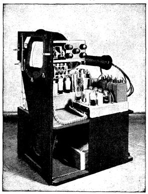
The chassis of the G.E.C. television receiver showing the sound and vision receiver beneath the cathode-ray tube.
