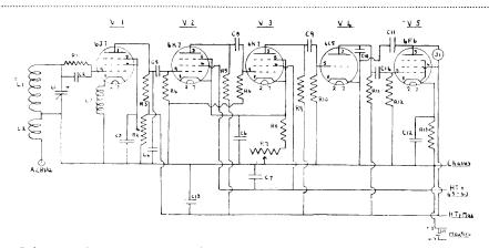
Only one tuned circuit is necessary in this receiver owing to the use of ingenious detector-oscillator circuit whereby regeneration is obtained through cathode coil L3—actually an R.F. choke.
