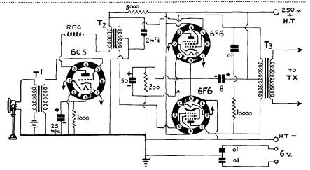
The modulator is very similar to the transmitter, consisting of a triode amplifier and two pentodes in Class A push-pull. Approximately 8 watts output can be obtained.
