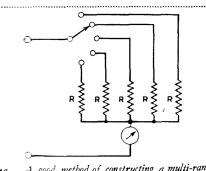
4a. .- A good method of constructing a multi-range voltmeter. ......
