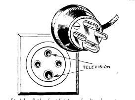
Special wall plug for television and radio relay systems.
