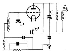
Fig. 7. A grid neutralised circuit of this kind is very effective, while the tuned circuit permits of easy coupling to the previous stage.
