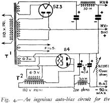
Fig. 4.—An ingenious auto-bias circuit for the transmitter.
