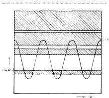
Fig. 1.—Possible energies (indicated by batching) for an electron moving in a simple periodic field.
