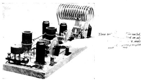
construction. To this end the equipment was built bread-board fashion with the minimum of loose connections an<sup>3</sup> wired with 12-gauge copper wire.
