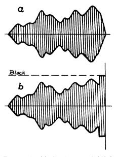
Fig. 1a.—A modulated carrier wave in which black corresponds to full amplitude. Fig. 1b.—The same carrier with the addition of a synchronising pulse at the end of the line.
