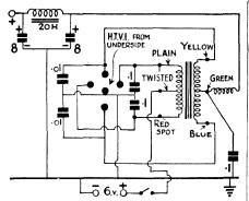
Two of these units are needed to drive the complete transmitter; one for the modulator and one for the oscillators.
