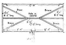
Fig. 6.—Rotary beam aerials only become practicable on 10 metres and under. Full dimensions of this aerial are given in this illustration.
