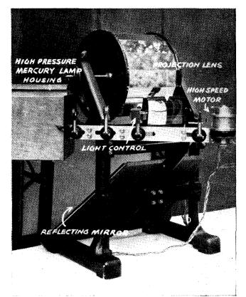
Rear view of the Scophony receiver showing the optical arrangements and light control.
