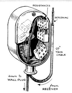
A junction box is provided in each flat which contains the connectors and resistances for television and radio relay.
