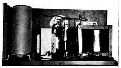
The mains transformer and special electrolytic condenser can be seen in this illustration.
