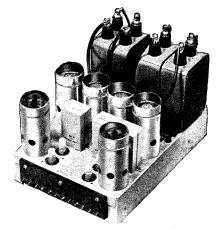
The G.E.C. double time base showing values, condensers and neon limiters.
