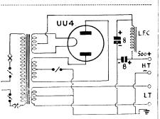
A power pack of this kind is required for the transmitter. It gives a maximum of 500 volts at 120 Mla.
