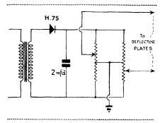
Fig. 1.—H.T. supply to picture shift circuit employing a metal rectifier
