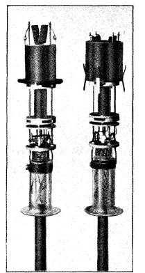
Fig. 1 Electrode structure of SAFAR tube, 1934 type.
