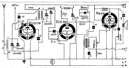
The numbers on the coils agree with the numbers that can be found on the base of the Eddystone coil holders. These should be strictly followed.
