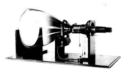
"CATHOVISOR " CATHODE RAY TUBE Type 15 MWI Complete with Electromagnetic Scanning and Focusing Equipment.
