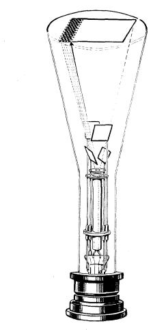
Fig. 2.—Diagram showing the scanning motion of the cathode beam.
