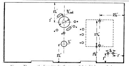
Fig. 2.—These are the dimensions for the screen which is fitted across the box.
