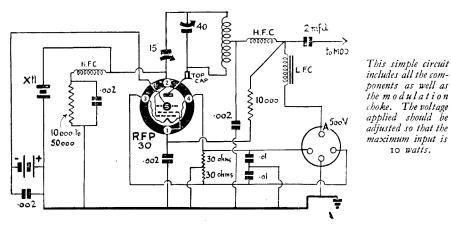
with heavy wire of at least 18 gauge, the coil will be fixed by the wiring so there is no need to mount it off the baseboard on stand-off insulators. While on the topic of coils, for 160 metres approximately 85 turns are required wound solenoid without gap on a 2 ins. former. The coil is centre tapped as shown in the theoretical circuit and is taken indirectly to high-tension positive.
