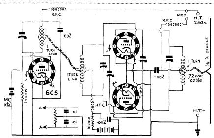
Here is the complete circuit for the transmitter. It consists of a triode crystal oscillator link coupled to two neutralised triodes in push-pull.
