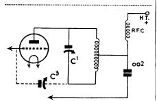
Fig. 1. Simplest radio frequency amplifier using a neutralised triode valve.
