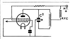
Fig. 3. Greater radio frequency output for a given input can be obtained from a pentode valve in this type of circuit.
