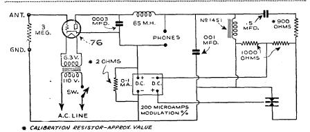
Fig. 5.-Instead of guessing at percentage modulation, use this type of meter which gives accurate direct readings.
