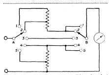
5. The switching arrangements in Figs. 3b and 4b can be used to form a combined voltmeter and milliammeter in shis way.
