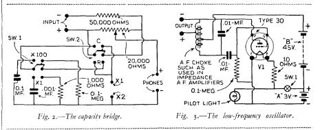
from the Belgian publication, Conseil-Radio. It shows a circuit for a capacity bridge and a low-frequency oscillator circuit. Fig. 2, showing the capacity bridge, can be simply built and is very flexible. It has two toggle switches; one for switching over from low-value resistances or condensers to components of higher values, and the other for changing the circuit from a capacity bridge to a resistance measurer.
