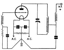
Fig. 6. To obtain smooth operation take all earth returns to a common point as shown.
