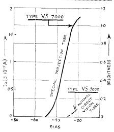
Fig. 3. Characteristics of projection tube.
