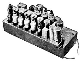
The sound and vision chass of the G.E.C. receiver showing aerial connection at the front and single tuning adjustment in the right foreground.
