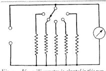
Fig. 2. If a milliammeter is shunted in this way it can cause considerable error.
