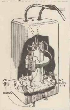
The tuning circuit with its associated condensers and resistors are mounted in a can as shown in this illustration.
