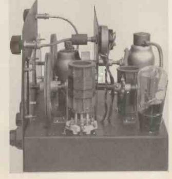
A good idea as to the general construction is obtainable from this view, which shows the aerial coil and output pentode valve.
