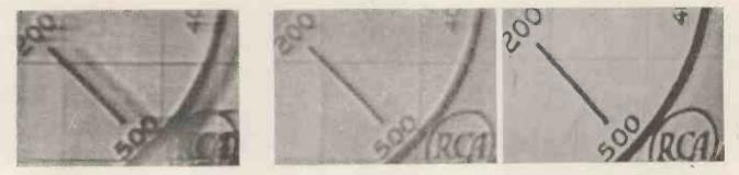
Figs. 2, 3 and 4. Section of the cathode-ray tube screen to illustrate the effect of various receiving aerials on reproduction. The receiver was operated with reduced contrast for best photographic results.
