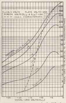
Furthermore, an | The transconductance curves for the 6L7 valve
