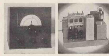
This illustration gives a very good idea as to the construction of the R.M.E. frequency expander. It is similar in appearance to the DB-20 but includes four valves.
