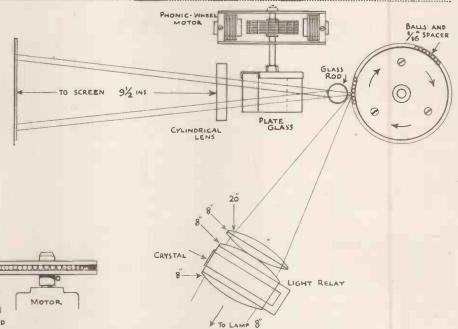
Figs. 5 and 6. These two drawings show a plan and elevation of the simple scanning system. The scanner is of a novel type employing steel balls and an entirely new device for framing and interlacing. All the parts used are of a very simple character and are available.
