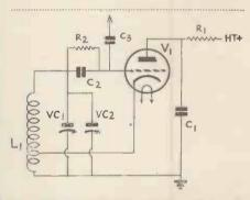
This is the circuit for the complete B.F.O. unit which can be mounted in a metal container or on a breadboard if it is more convenient.
