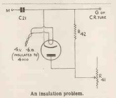
possibility that the measure of insulation you have provided for the tube heater and cathode leads is inadequate. Ensure that the leads are kept well clear of the chassis and provide large clearance holes where they pass through.
