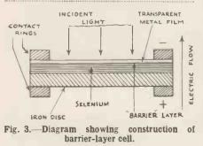
This layer is coated on its outer surface with an extremely thin transparent metal deposit. Incident light passes through this metal deposit and creates a potential difference at the boundary-plane between the
