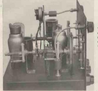
This is the opposite end of the receiver showing the flexible coupler going to VC6 which tunes to wave trap circuit.
