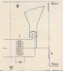
The voltage existing across  $\times$  is 4,000. With the 6-way plug withdrawn this circuit is removed.
