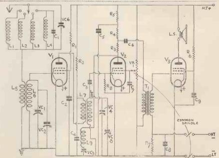
How the wave trap circuit is embodied can be seen from this theoretical circuit. L.F bias is obtained automatically.
