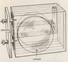
Fig. 7 (above) The supersonic light modulating cell merely consists of a glass sided box capable of holding a liquid with a crystal at one end to which the input from the receiver is applied. The owners of the patent for this type of cell are Scophony Ltd. and it is only permissible to use it experimentally.
