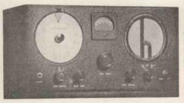
The Sky Buddy Receiver although only using five valves has a performance equivalent to a nine stage receiver.
