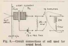
it can be assumed that the maximum output is obtainable if the external resistance is equal to two-thirds of the internal resistance. This is of importance when designing lightoperated relay devices.
