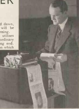
$8\frac{1}{2}$  in. The length of each page is cabinet. Two designs of facsimile receiver-printers have been developed. One is fairly elaborate and automatically cuts the paper into 12-in, pages and deposits them neatly in a tray. The other is much simpler, and does not cut the paper into strips.
