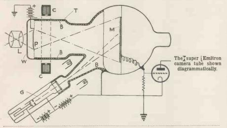
sheet of mica backed by a metal signal plate. The optical image is focused by a lens L on to a conducting transparent photo cathode P, which is supported on a thin sheet of transparent material (e.g., glass or mica) situated close to a polished glass window W.
