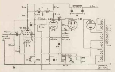
A typical amplifier embodying volume expansion, using a Heptode, triode, double diode and rectifier.
