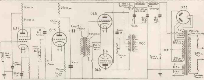
Only five valves are used in the complete circuit which includes the rectifier. Notice that the input valve is a pentode with triode connections.
