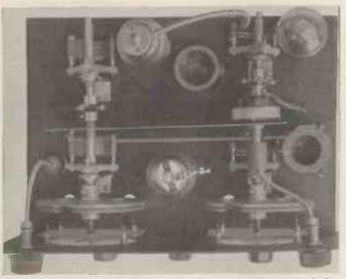
This plan view shows the lay-out of the components, particularly how the flexible couplers are used.
