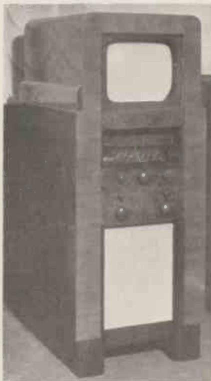
The Ferranti model T.4. Giving a picture size 10 in. by 8 in. this receiver also incorporates an all-wave broadcast set.
