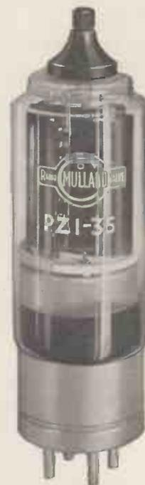
This Mullard pentode the PZ1-35 with 1-watt of excitation will provide a carrier power of 10-watts at 15 metres.
