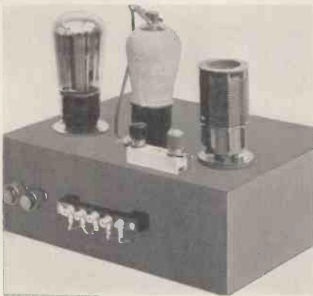
Notice now that four out of the five terminals are in use. If headphones are used they should be isolated from the final valve by a 1/1 ratio output transformer.
