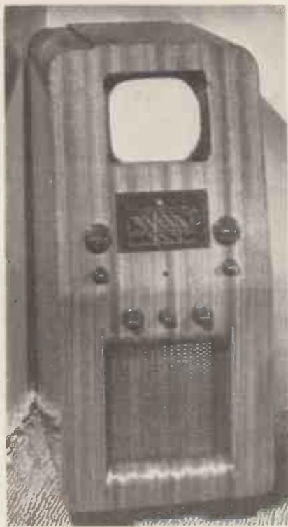
With this model by Marconiphone the picture size is 6 in. by 7½ in. A 5-valve radio receiver is also incorporated.
