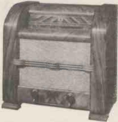
A fine 8-valve all-wave high quality receiver produced by G.E.C.
