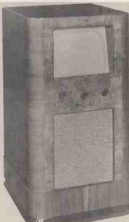
This is the G.E.C. console model providing a picture 10 in. by 8 in.
