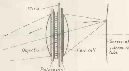
Fig. 3. Schematic diagram of receiver.
