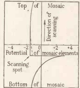
Fig. 5. Diagram showing how the picture signal is derived.
