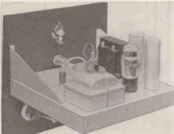
The power unit is quite compact but takes up the majority of the base plate. Notice how the flexible coupler is fitted.
