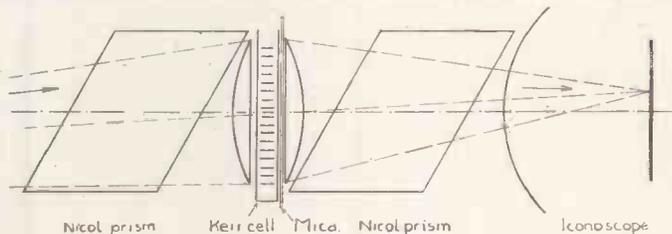
High voltages, however, can be avoided by producing one part of the path-difference by a crystal plate (Fig. 1).
