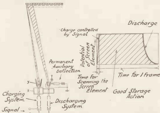
Fig. 6. Storage arrangement with two electron beams and good storage effect.
