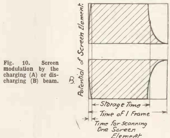
Fig. 10. Screen modulation by the charging (A) or discharging (B) beam.
