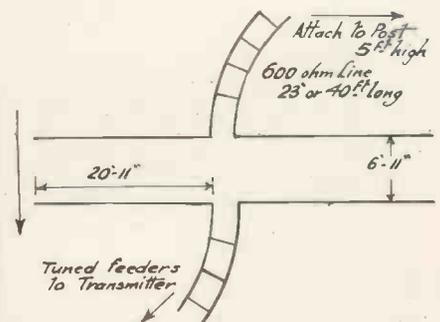
Fig. 3. Parasitic elements with phased half-wave radiators.
