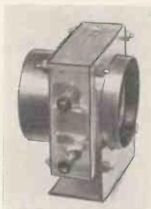
Light relay with crystal, showing angle-brass mount. (Note: In this photo the brass angle is turned the other way from that recommended in the drawings, as this was a first model, and drilled slightly differently.)
