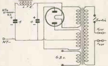
A power pack is optional, but here is the circuit if constructors wish to make the pre-selector self-contained.
