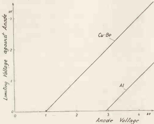
Fig. 3. Charging potential, dependent on anode voltage for various materials.
