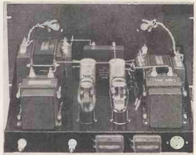
Two power units are needed for the speech amplifier equipment and these are mounted in this manner.
