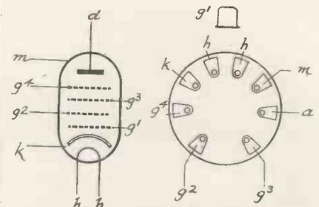
Here are the connections for the EF8 valve
