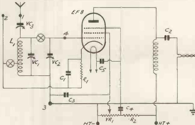
All the coil connections are carried out by the manufacturers so that this portion of the circuit only takes about half-an-hour to complete.
