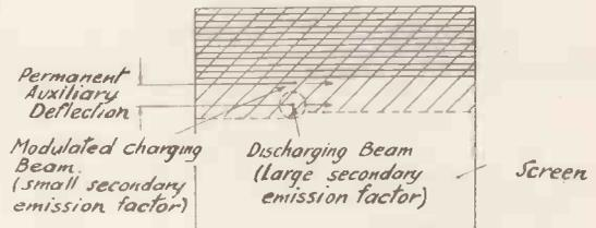
Fig. 7. How the potential distribution is built up.
