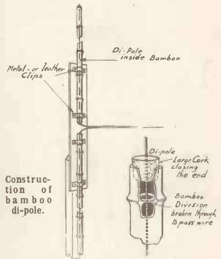
Construction of bamboo di-pole.
