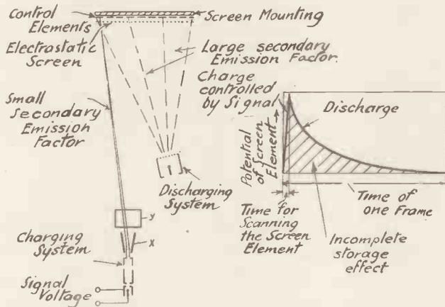
Fig. 5. Simple storage arrangement working with secondary emission.
