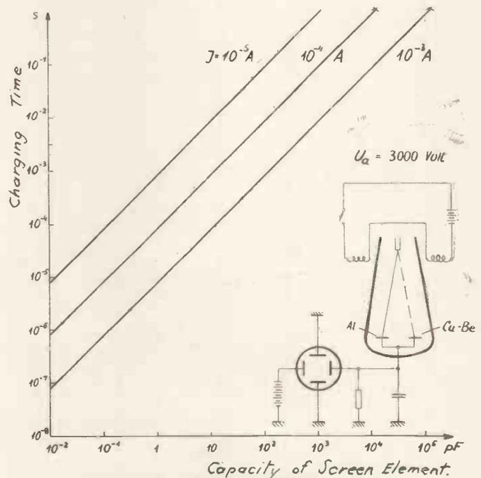
Fig. 4. Charging time for screen elements dependent on their capacity for three different values of beam current and approximately 1,500-volt charge potential. (Charge potential produced by change over from Al to Cu-Be target. Charging time = time in which 63 per cent. of the limiting voltage change is obtained.)
