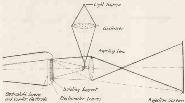
Fig. 11. Projection receiver with "Electrometer" screen.
