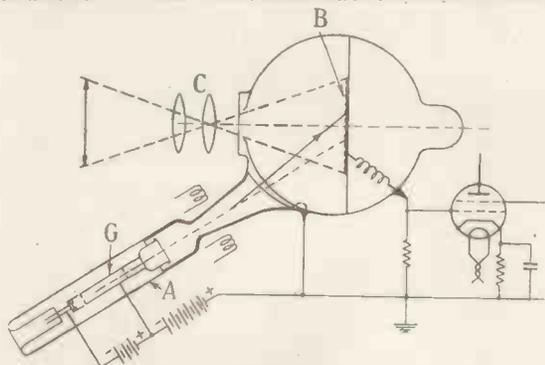
Fig. 1. Schematic diagram showing the constructional and operating principles of the Emitron.
