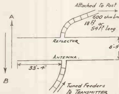
Fig. 2. Two half-waves in phase with parasitic elements.
