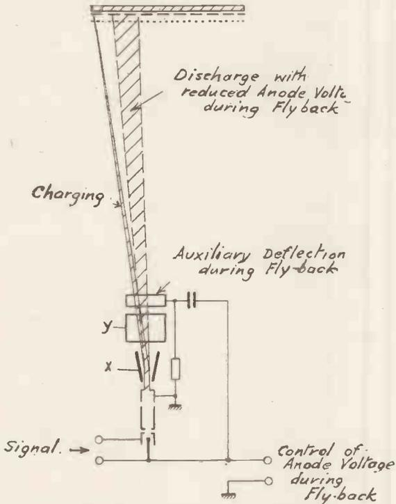
Fig. 8. Storage arrangement with one electron beam.
