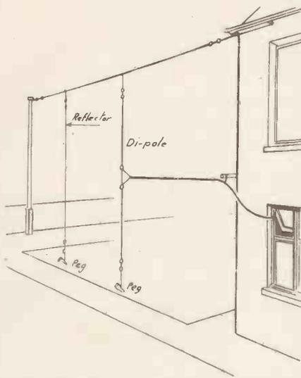
Using the broadcast aerial as a support for the dipole.
