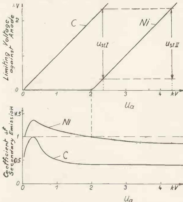
Fig. 1. Production of the control voltage  $U$  on an isolated screen element :
