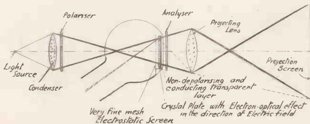
Fig. 12. Projection receiver with electron-controlled screen.
