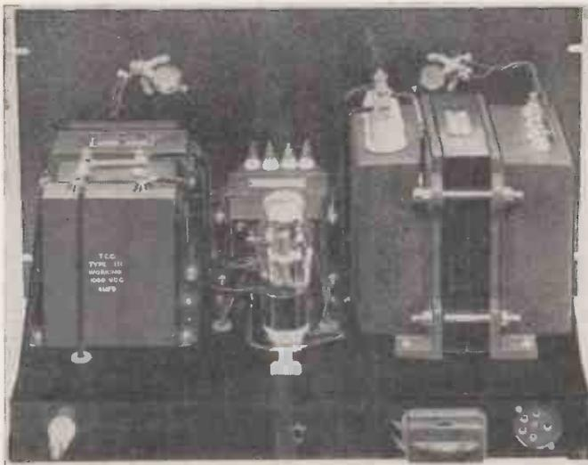
This is the large power unit for the R.F. portion of the transmitter. It provides between 700 and 750 volts at 250 m/A.
