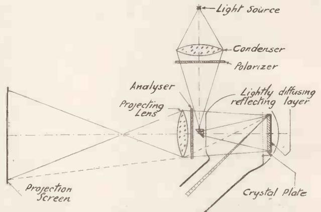
Fig. 13. Storage projection receiver in which the electron optical effect is doubled.
