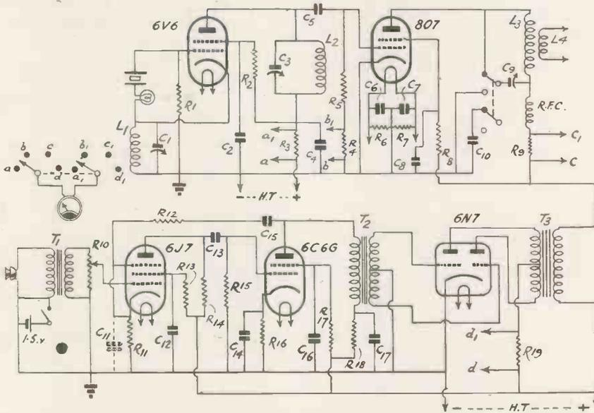
Fig. 1. A most effective low power U.H.F. transmitter suitable for C.W. of telephony.
