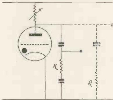
Fig. 4. Inclusion of a resistance R increases the fly-back speed. An alternative arrangement often employed is shown by the dotted connections.
