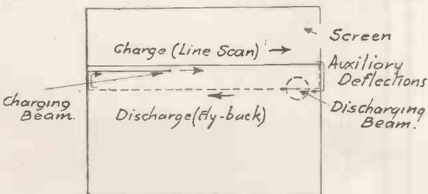
Fig. 9. Shape and movement of the electron spot on the screen of the arrangement according to Fig. 8.
