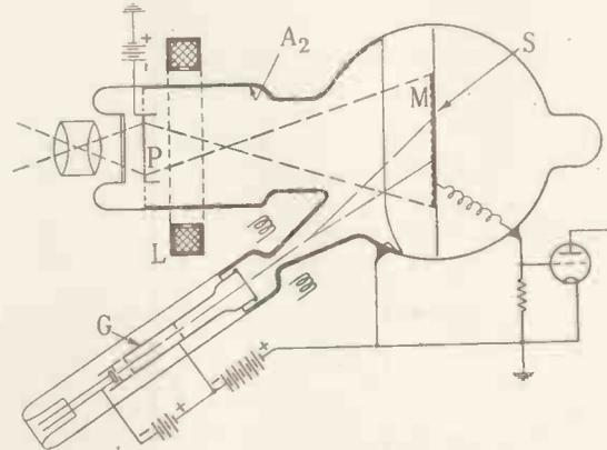
Fig. 6. Schematic diagram of the Super-Emitron.
