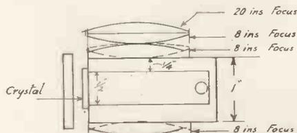
Constructional details of light relay cell.
