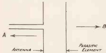
Fig. 1. Parasitic elements with phased radiators co-linear.
