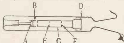
Fig. 2. Diagram of electron gun arrangements.
