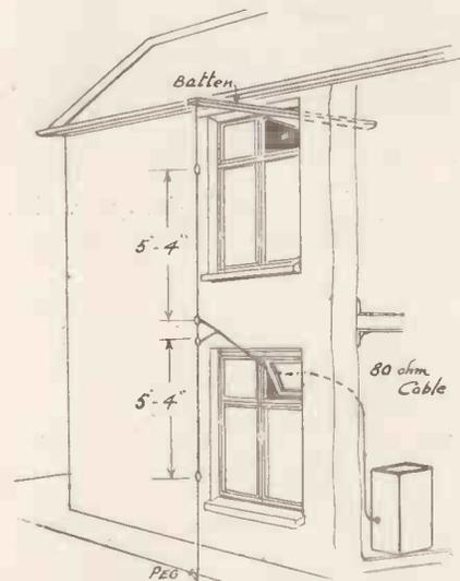
A simple di-pole consisting of two tensioned wires.
