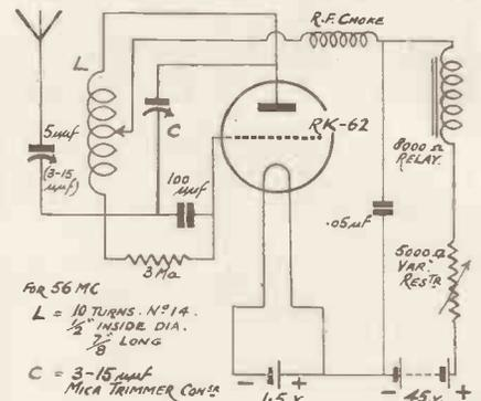
This is the remote control circuit using a new gas triode type RK-62.
