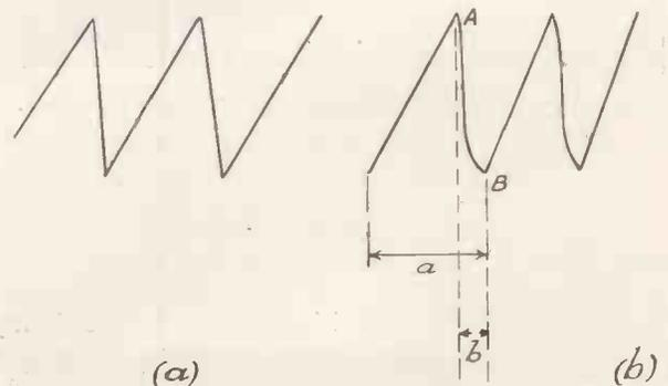
Fig. 3. In (a) above is shown the required wave shape. In (b) the fly-back tends to slow down when nearing completion, but providing (b) is equal to or less than 10 per cent. of (a) no harmful result obtains.
