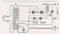
A metal rectifier is used in the power unit and here is the circuit.
