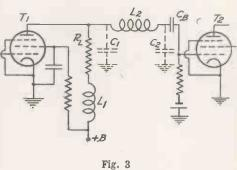
$0.034/f_0$ , i.e., 3.4 per cent. of the period  $T_0$  at the top frequency,  $f_0$ . With  $f_0=3$  Mc,  $\Delta_T$  is 0.011 microseconds. This is the difference in seconds. time delay caused by the presence of shunt capacitance in the plate-load circuit.
