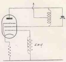
Fig. 4.--Hartley resonant circuit.
