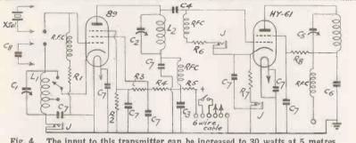
Fig. 4. The input to this transmitter can be increased to 30 watts at 5 metres.
