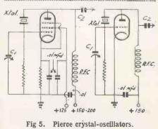
quency-multiplier is a popular arrangement for frequency multiplying. Although the tank circuit values are given for 10- and 5-metre operation, the circuit can be adapted for any crystal frequency by choosing the correct tank constants. It is the usual practice in amateur applications to provide a switching arrangement so that the buffer stage can be coupled either to the output of the crystal oscillator for working at the crystal frequency, or to
