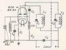
Fig. 8: Double-triode, oscillator-doubler for 5-metre output.
