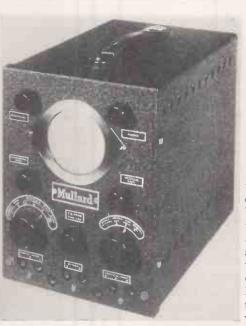
The Mullard type G.M. 3155 portable cathoderay oscillograph employing a three-inch highvacuum tube.
