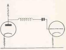
Fig. 8.-Series correcting inductance.
