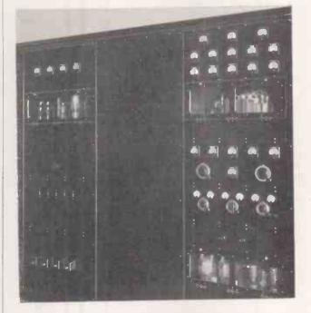
This is the trans-mitter at W9XUP which is now operating on 26.150 Kc. and relaying the N.B.C. red network programmes. The power input to the final is 1,000 watts.
