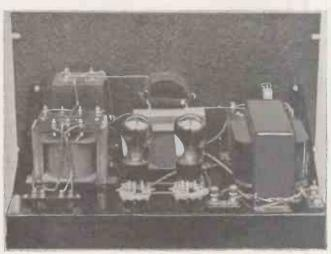
The power unit uses two GU1's and provides 1,000 volts D.C. For lower inputs a 500-volt transformer would be satisfactory with a type 83 full-wave rectifying valve.
