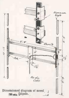
In order to preserve the aerial from the effects of the weather, both the wood and metal parts were given a couple of coats of good varnish after attachment of the lead-in; this in fact will be essential if an aerial of this type is used near the coast, otherwise, the aluminium will corrode and soon fracture.
