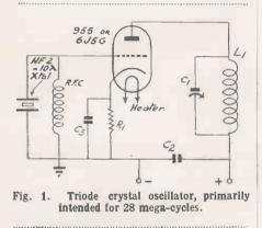
into the circuit in such a manner that the crystal becomes a frequency determining element. The conventional triode or pentode crystal oscillator is merely the well-known tuned-anode tuned-grid circuit with a quartz crystal substituted for the grid tank. For purposes of discussion, such circuits are sometimes called tuned-anode crystalgrid oscillators.
