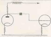
Fig. 7.-Conventional correcting inductance.
