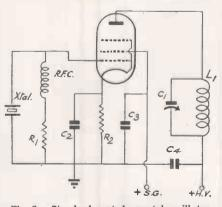
Fig. 2. . Standard pentode crystal oscillator.
