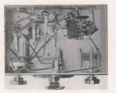
Most of the small components are connected under the chassis as shown in this illustration. Notice the midget inter-valve transformer.
