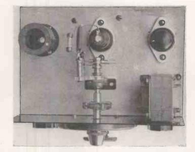
The grid condenser and leak are connected between the grid of the 6J7 and the band-spread condenser.
