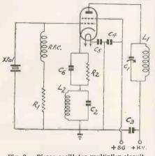
Fig. 6. Pierce oscillator-multiplier circuit.
