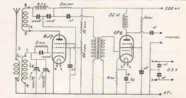
The coils have been numbered in order that constructors will connect them the correct way round in order to obtain maximum gain and reaction.
