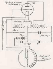
Fig. 1. The Philco remote control arrangement.
