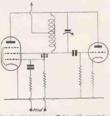
Fig. 5.-Modulated oscillator with sustaining valve.
