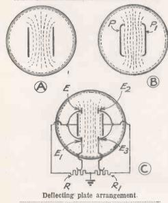
plates of a cathode-ray tube to diverge outwards beyond the edges towards the metallised lining S of the tube, as shown in Fig. A. This " spreading " or curvature of the lines causes the outer parts of each " sweep " of the scanning-stream to have a slightly different focal length from the stream forming the inner or central parts of the sweep, and so gives rise to a lack of definition at the marginal parts of the picture.
