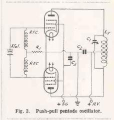
conventional pentode or tetrode oscillators, while a lower ratio is better with triode valves. The greater internal anode-to-grid capacity and the low amplification factor of most triodes, requires that the tank voltages be limited so that the crystal excitation will not become excessive. This applies also to the cathode tank of the tritet circuit, for the oscillating portion is a triode.
