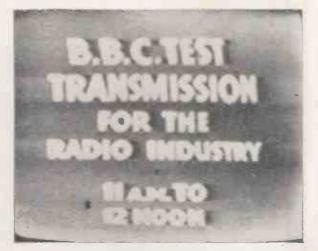
Fig. 6. The uneven background illumination in the above photograph is due to the loss of or inaccurate restoration of the D.C. component.
