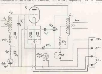
The circuit is a straightforward one but in order to obtain maximum R.F. output the components values should be strictly adhered to. Grid bias is obtained automatically.
