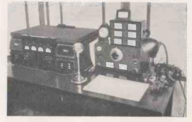
W9DXX has invested in one of the new Hallicrafter HT1 transmitters, which gives 75 watts on telephony and over 100 watts on C.W.
