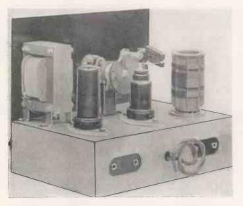
This view of the chassis indicates just how the major components are laid out shows and the sockets for H.T. supply and aerial and earth in addition to the two leads for the heaters.
