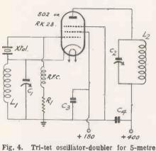
Fig. 4. Tri-tet oscillator-doubler for 5-metre output.
