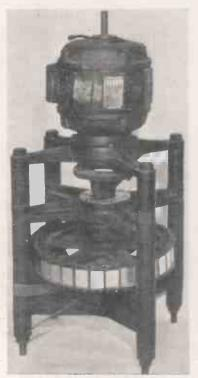
Fig. 1. Mirror-drum scanner (Montrouge 1929)
