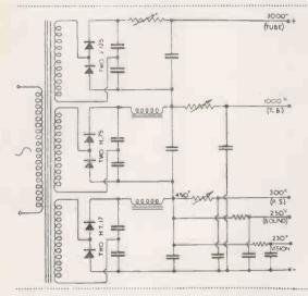
the tube (modulating both shield and first anode) and restores the D.C. component of the picture signal which normally is lost between the output of the video-frequency valve, and the shield of the C.R. tube.
