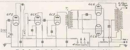
Fig. 5. Over 20 watts of audio are obtainable from this modulator.
