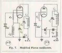
much better than obtainable in the conventional triode oscillator due to the action of the screen-grid. This grid reduces the internal anode-to-grid feedback and also has a compensating action on the valve impedance under conditions of changing power supply voltages. With valves such as the RK23, 802 and 807, which are designed specifically for use at radio frequencies, power outputs of 10 to 15 watts can be obtained at frequencies above 500 kc., with a reasonably low crystal current.
