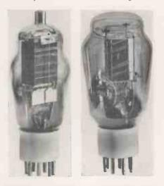
On the left is the Tungsram 0S12/500 a valve similar to the 837. An interesting valve is shown on the right—the Tungsram 015/600 specially made for 5 metre operation.
