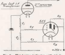
Fig. 2. The tuning indicator with triode detector.
