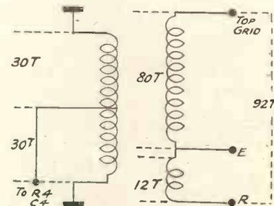
How the coil is wired.
