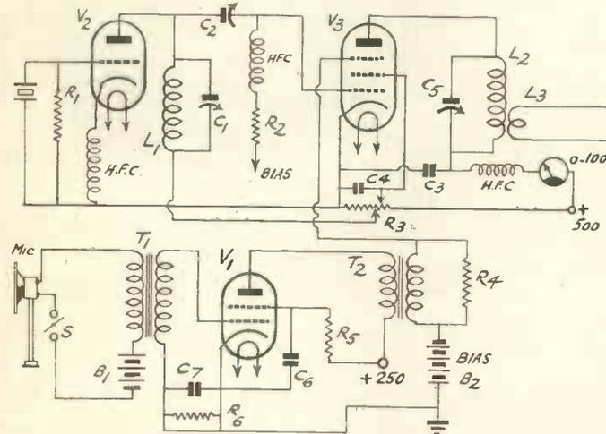
Fig. 4. With this arrangement the transmitter has been designed for telephony use and to run from A.C. mains.
