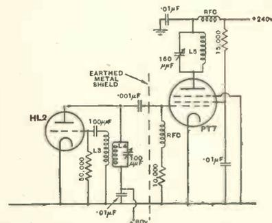
Fig. 2. In this circuit the crystal has been omitted but the scheme is not to be recommended unless a good frequency meter is available.
