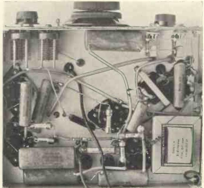
The actual receiver itself is quite small, and in this view can be seen the output pentode, detector and valve voltmeter valve.
