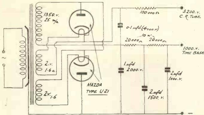
Fig. 6b. Circuit diagram of C.R. tube and time base power supply unit. Two indirectly-heated rectifiers in a voltage doubling circuit are employed; the need for some form of delay switch is thereby avoided.
