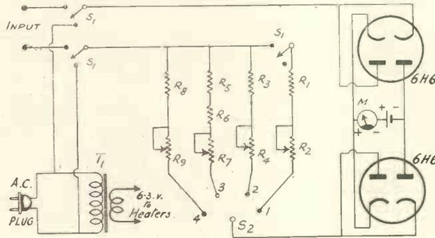
Fig. 1. This meter will read up to 1,000 volts and the resistance values are as follows: R1 5,000 ohms, R2 1,000 ohms, R3 70,000 ohms, R4 15,000 ohms, R5 200,000 ohms, R6 25,000 ohms, R7 50,000 ohms, R8 800,000 ohms, R9 100,000 ohms.
