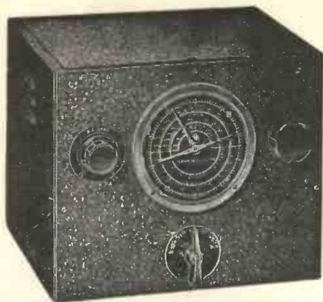
The new Peto-Scott pre-selector uses two of the latest EF8 low-noise R.F. amplifiers. It covers five bands and has its own power unit.
