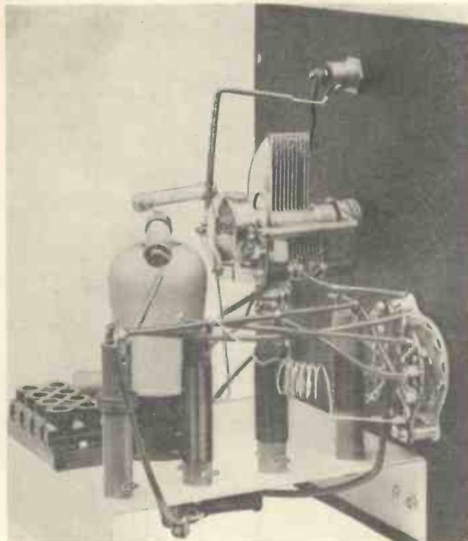
A small chassis has to be used on which to mount the components for the phone monitor and notice that the 10-metre coil is air spaced and mounted in the wiring. The remainder of the coils have a very simple fixing with one 6 B.A. bolt.
