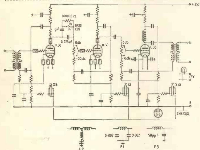
Fig. 5. Circuit of ribbon microphone "A" amplifier.
