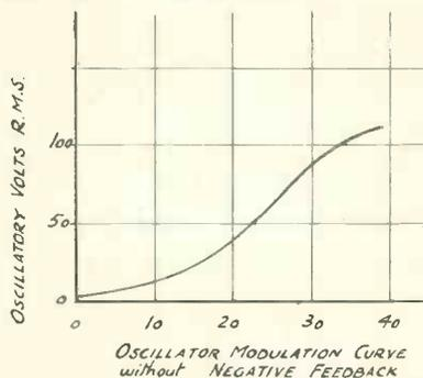
Oscillator modulation curve without negative feedback.
