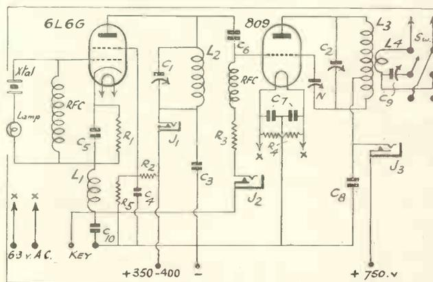
Fig. 2. Up to 60 watts can be obtained from this simple transmitter. Despite the fact that the cathode coil is left in circuit when operating on fundamental frequency, the designer states that crystal current is not high. The transmitter can be arranged for two-band operation without coil changing while the aerial is switchable for series or parallel tuning.
