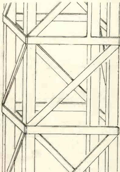
This is how the middle section of the mast is built.
