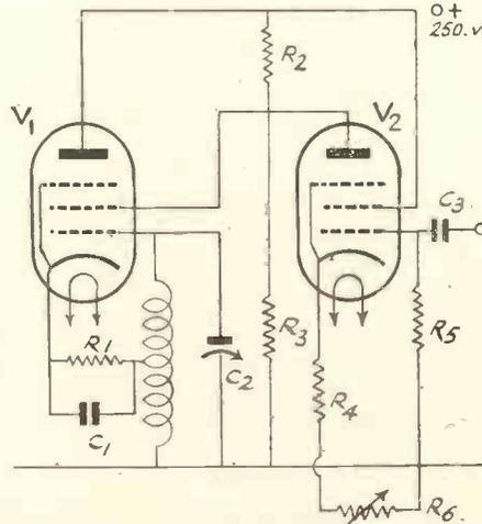
Circuit diagram of modulated oscillator.
