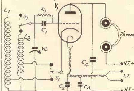
Fig. 1. The single valve C.W. monitor.
