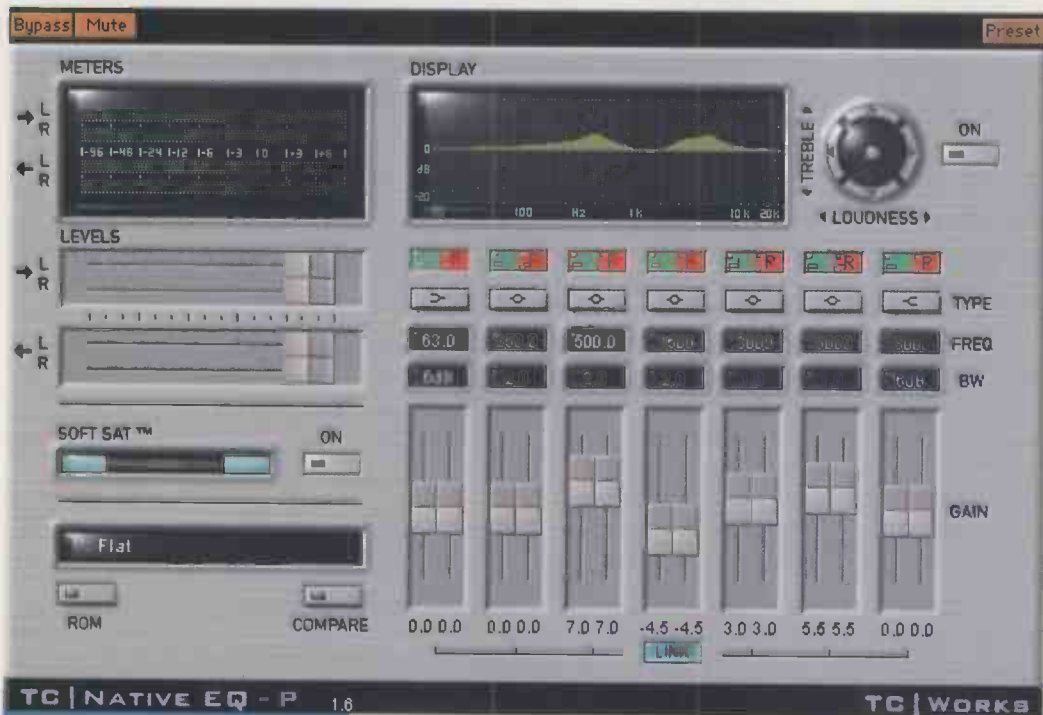
The Parametric EQ includes seven fully-programmable bands, plus a virtual joystick for controlling treble and loudness
