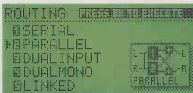
Connect the internal effects engines in (count 'em) six different ways
