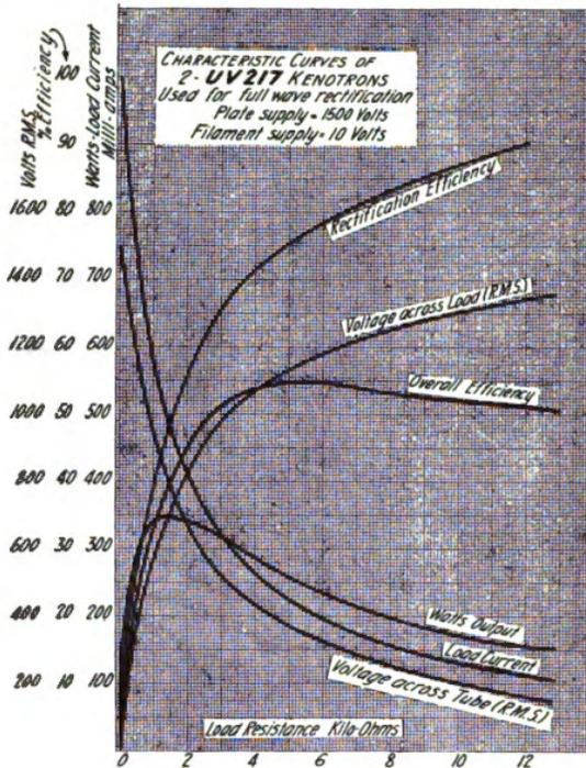
Figure 13—Load characteristics
