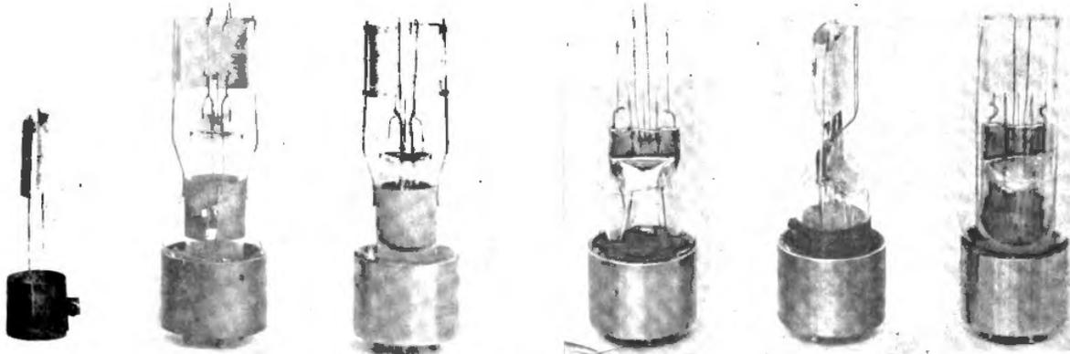
Figure 1—UV-217 Kenotron having a rated D. C. output of 150 watts at 1000 volts. Center view has one-half of plate cut away to show the filament
