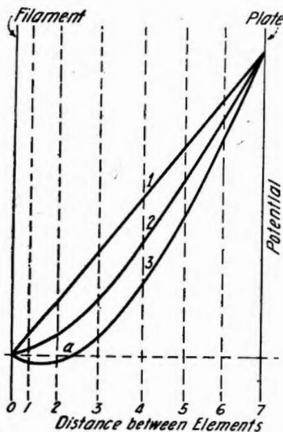
Figure 8—Potential distribution in the Kenotron under various filament temperatures
