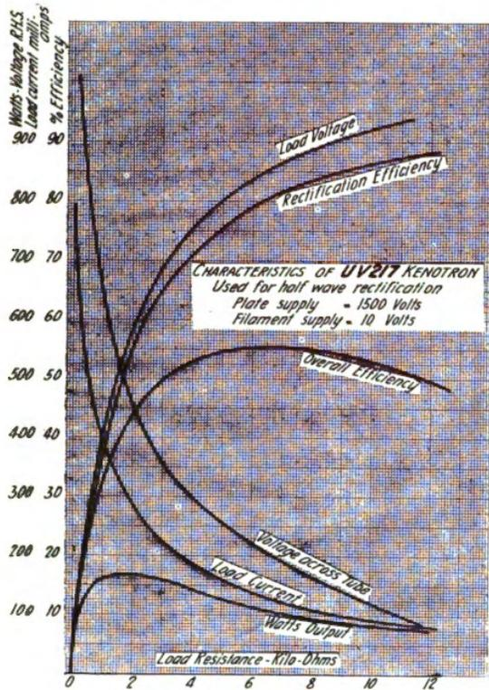
Figure 12—Load characteristics
