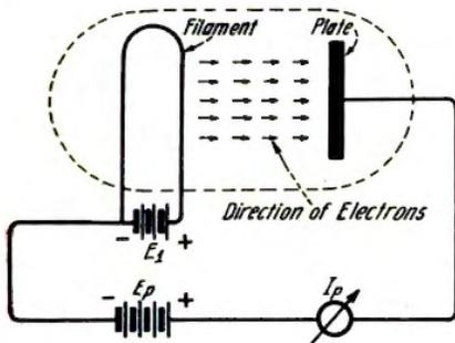
Figure 4—Circuit to determine relation between filament and plate currents
