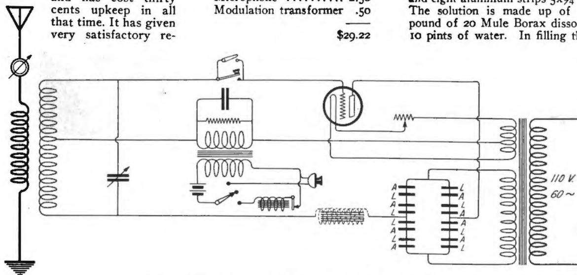
Figure 1—Circuit diagram of the 5-watt vacuum tube transmitter
