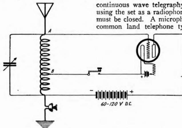
Figure 1—Circuit diagram of a simple CW transmitter
