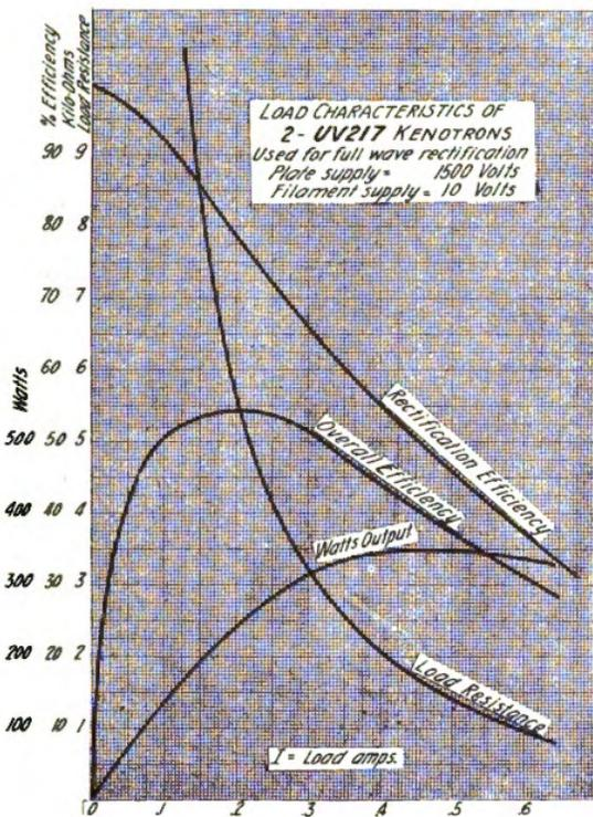
Figure 14—Load characteristics
