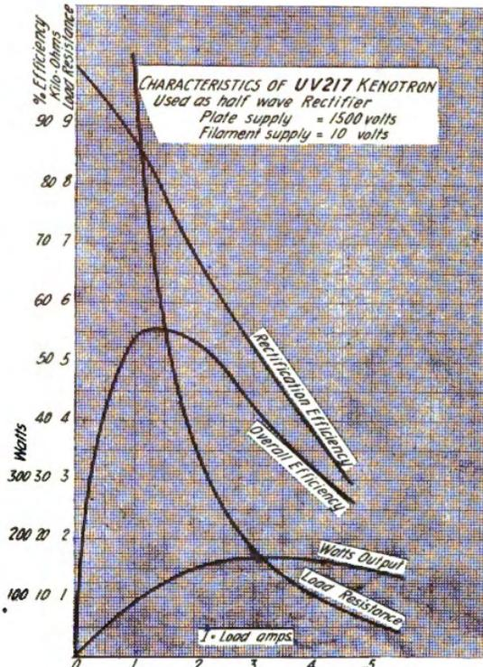
Figure 15—Load characteristics
