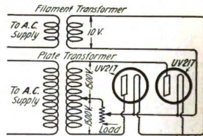
Figure 17—Circuit for full wave rectification
