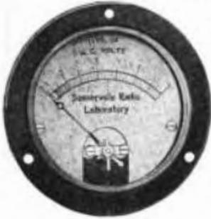
This is a comparatively new meter, brought out to be used in conjunction with the RADIOTRON power tubes. By the use of the proper voltage and current in the filament heating circuit, the life of the tube can be prolonged from two to three times, and the
