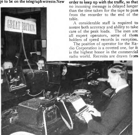
Close-up of transmitting side of English circuit, showing operator at Kleinschmidt perforator. The tape from this passes through the Wheatstone transmitter at the left. One perforator is capable of from 75 to 80 words a minute, and in case greater speed is required, a second operator uses the spare perforator seen at the right
