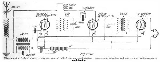
and the coil at the right as the tickler. For the plate coil, one of about 50 or 60 turns is desirable. For the grid coil, one of about 75 turns will do, and another of 40 turns will serve as the tickler.
