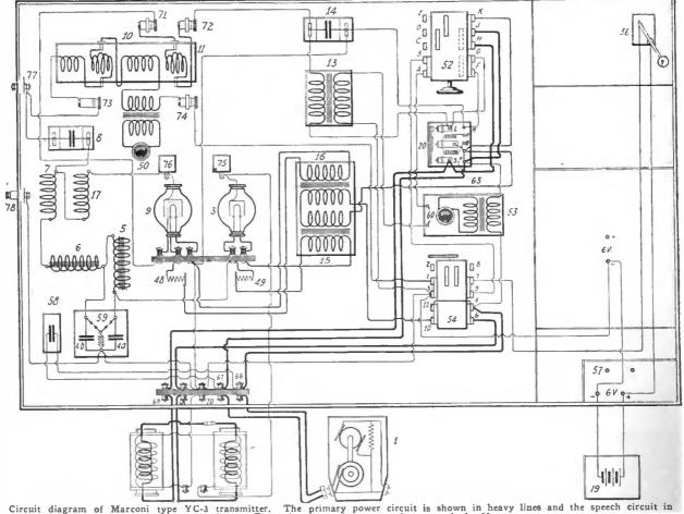
YC-3 transmitter. The primary power circuit is shown in heavy lines and the speech circuit in thin lines. The microphone is connected to terminals 60 Circuit diagram of Marconi type
