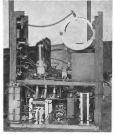
Close-up view of the set showing the three tubes and various other parts
