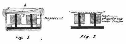
Diagrams of the standard telephone receiver
