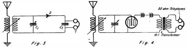
Circuit showing the telephone bridging condenser
