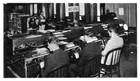
Close-up of the receiving side of one of the English circuits during high speed operation. The undulator signals are written on the tape by the recorder at the extreme right, and are read by the operators. At the time this was taken, 90 words a minute were being received
