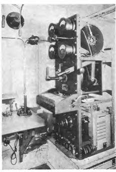
The RCA type SE-1060, 1 K.W. spark transmitter used in regular service
