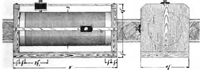
Constructional details of the two-slide tuner
