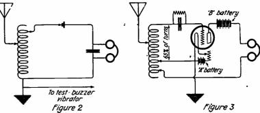
Diagram showing a double-slide tuner crystal set transformed into a regenerative
