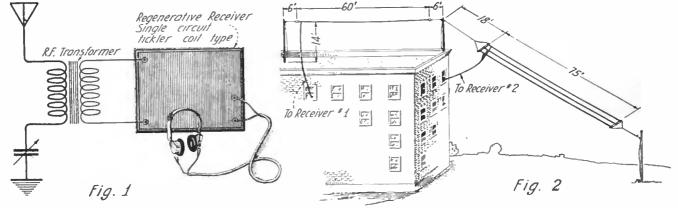
Radio-frequency regenerative set used and antenna conditions during the test
