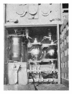
Marconi portable transmitter, type YC-3 using one 500-watt oscillator and one rectifier to supply D.C. to the plate
