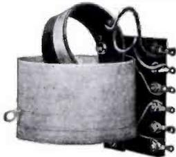
No. 105 Low Loss R. F. Coupler, provided with fixed primary; secondary with neutralizing tap and adjustable rotor. Range with No. 301-A condenser 200 to 500 meters.
