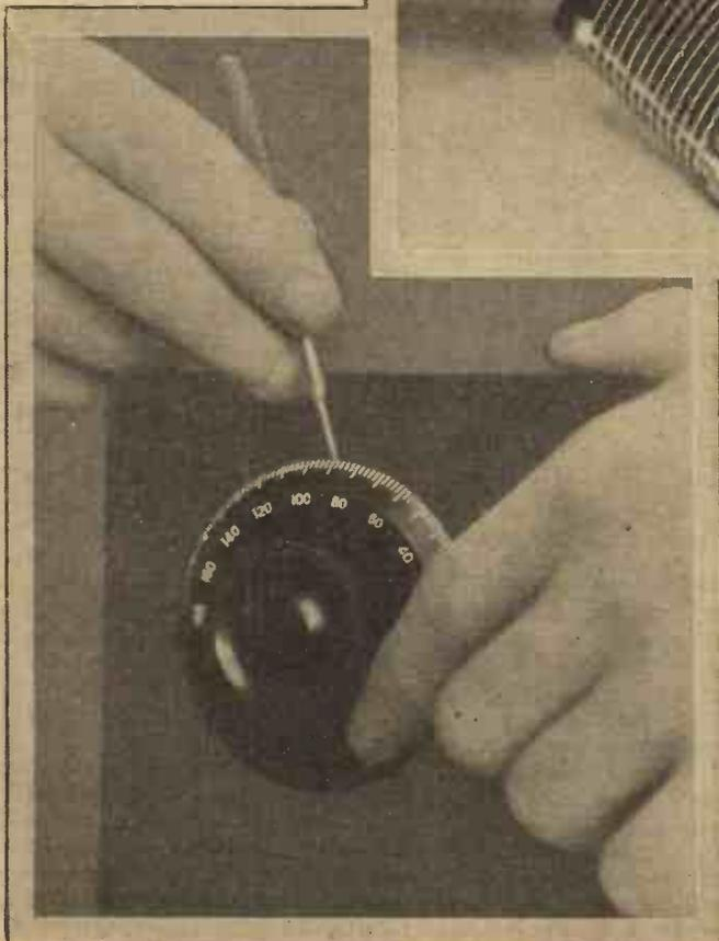
fifth photograph shows how a pipe cleaner may be used as a remedy. This operation should be carried out with considerable care, so as not to bend the plates about, and the cleaner should be passed carefully between each pair of both fixed and moving plates, until it can be seen that both are reasonably clean when held up against a piece of white paper.
